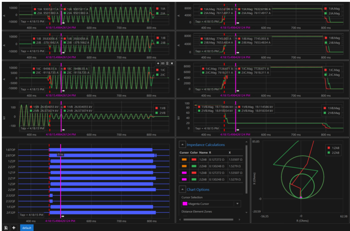
Figure 11. R1 response of the CAPE and PSCAD model for a three-phase close-in fault on bus 10
