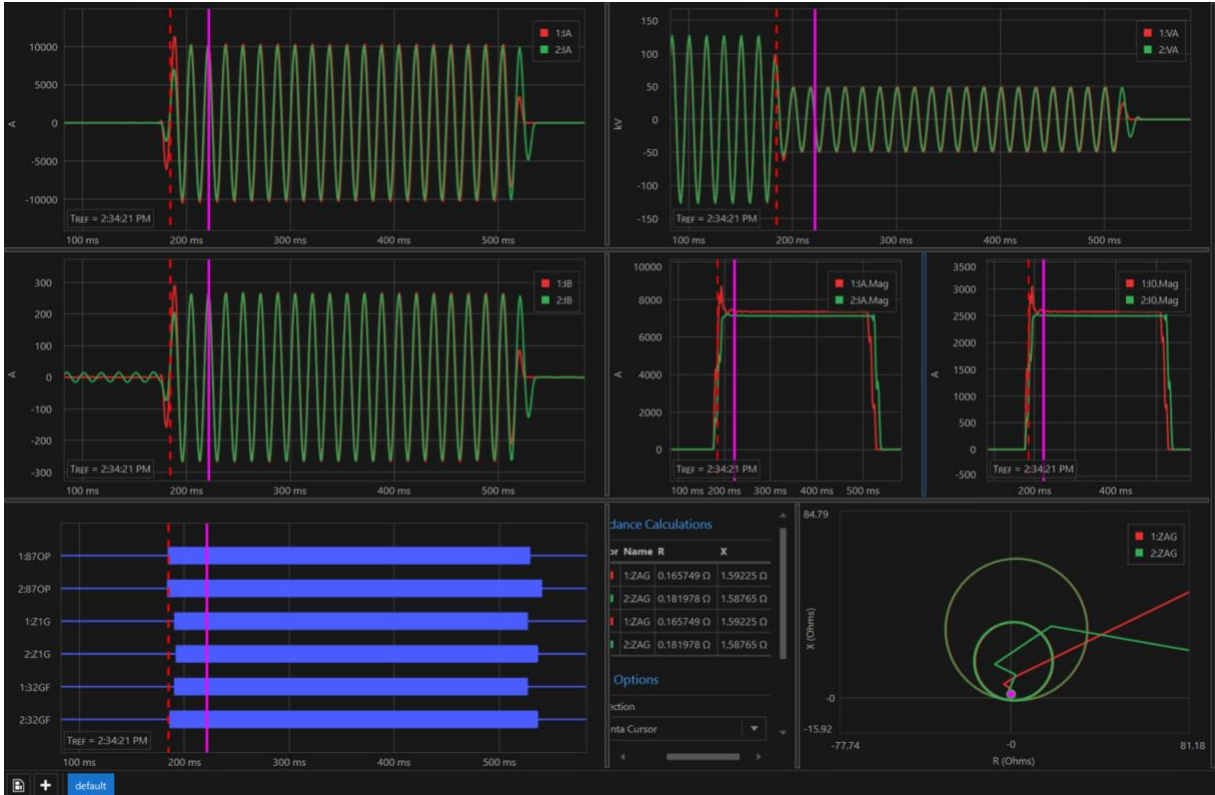
Figure 13. R1 response of the CAPE and PSCAD model for an SLG close-in fault on bus 10
