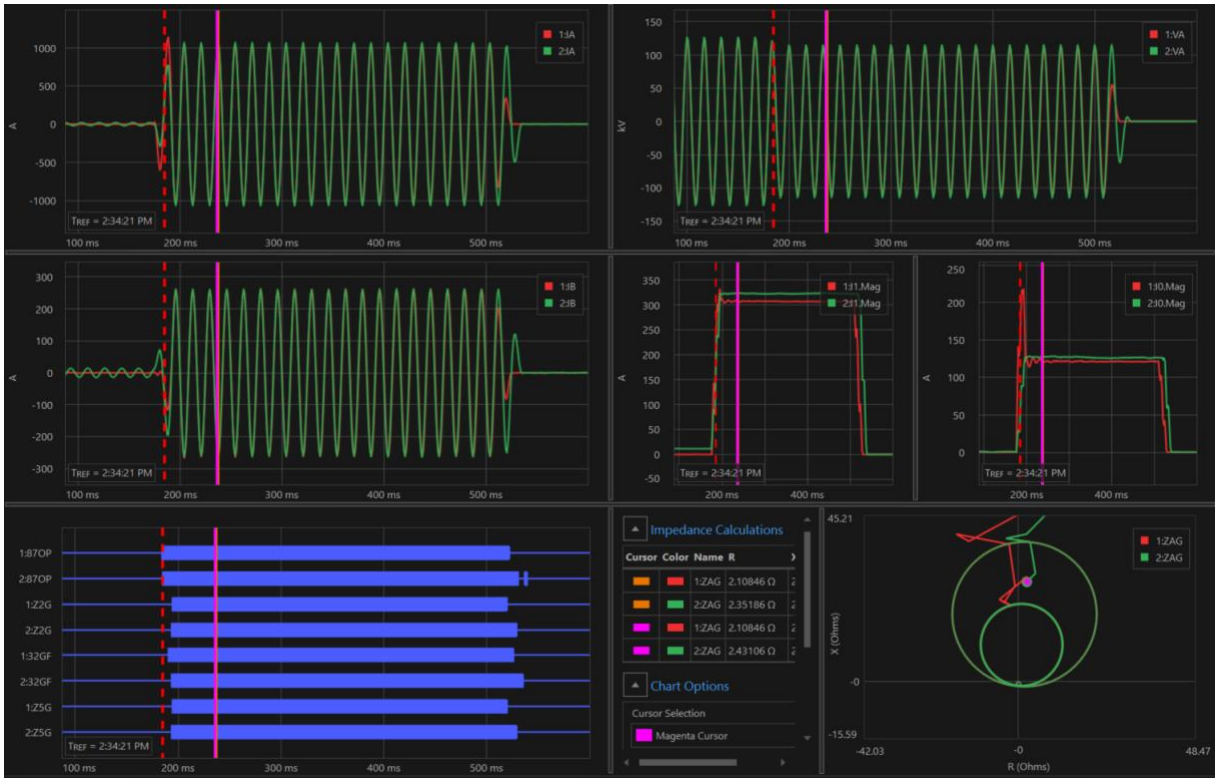
Figure 14. R4 response of the CAPE and PSCAD model for an SLG close-in fault on bus 10
