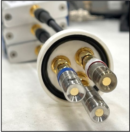
Array of three scCVD sensors in vacuum assembly (left) and gain-matched spectrum (right) of ^{239}\text{Pu} + ^{241}\text{Am} + ^{244}\text{Cm} source (black) [Si in blue]
