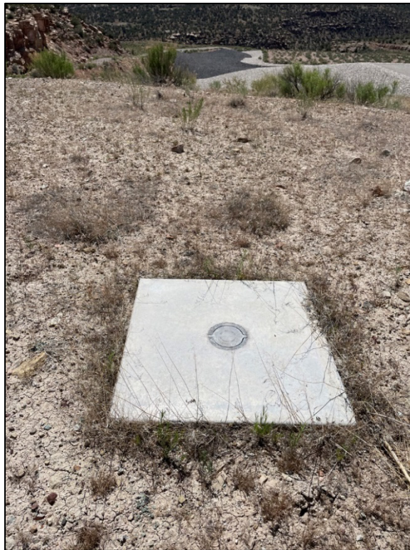
PL-4. Aerial Survey Quality Control Monument QC-3
