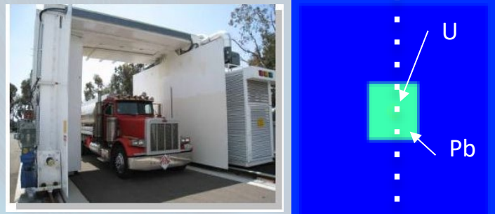
Bremsstrahlung sources- limited resolution CAARS radiography/Z: U sphere in Pb box
