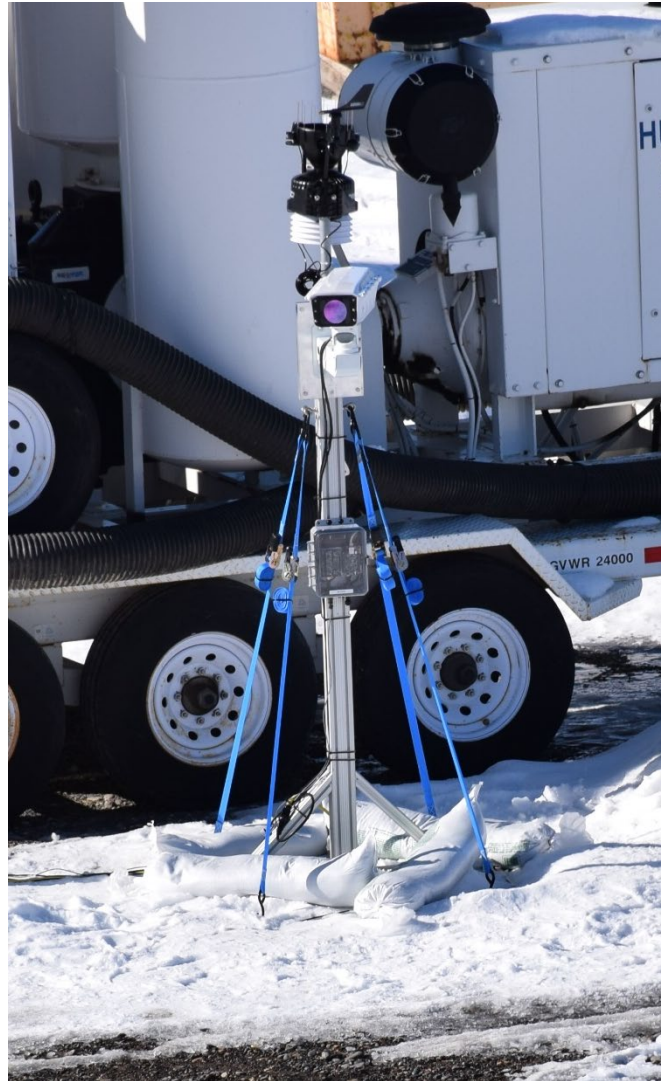
A sensor tree with a weather station, a thermal imager, and a MERYLN
