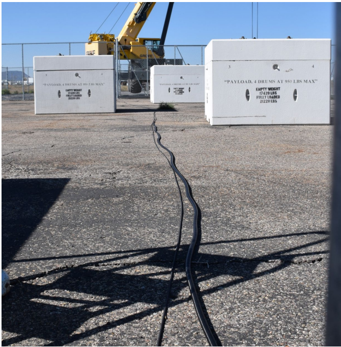
Fig 6. Field testing deployment of the 50-m scintillating fiber and the 20-m optical fiber coupled to 100-m of optical fiber.
