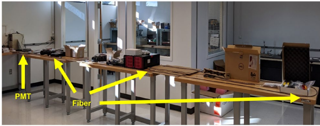
Fig 2. Laboratory bench set-up using a 10-m scintillating fiber.
