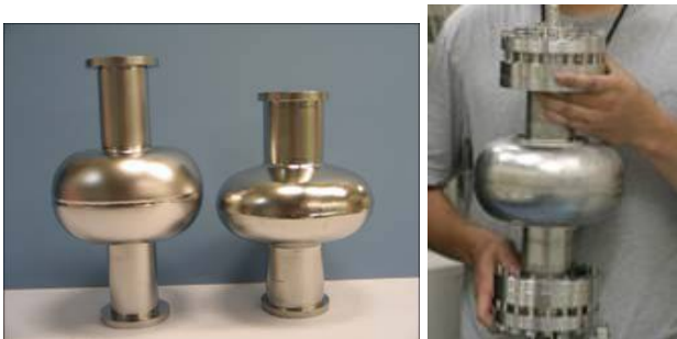
FIG. 8: Single-cell 1.3 GHz elliptical cavities: Cornell re-entrant (left), Tesla (center) and Ichiro (right).
