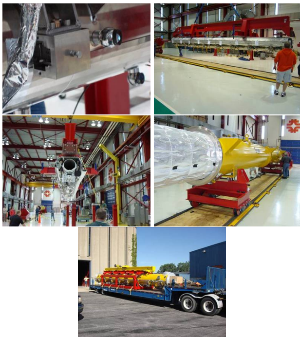
FIG. 19: Recent photographs of the CAF-ICB facility, showing stages in the assembly of the first cryomodule, CM1. [Courtesy of Tug Arkan.]
