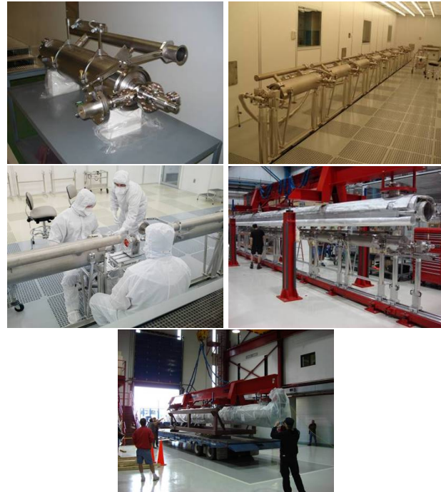
FIG. 18: Recent photographs of the CAF-MP9 facility, showing stages in the assembly of the first cryomodule, CM1. [Courtesy of Tug Arkan.]
