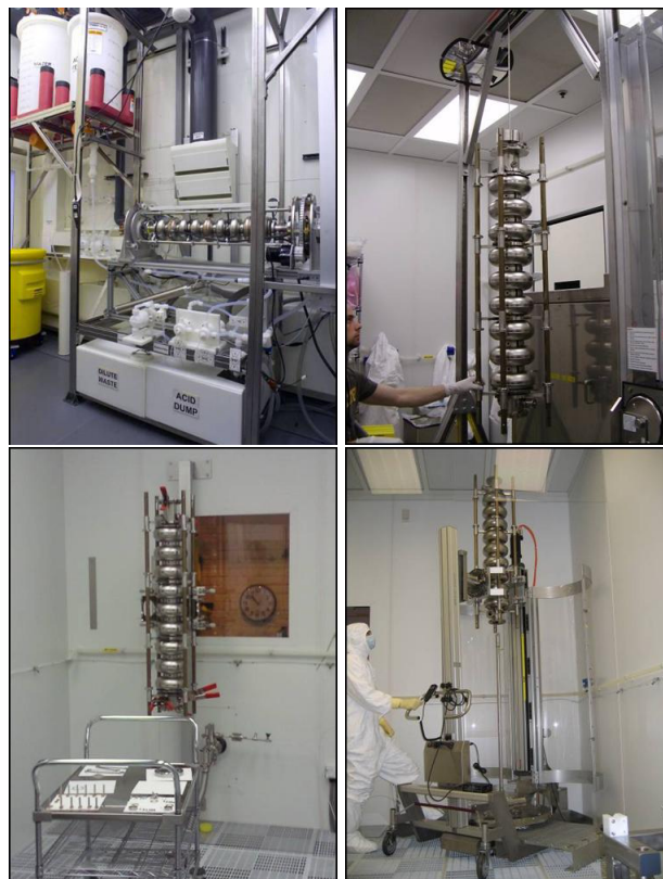
FIG. 14: ANL/FNAL joint facility infrastructure: (clockwise from top left) EP, ultrasonic degreasing, HPR and assembly stands. [Courtesy of Michael Kelly and Damon Bice.]
