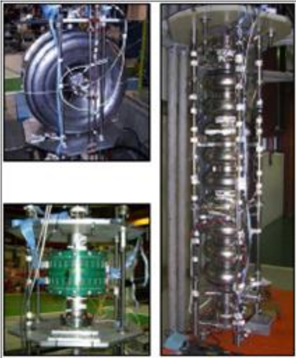
FIG. 15: Some of the cavities recently tested at the Fermilab VCTF: (clockwise from top left) SSR1, 9-cell Tesla-shape, and 1-cell Tesla-shape (with diode thermometry) cavities. [Courtesy of Bill Mumper.]
