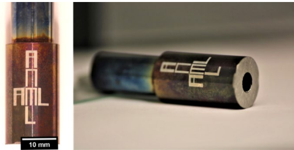
Figure 1. Conformal printing on a 16 mm diameter Haynes 244 tube
