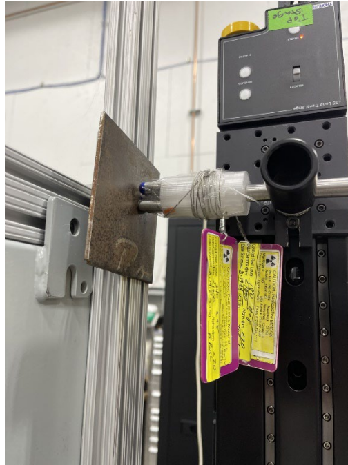
Figure 8. Detector count rate measurement setup using five neutron sources.
