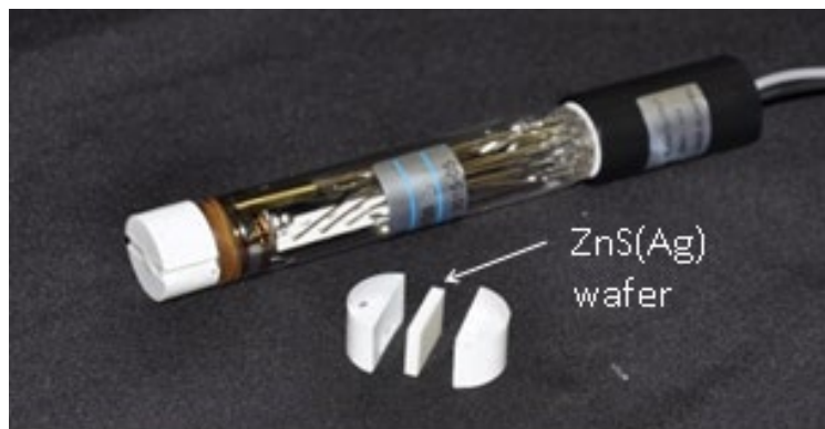
Figure 2. Hodoscope detector components including the proton recoil scintillator (in white) coupled to the photomultiplier tube.
