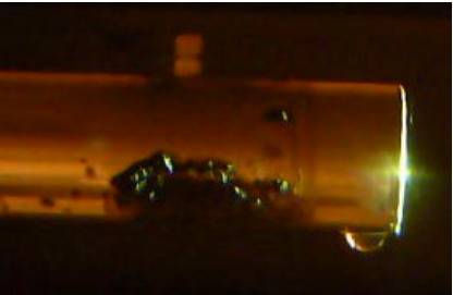
MINOS NT-01 target containment water leak (FNAL)
