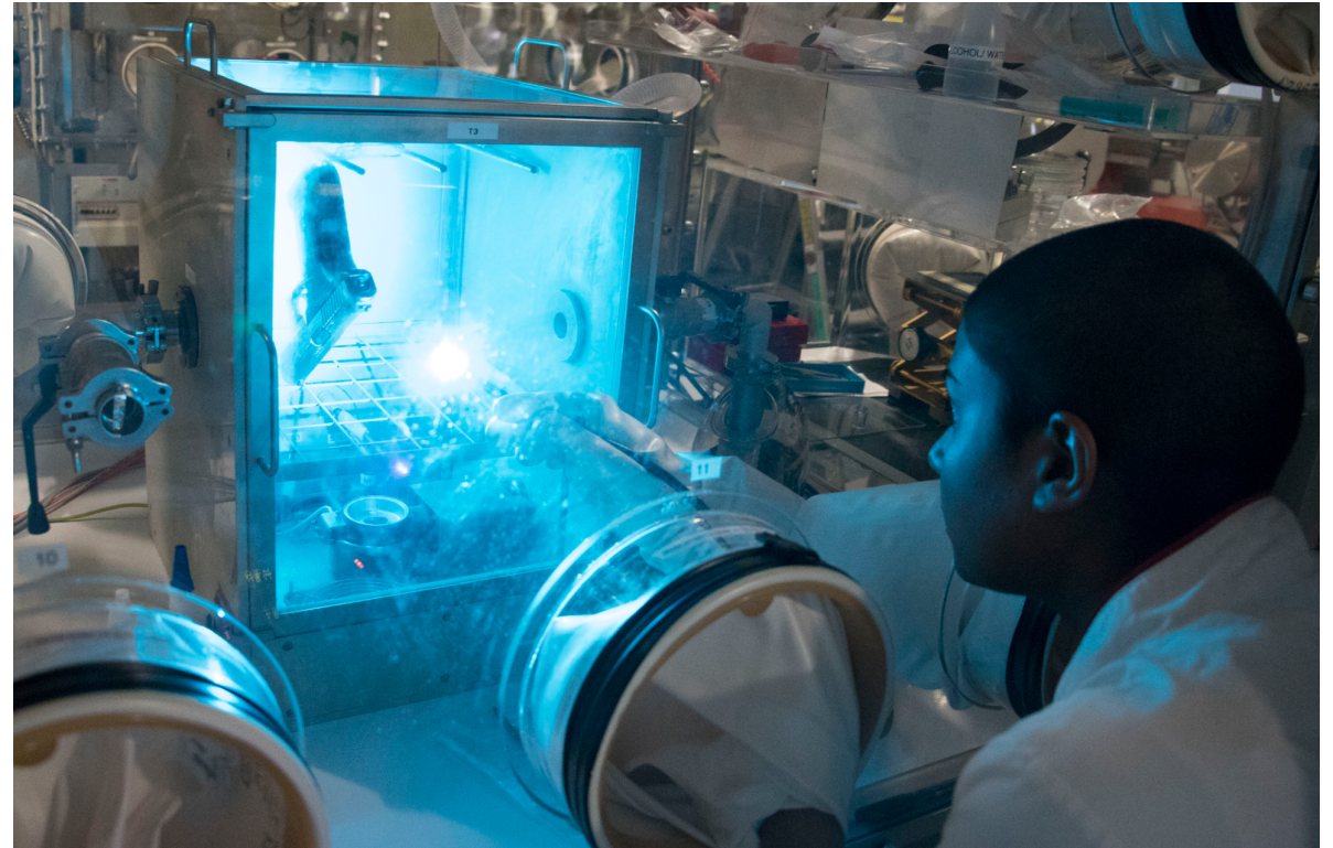
Cyanoacrylate fuming inside a glovebox of a piece of evidence collected from a radiological crime scene during an exercise with the German police
