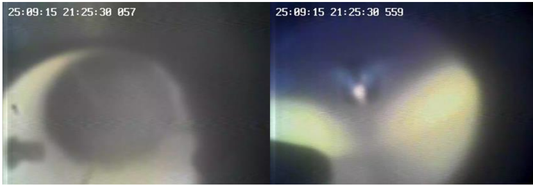
Figure 3 – (a) Micro Mixer and two H 2 AFS injectors on 100% Hydrogen (b) Hammer Head injector on 100% Hydrogen.
