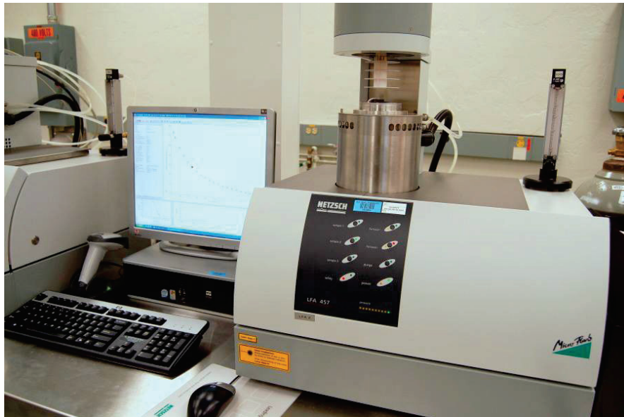
Figure 10. LFA measurement station for determining thermal diffusivity.
