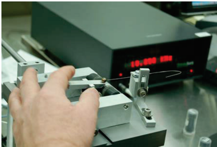
Figure 8. Fundamental frequency measurement station.
