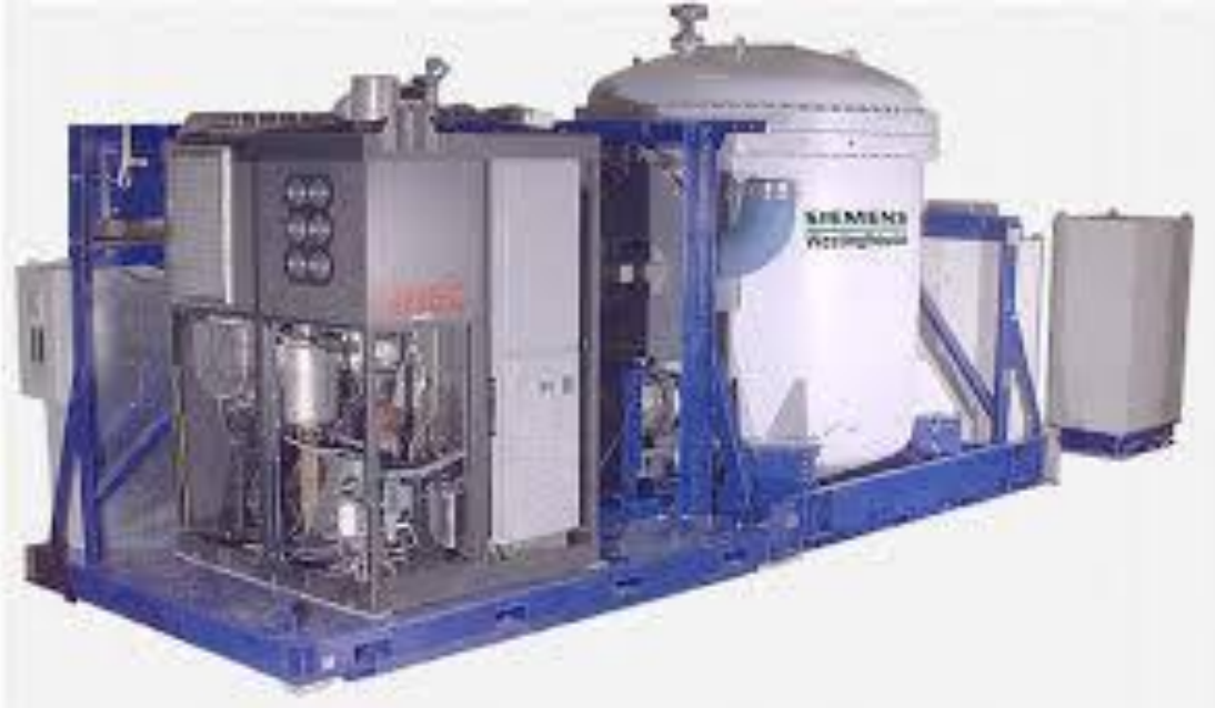
Siemens Westinghouse pilot demonstration 220 kW Solid Oxide Fuel Cell – Gas Turbine (SOFC-GT) Hybrid.
