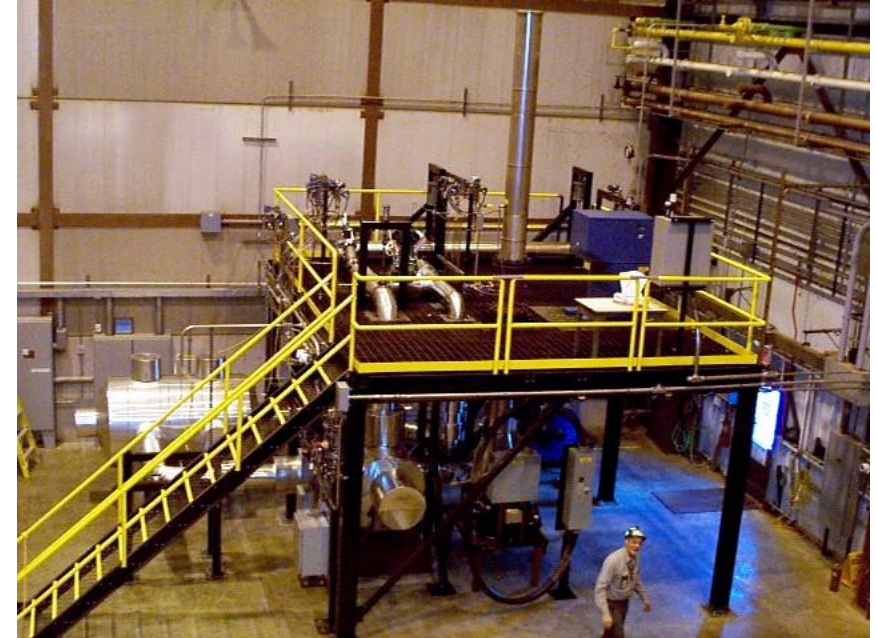
NETL cyber-physical system 400 kW SOFC-GT Hybrid.
