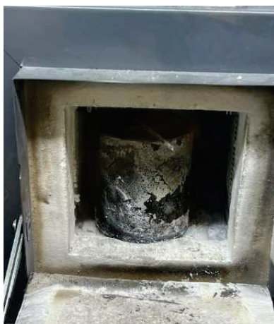
Figure 24. Condensation of salt vapors observed on the outer surface of the crucible and along the interior walls of the furnace following thermal cycling. These deposits are indicative of partial vaporization of NaCl–MgCl 2 salt during repeated exposures to peak temperatures slightly exceeding 700°C
