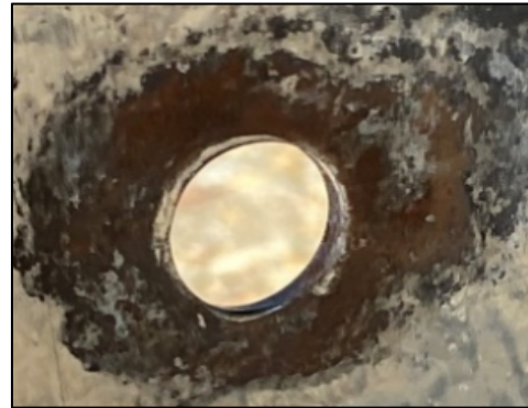
Image 13: Example of fretting wear of G90 purlin at the joint interface due to repeated joint slip.
