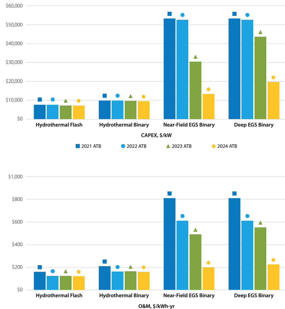
Figure 18. CAPEX (top) and O&M costs (bottom) for hydrothermal and EGS technologies from the 2021 ATB to the 2024 ATB. All costs are in 2022 dollars (the base year for the 2024 ATB).
