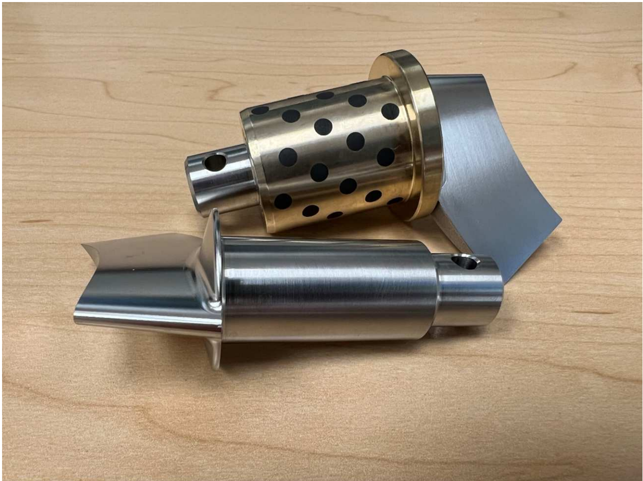
Figure 10. IGV Vane and Vane installed in Brass Bushing
