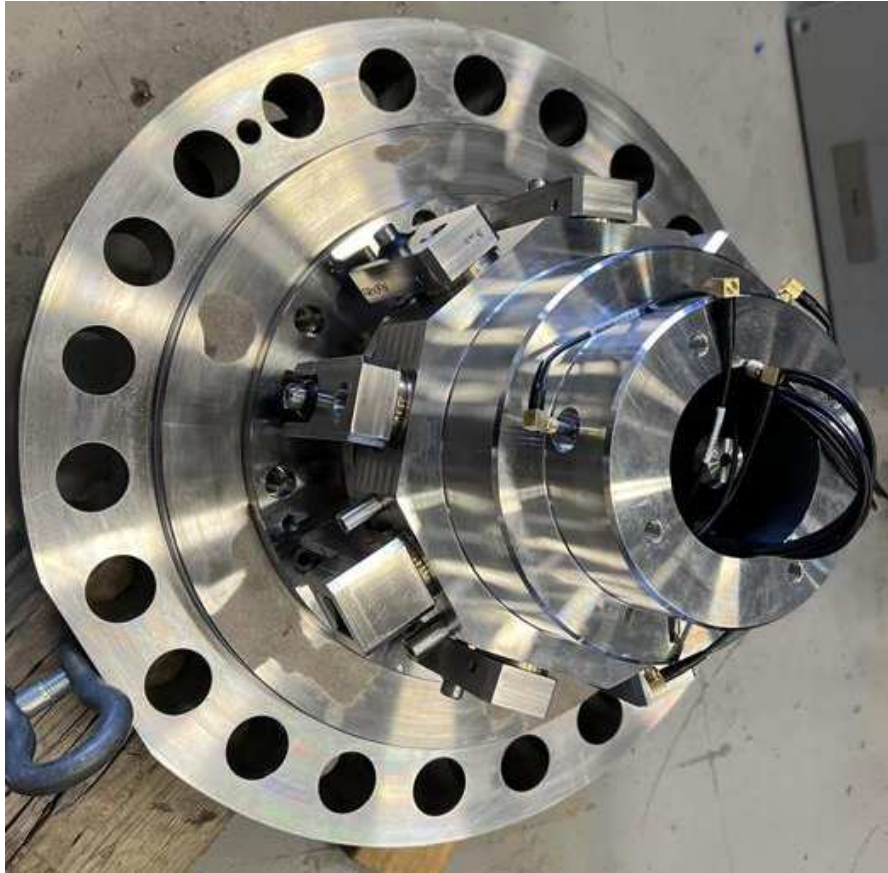
Figure 13. IGV assembly with dynamic pressure probes shown on the inlet duct.
