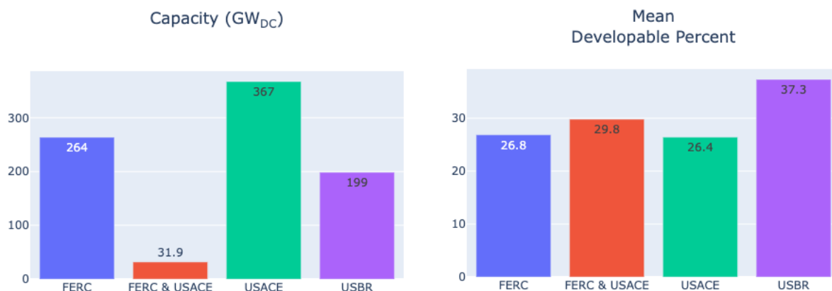
Figure 4. Distribution between the type of reservoirs of capacity and the FPV developable percent.
