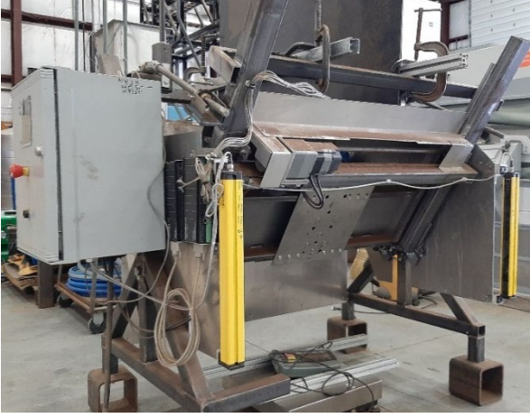
Figure 2: Lab scale adjustable hopper (left) and it's schematic (right).
