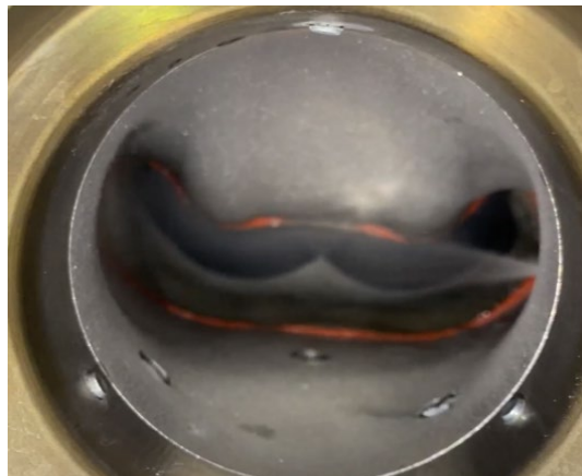
Figure 40: Horizontal spray pattern
