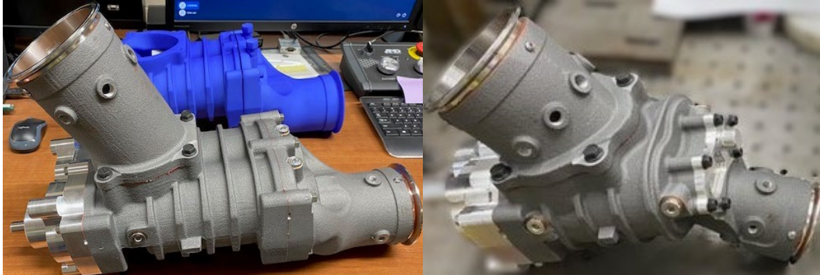
Figure 15: Picture of assembled compressor and expander
