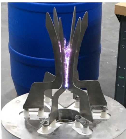
Figure 8. Operation of 3-pair electrode reformer.
