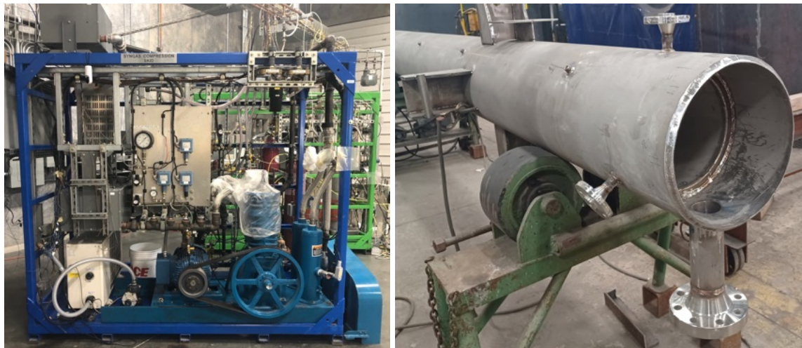
Figure 11. Fabrication of syngas compression skid (left) and FT cooling vessel (right).
