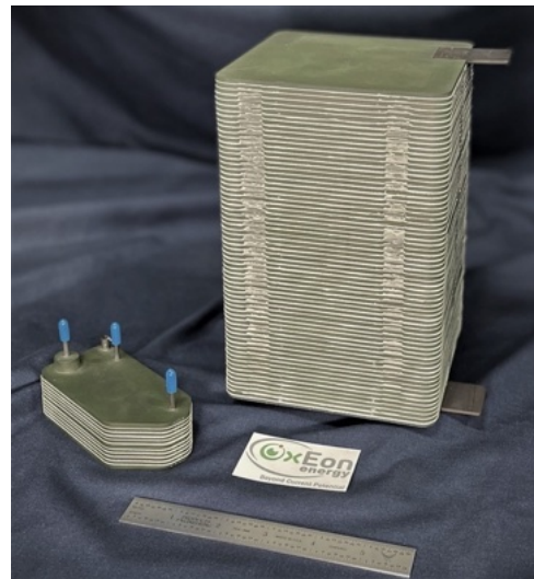
Figure 3. Comparison of SOXE stacks from MOXIE (left) and mission-scale (right).
