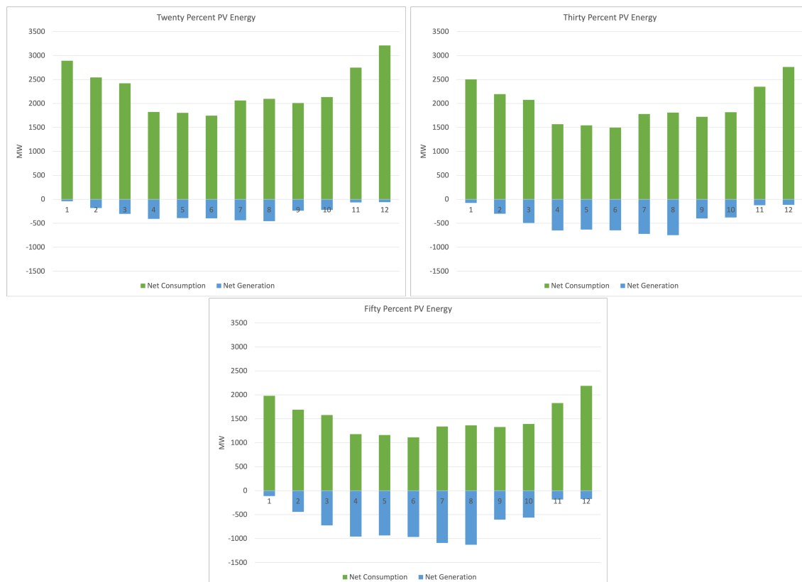
Figure 4: Monthly consumption and generation for three BTM solar levels: 20% , 30% , 50% (right).
