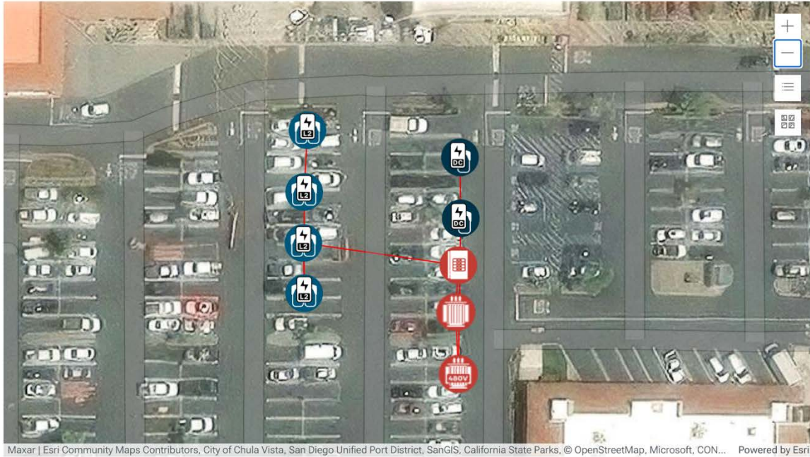
Figure 12. An example single-line site diagram shows the charging stations and essential electrical components—transformer(s), service panel, and electrical lines—generated by the GIS algorithm
