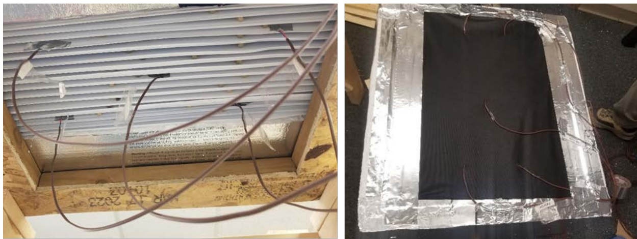
Figure 8. Thermocouple placements at the inlet and outlet of the heat exchanger
