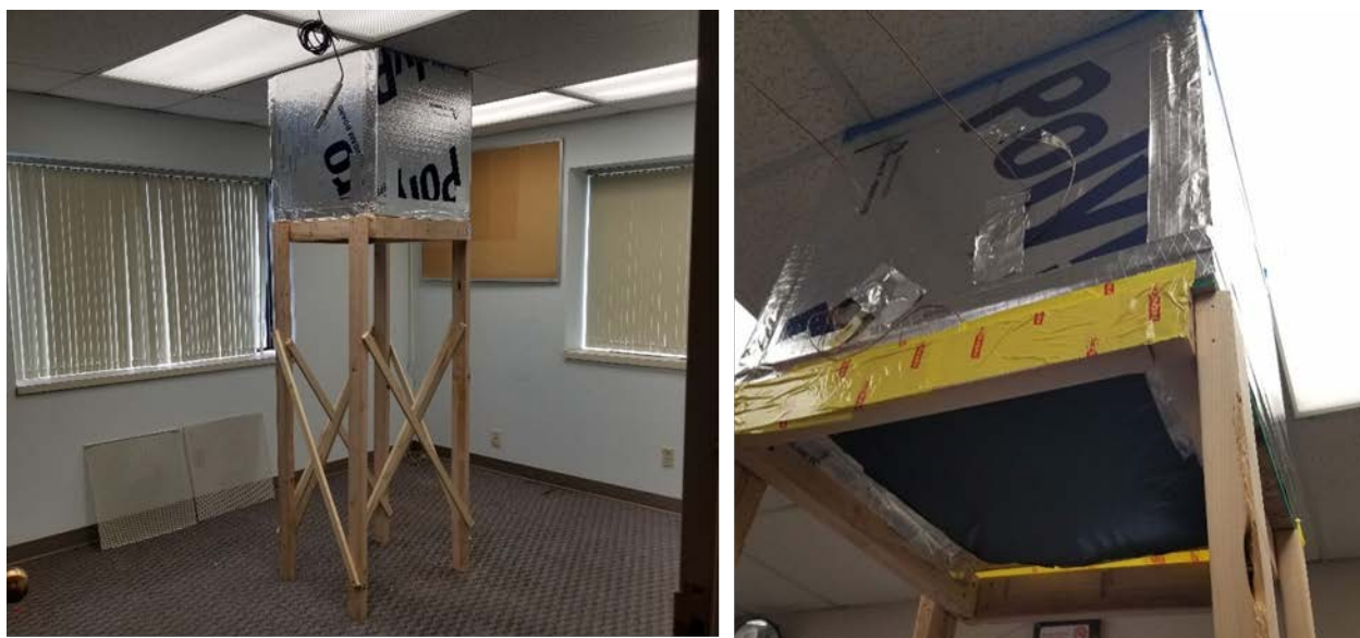
Figure 6. (Left) Insulated heat exchanger box with PCM. (Right) Landscape fabric attached to the outlet was used as a diffuser to distribute flow.
