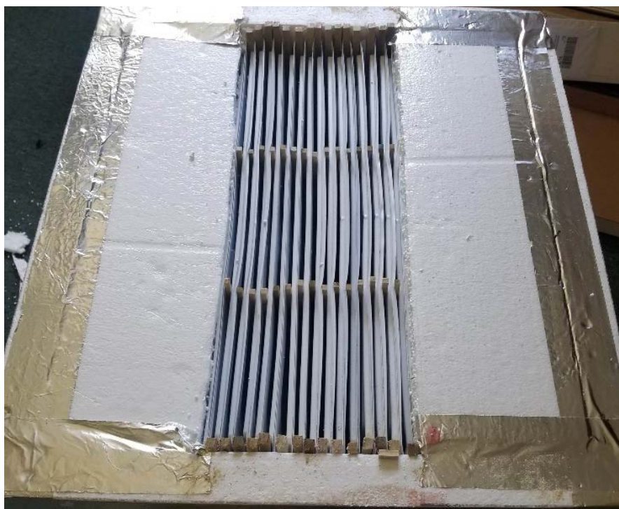
Figure 7. Heat exchanger inlet with PCM tile fins. The area is smaller than the diffuser size to increase airflow velocity across the PCM.
