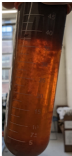
Figure 28: Colloidal solution of oxidized coal after ultrasonication and resting for 2 h
