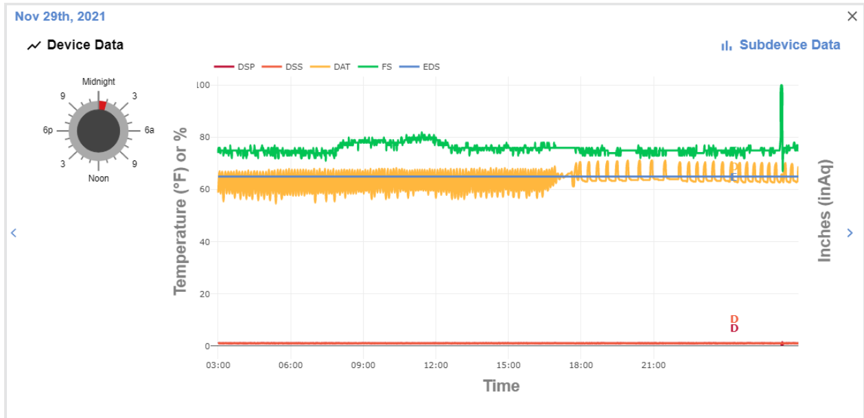
Figure 4-14. Supply Temperature Set Point is Constant for AHU-11-NORTH
