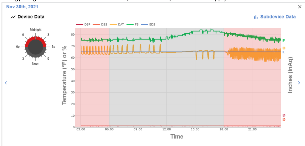
Figure 4-11. AHU-11-SOUTH Operating Continuously During Unoccupied Hours
