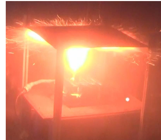
Venting prismatic cell ejecting particles and gas
