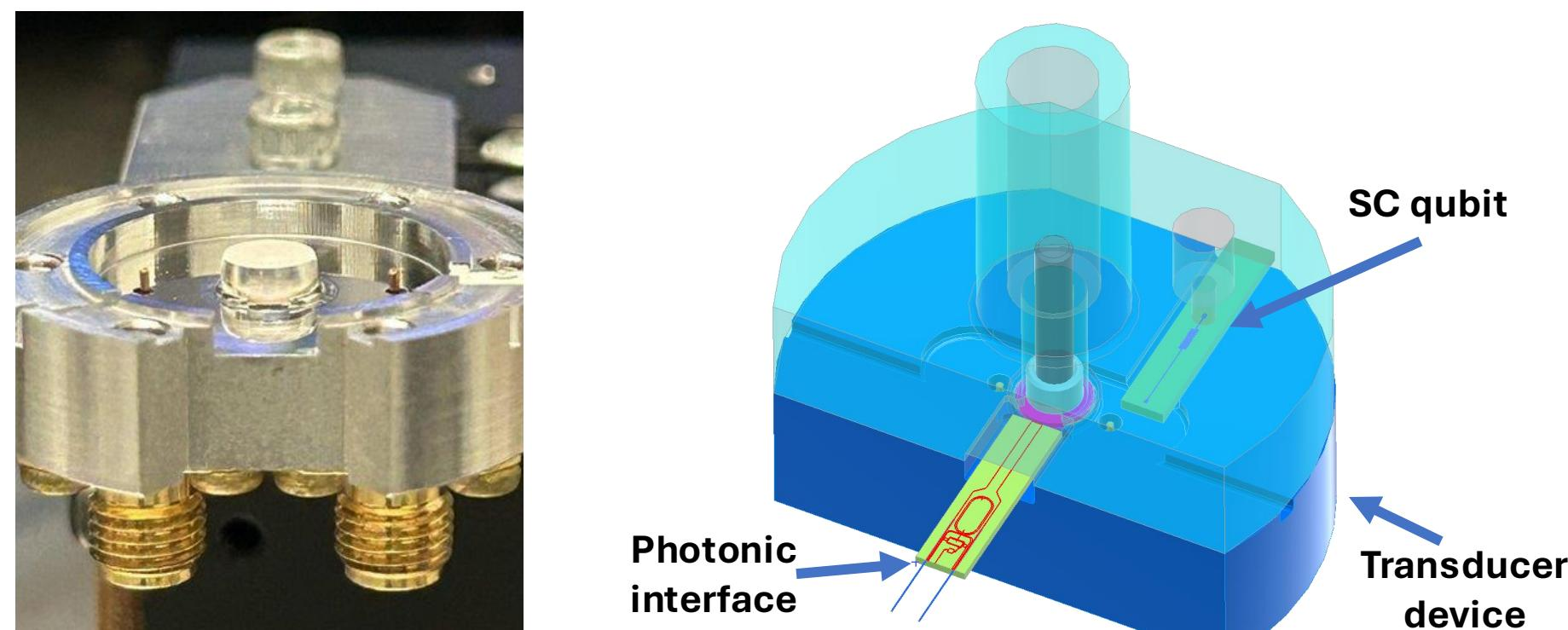
The electro-optic effect provides direct conversion and two-mode squeezing through three-wave mixing.
