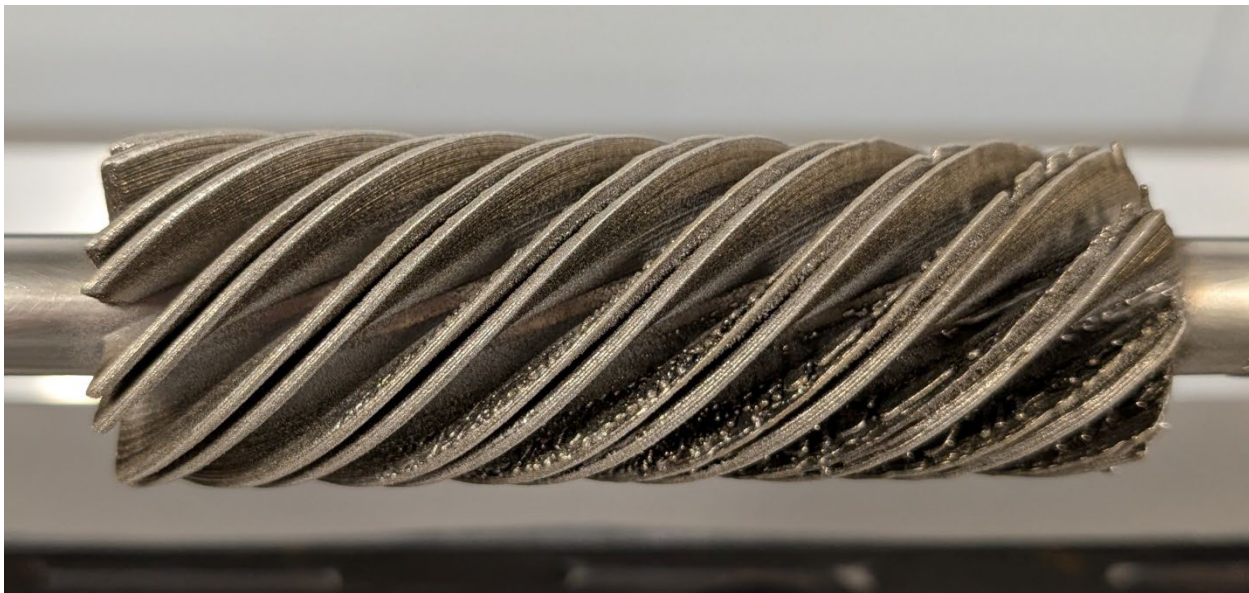
Fig. 25: Over-melting on 8x print.
