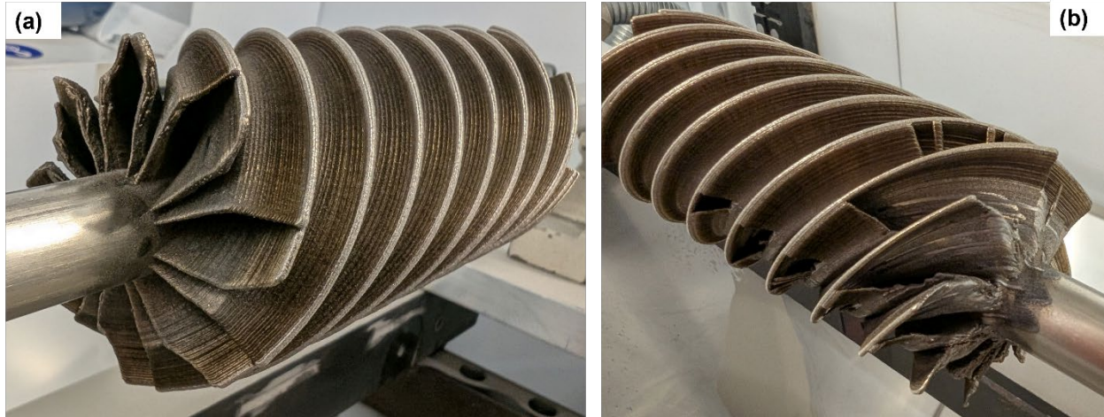
Fig. 30: 8x build errors. (a) Constrained side. (b) Free side.
