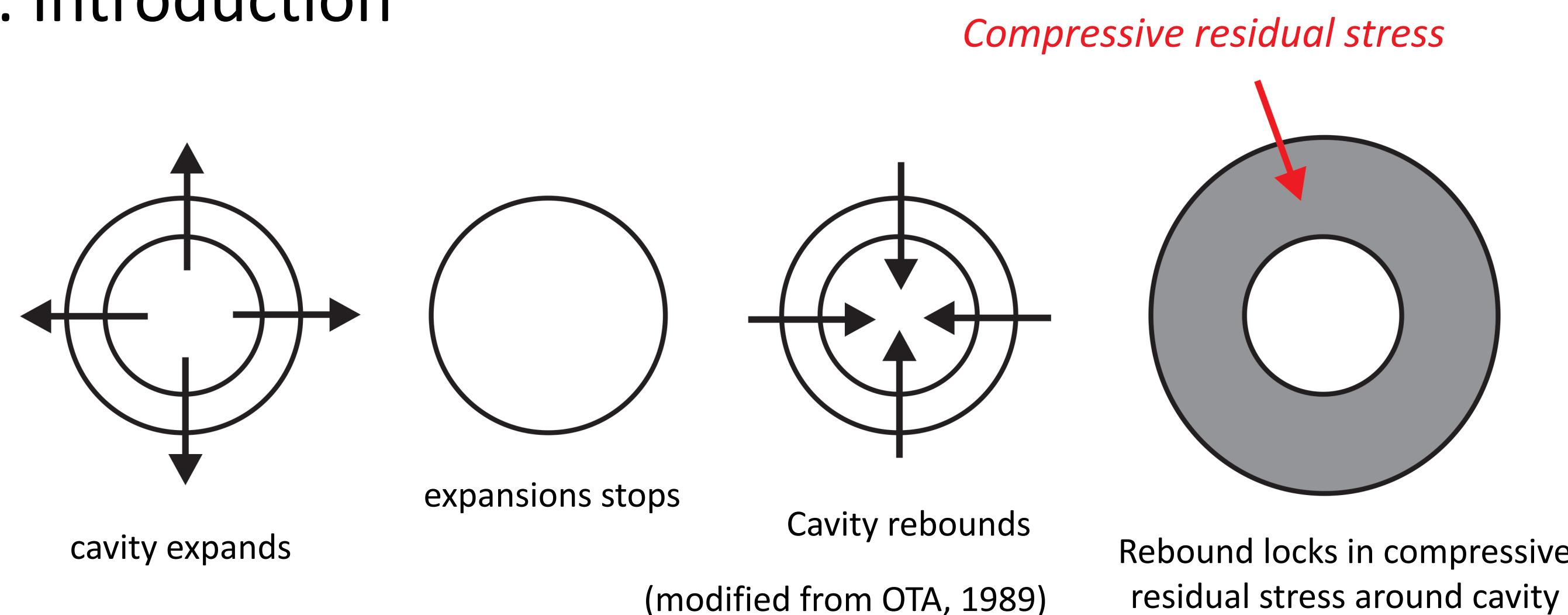
Formation of a compressive residual stress cage around an explosively formed subsurface cavity acts to close fractures and contain debris, including liquids, gases, and particulates. We have developed a new **meso-scale** geomechanics capability using an 8.84-m (29-ft) radius centrifuge for physically simulating underground chemical explosions and potential stress cage processes in scaled geologic models.
