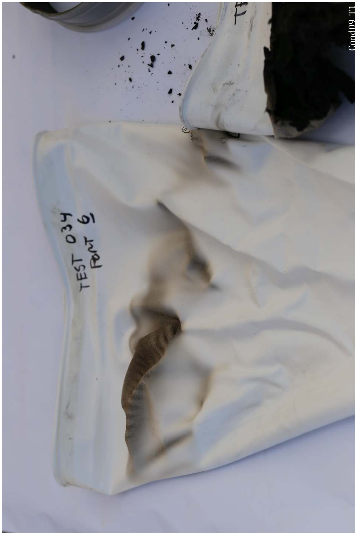
Figure 172: Condition 09 Trial 1. The port 6 glove sustained slight damage near the ring.
