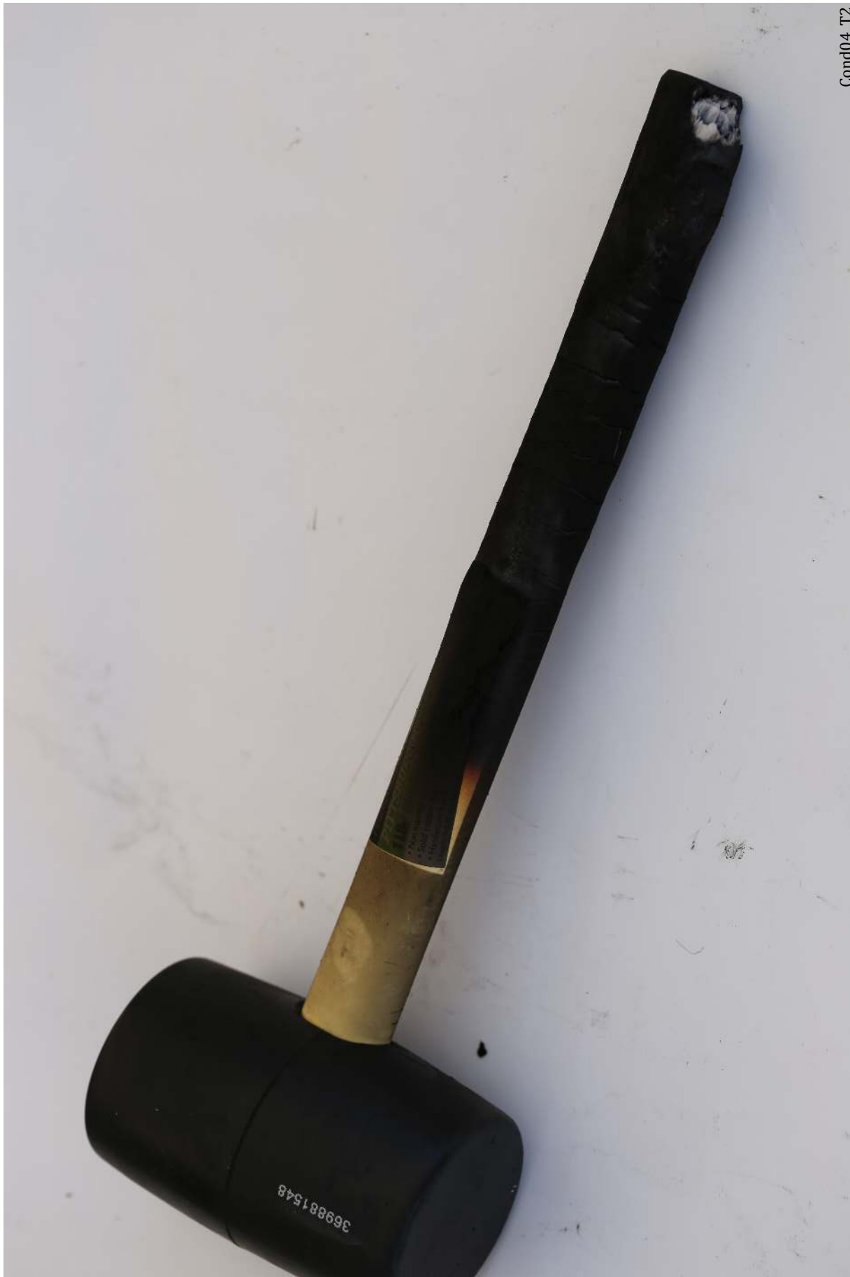
Figure 123: Condition 04 Trial 2. The mallet handle sustained a fire and was nearly completely charred.
