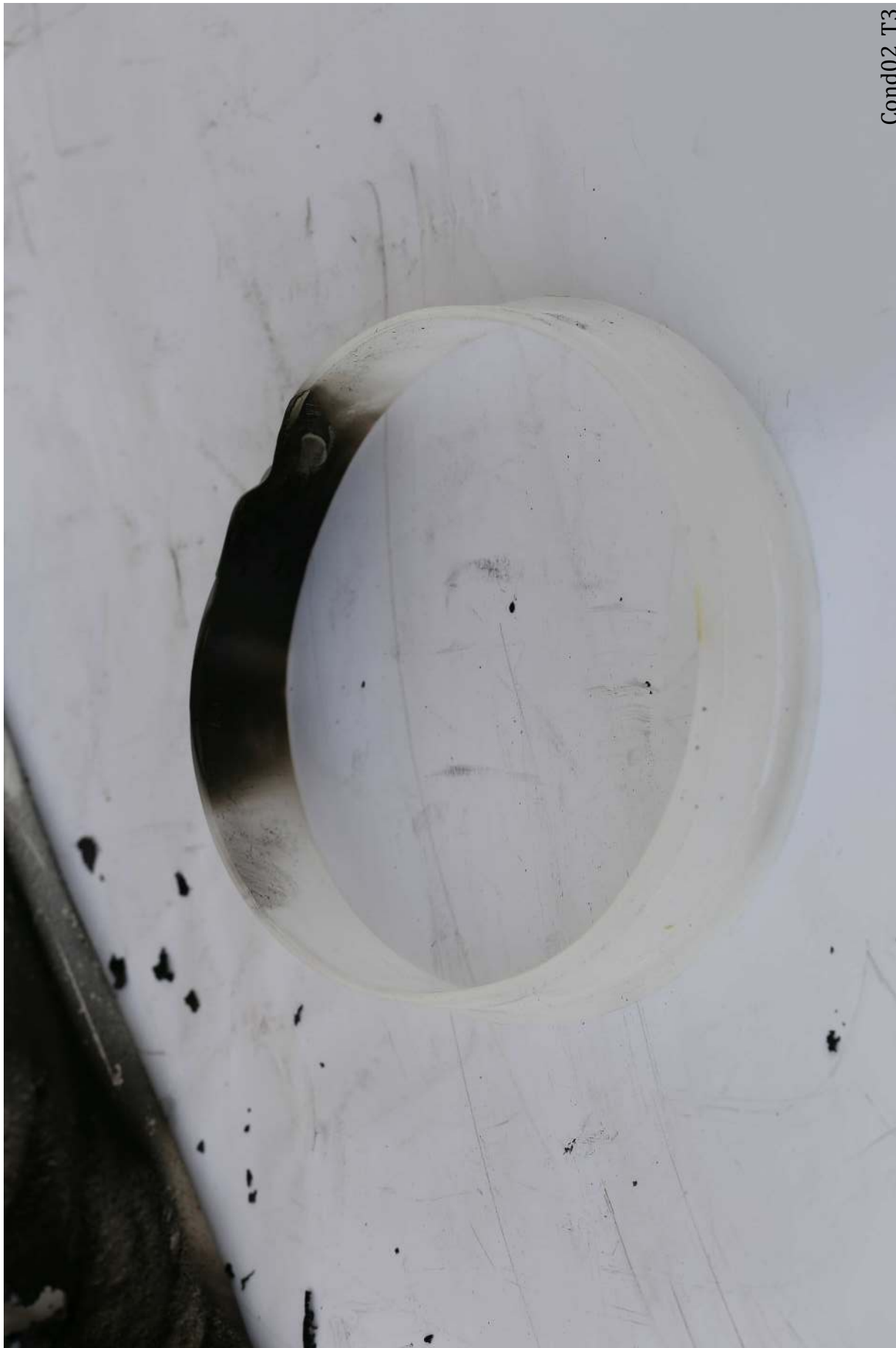
Figure 93: Condition 02 Trial 3. The port 10 ring was blackened and partially melted.
