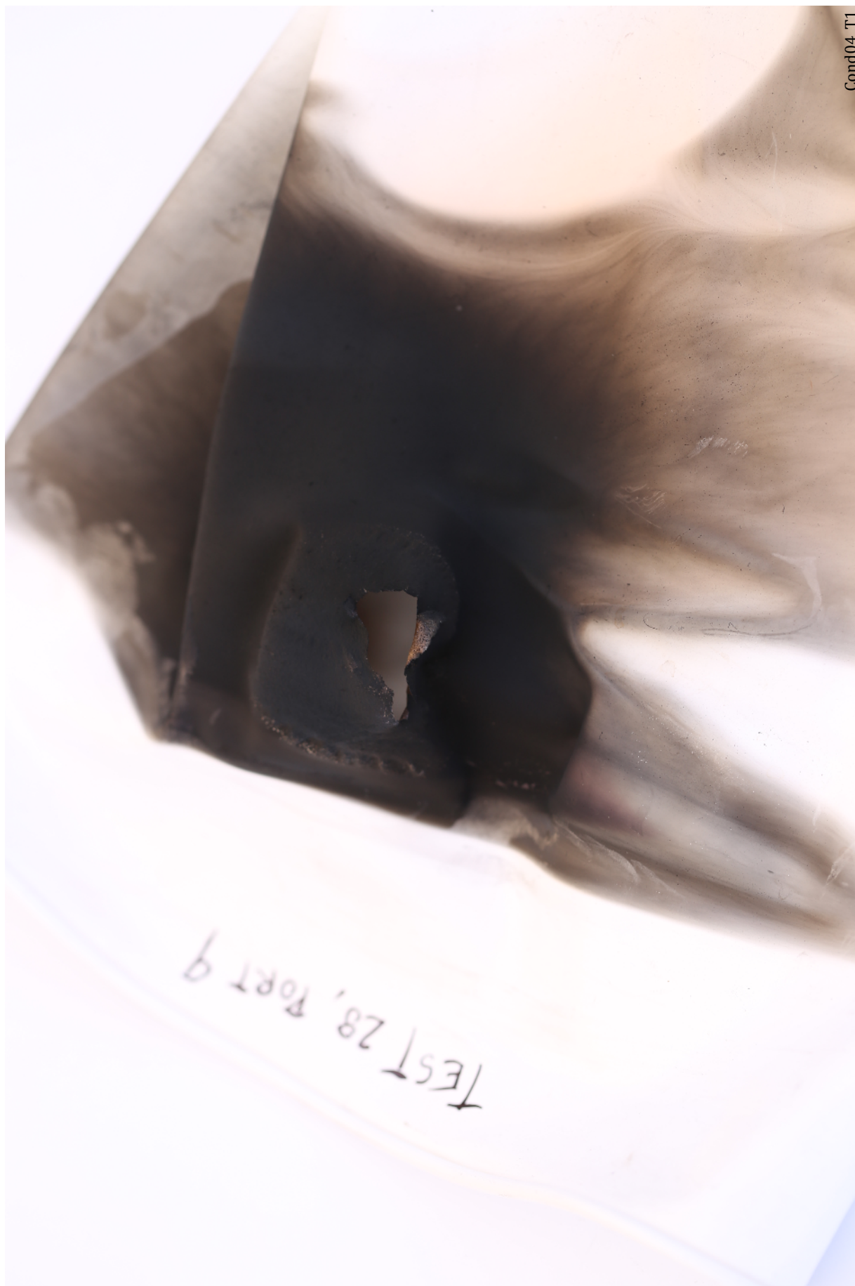
Figure 117: Condition 04 Trial 1. A small hole was evident in the port 9 glove.
