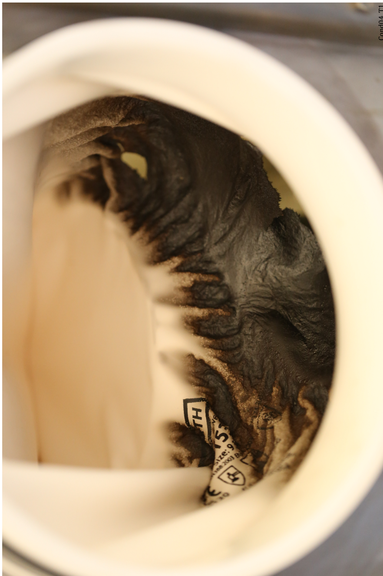
Figure 118: Condition 04 Trial 1. Charring, bubbling, and cracking occurred near the ring of the port 9 glove.
