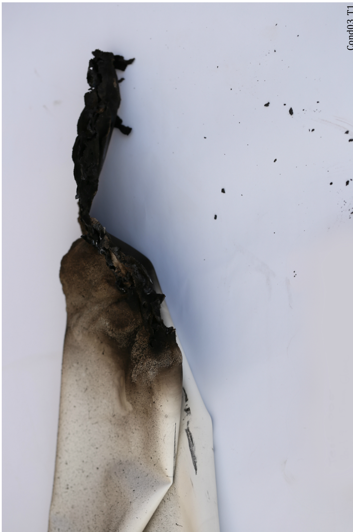
Figure 103: Condition 03 Trial 1. The hand of the port 9 glove was consumed.
