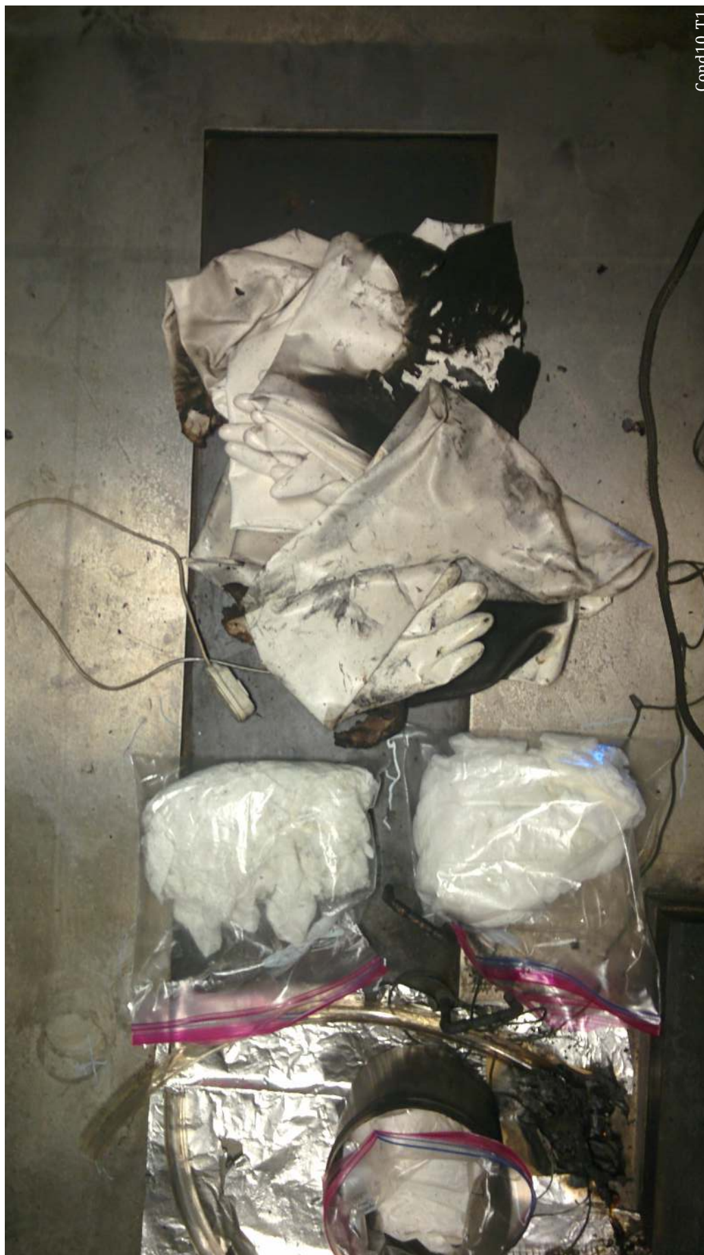
Figure 190: Condition 10 Trial 1. Gloves piled across the GB from the igniters were not involved.
