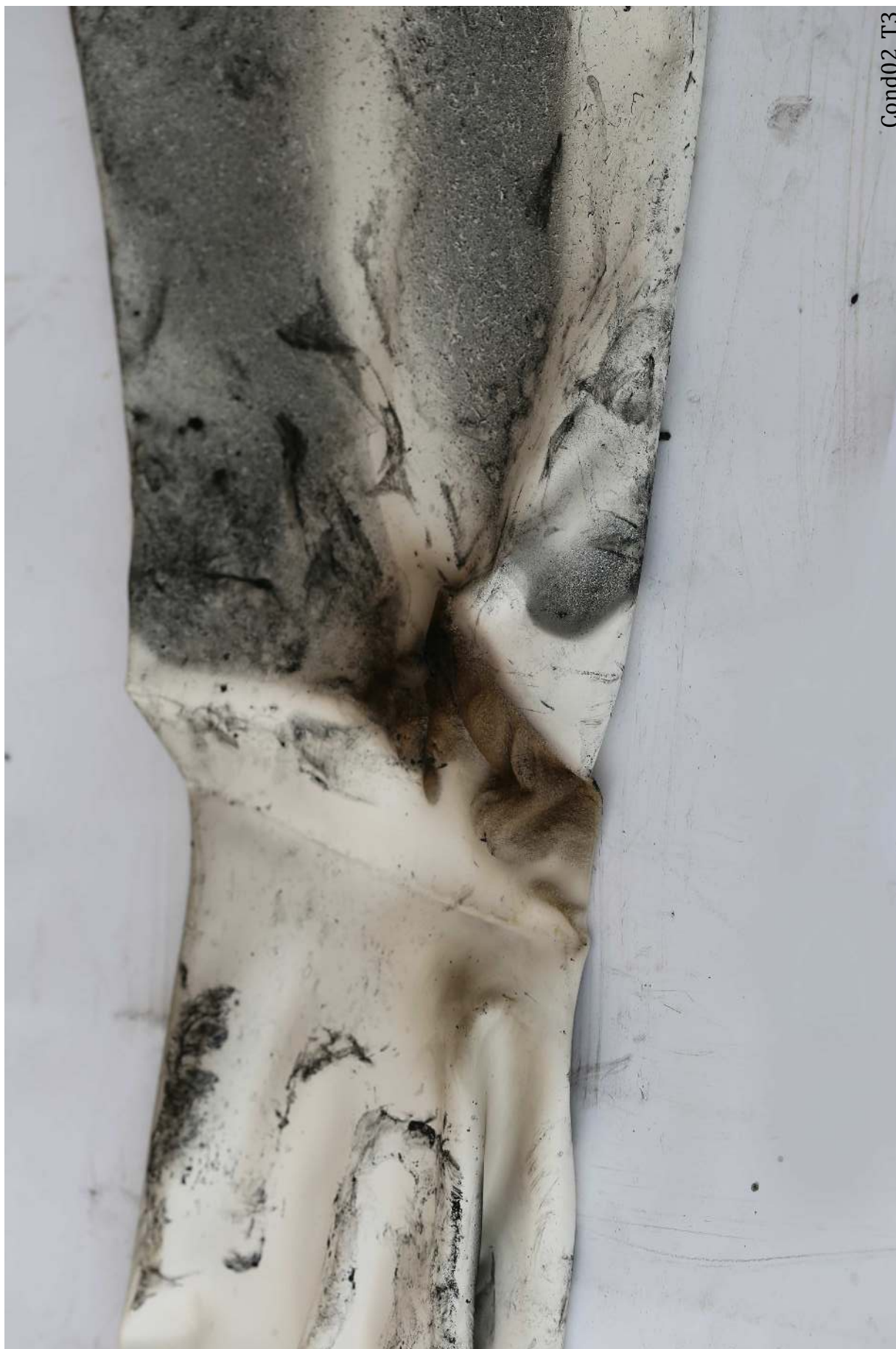
Figure 94: Condition 02 Trial 3. Minor bubbling is apparent on the port 24 glove.
