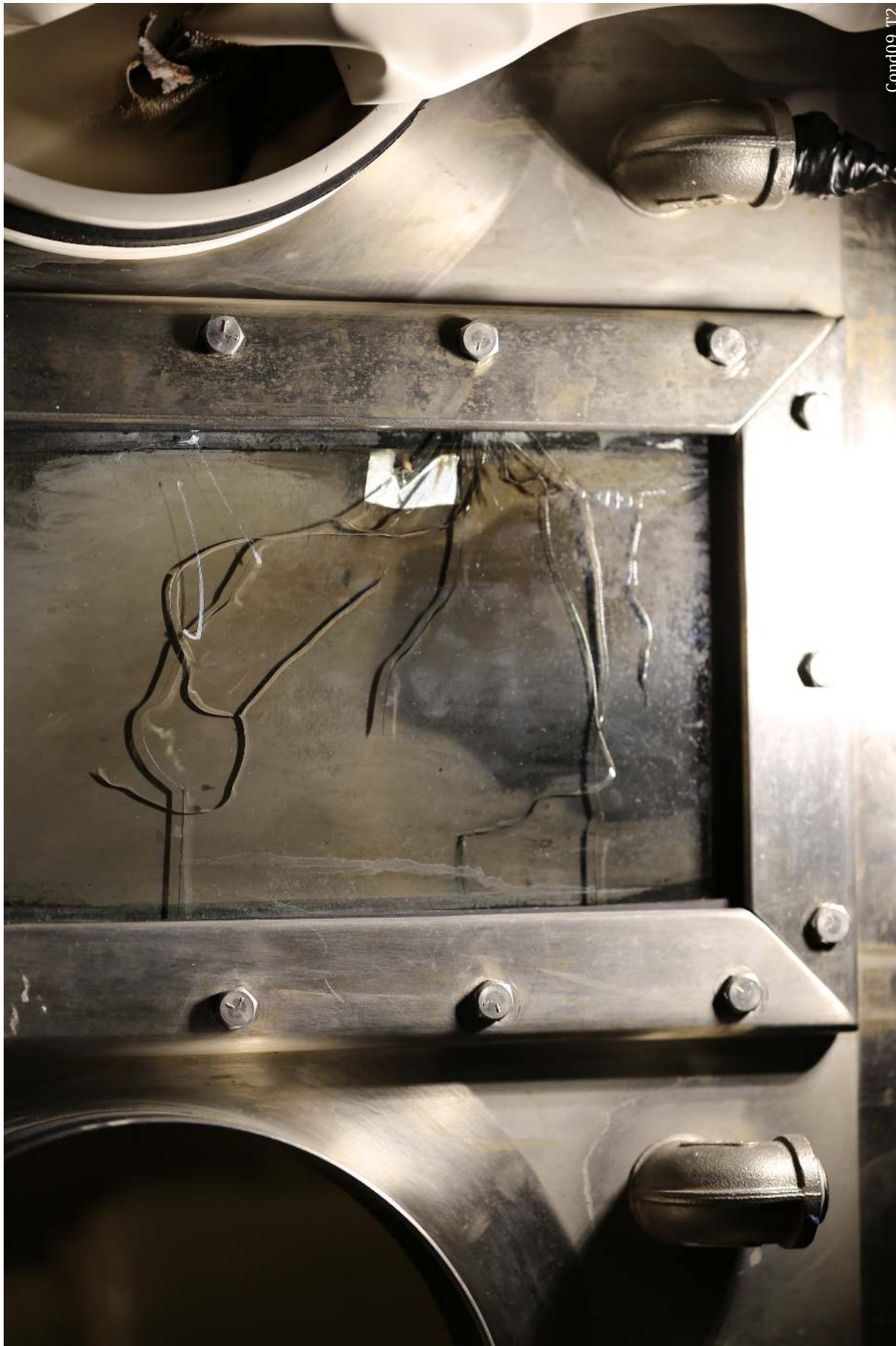
Figure 174: Condition 09 Trial 2. The fire cracked the window between port 9 and port 10.
