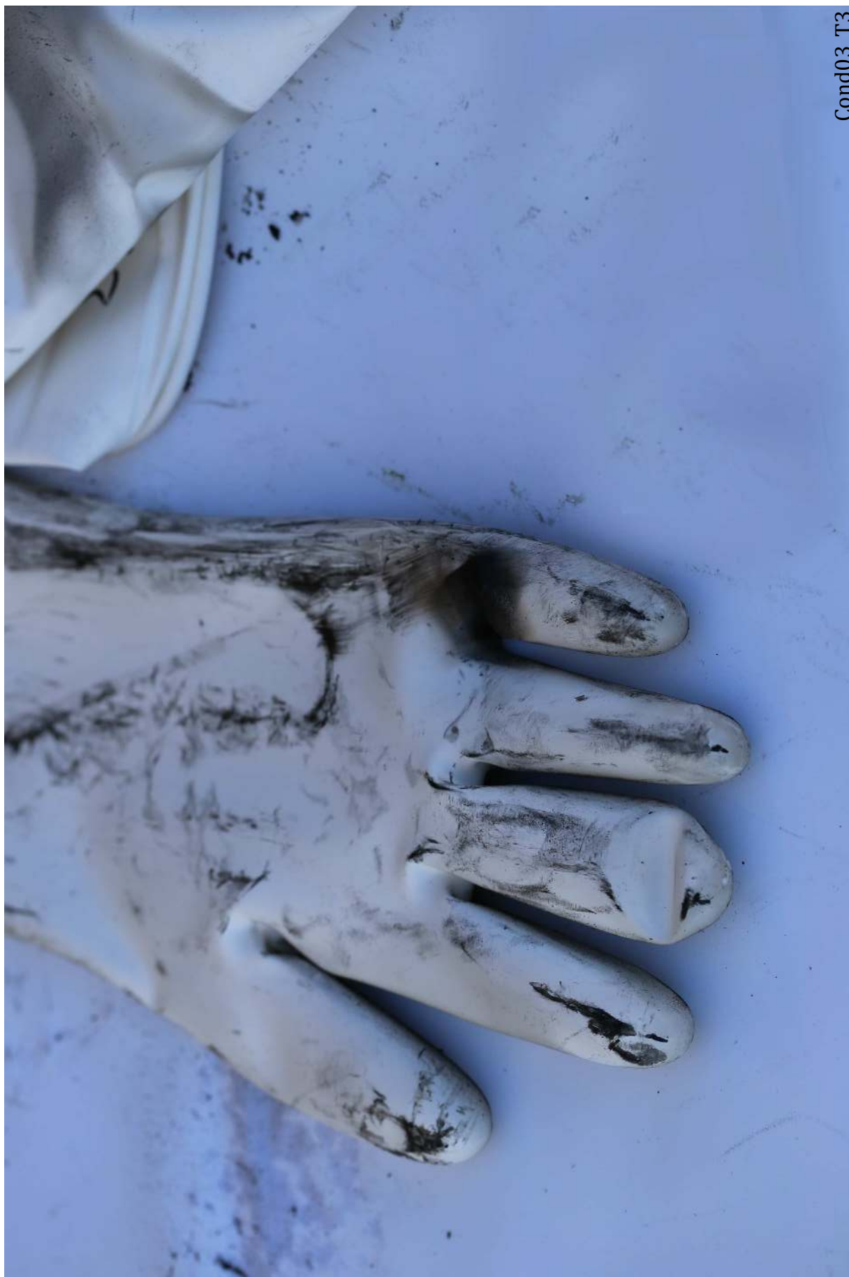
Figure 113: Condition 03 Trial 3. Minor Damage was inflicted on the fingers of the port 23 glove.
