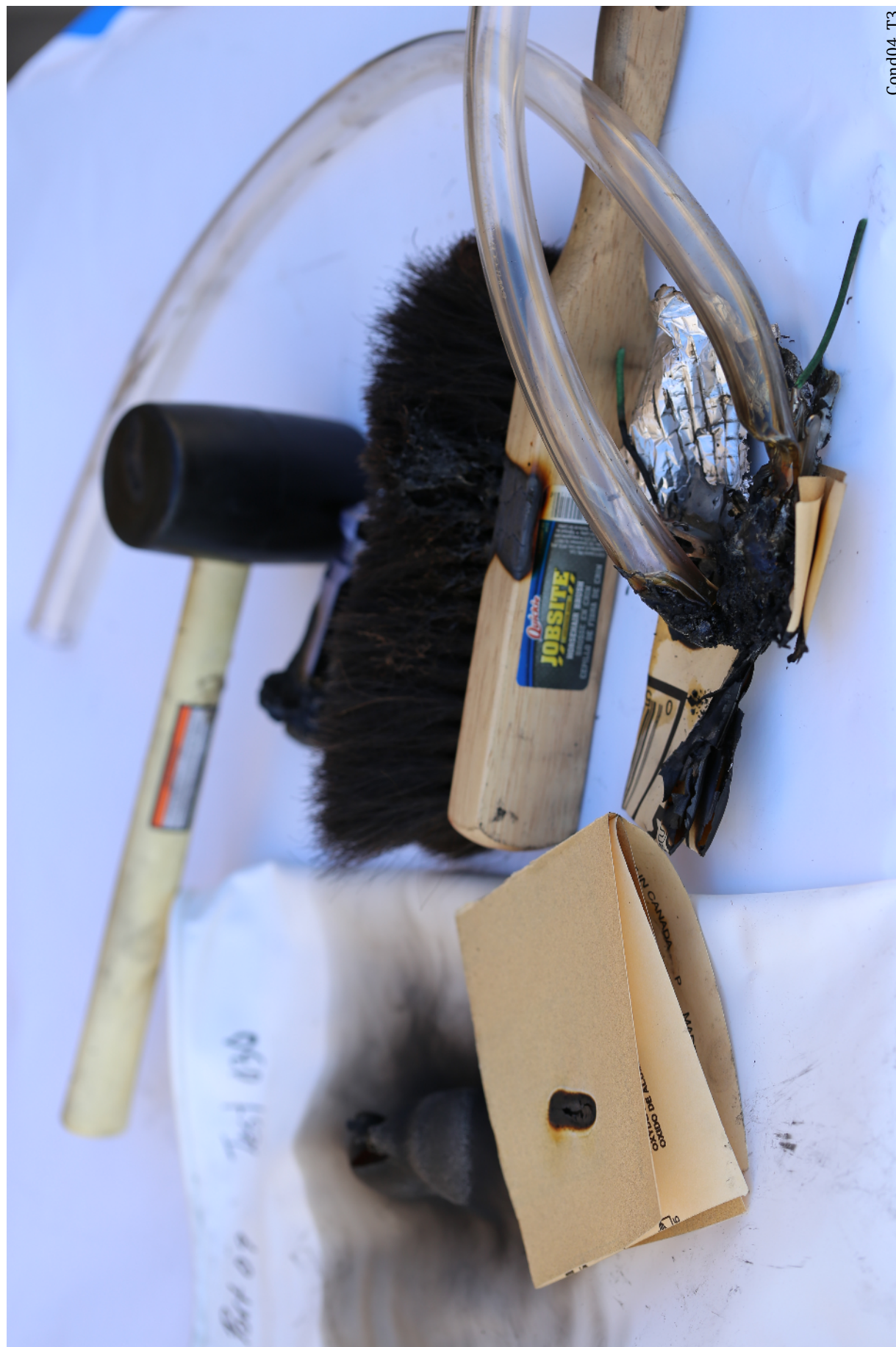
Figure 128: Condition 04 Trial 3. Tygon tubing, horsehair, and sandpaper contributed to the fire.
