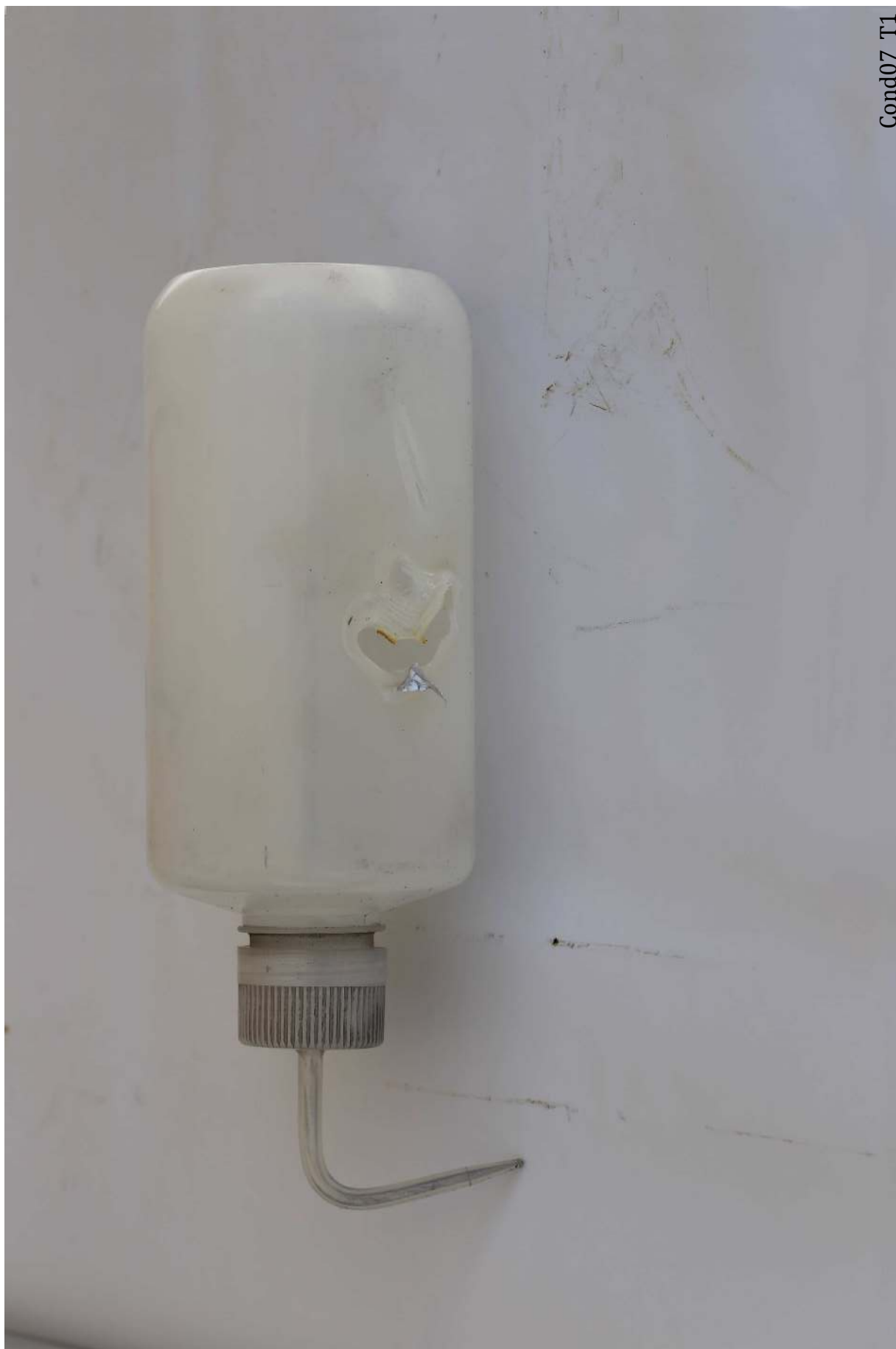
Figure 149: Condition 07 Trial 1. The igniter melted a small hole in the empty polypropylene bottle.
