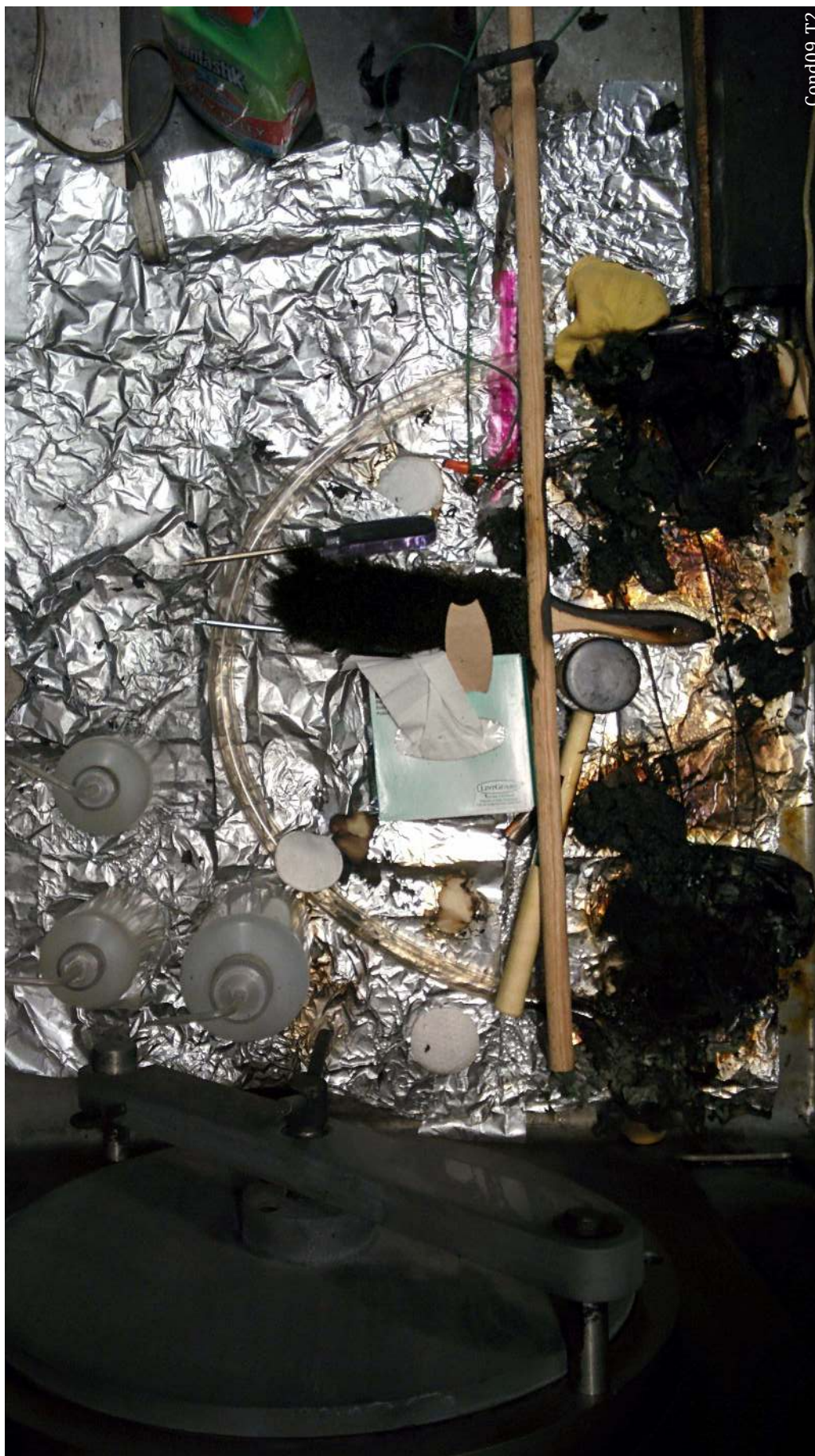
Figure 173: Condition 09 Trial 2. Consumables were burned severely and several gloves in port covers were breached.
