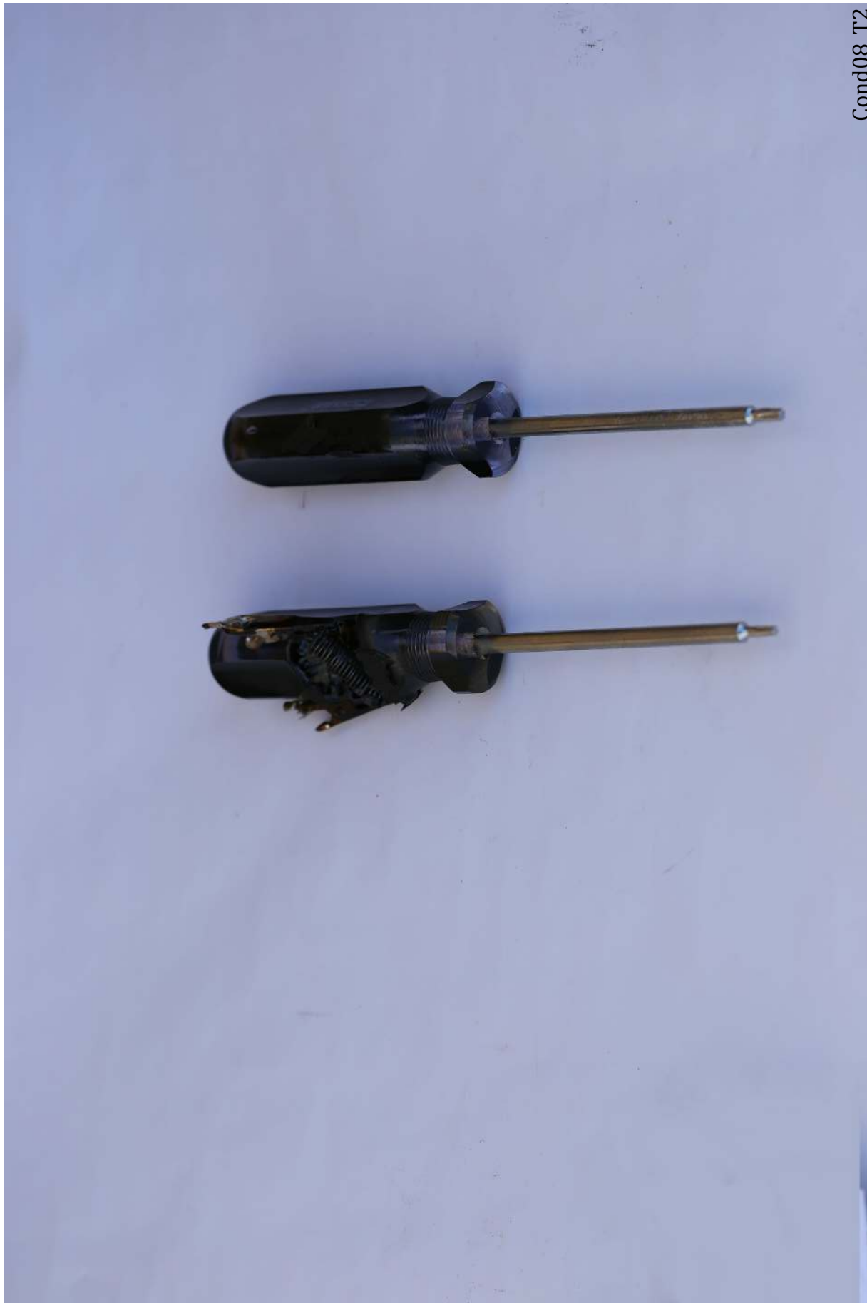
Figure 159: Condition 08 Trial 2. Screwdrivers charred and melted where they contacted the igniter.
