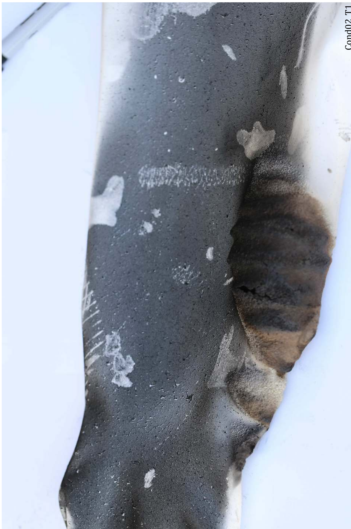
Figure 79: Condition 02 Trial 1. Bubbling and cracking are apparent on the port 10 glove.
