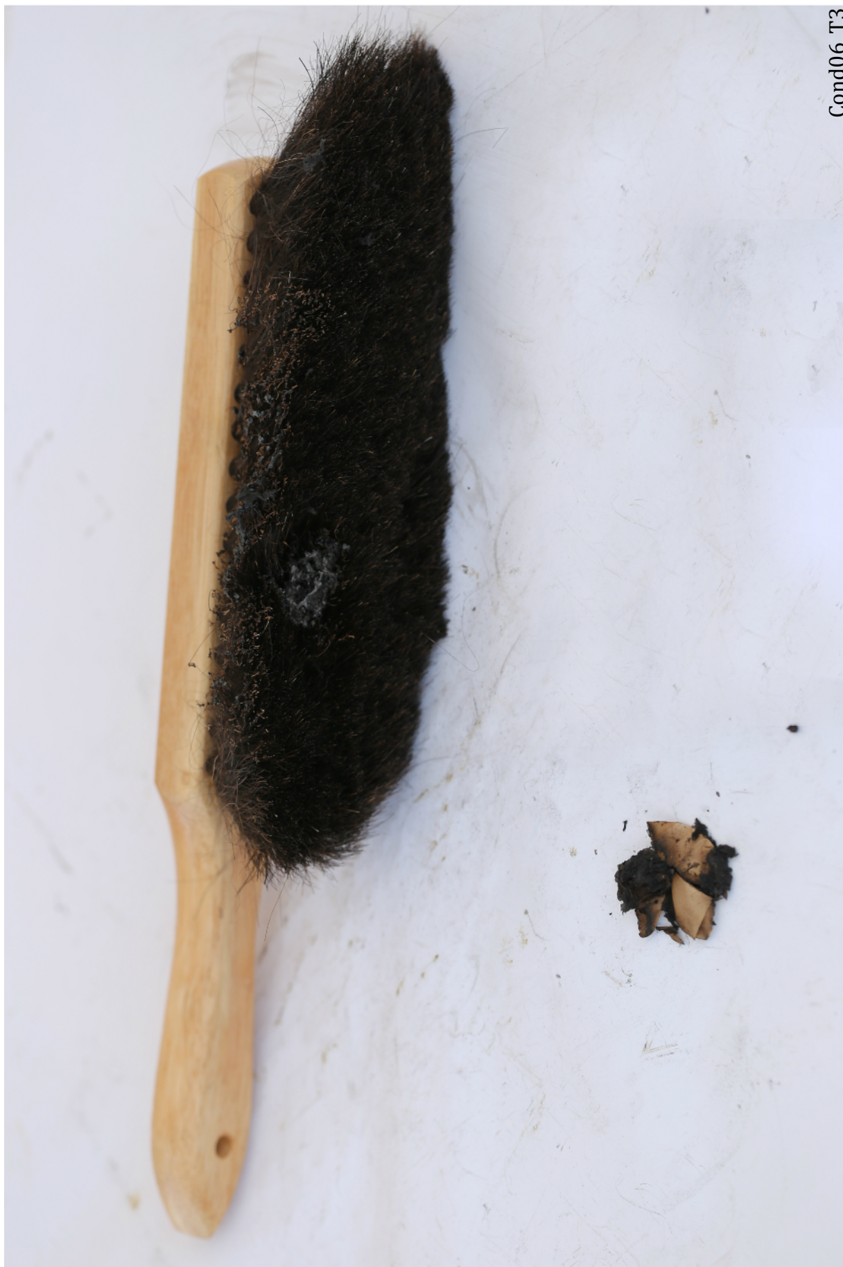
Figure 147: Condition 06 Trial 3. The horsehair brush was lightly singed and task wipes were burned.
