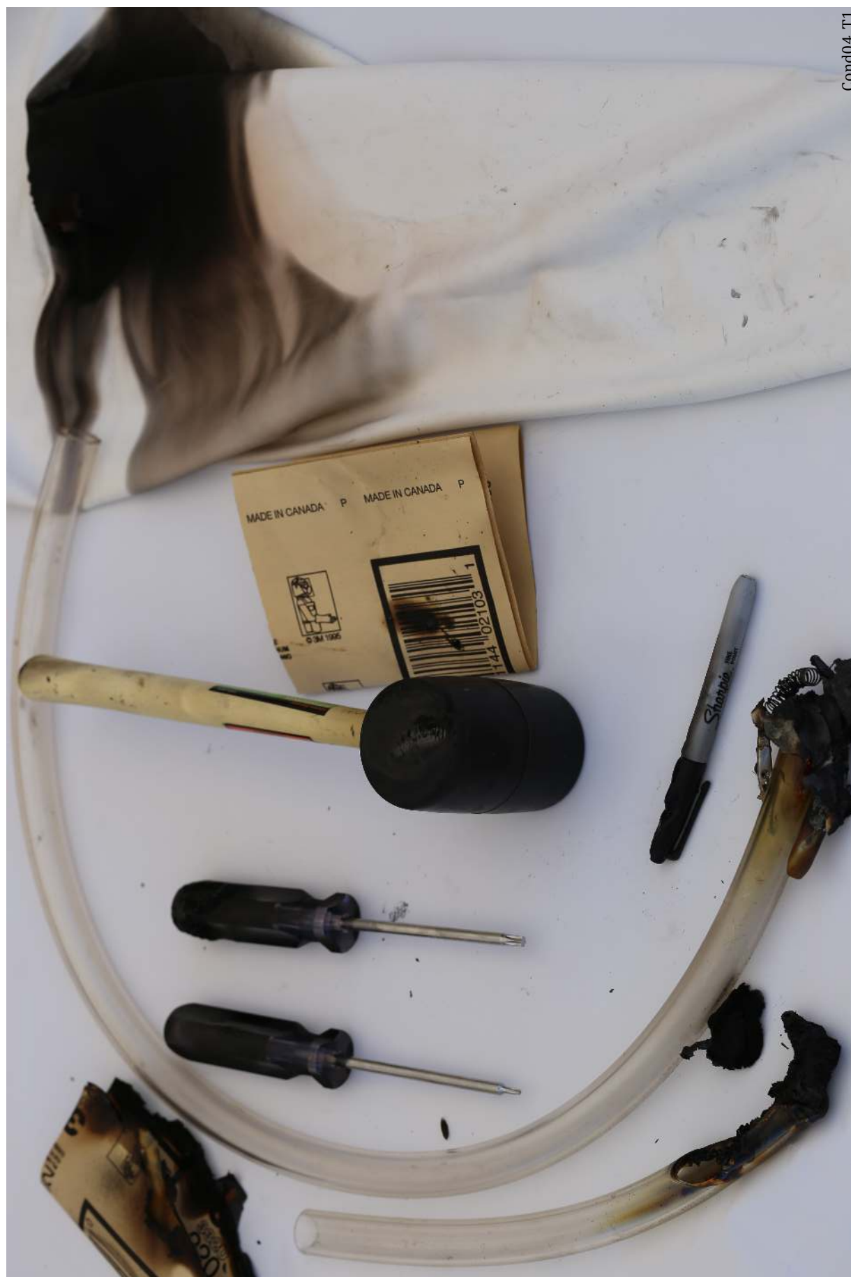
Figure 116: Condition 04 Trial 1. Tygon tubing, a marker, and sandpaper contributed to the fire.
