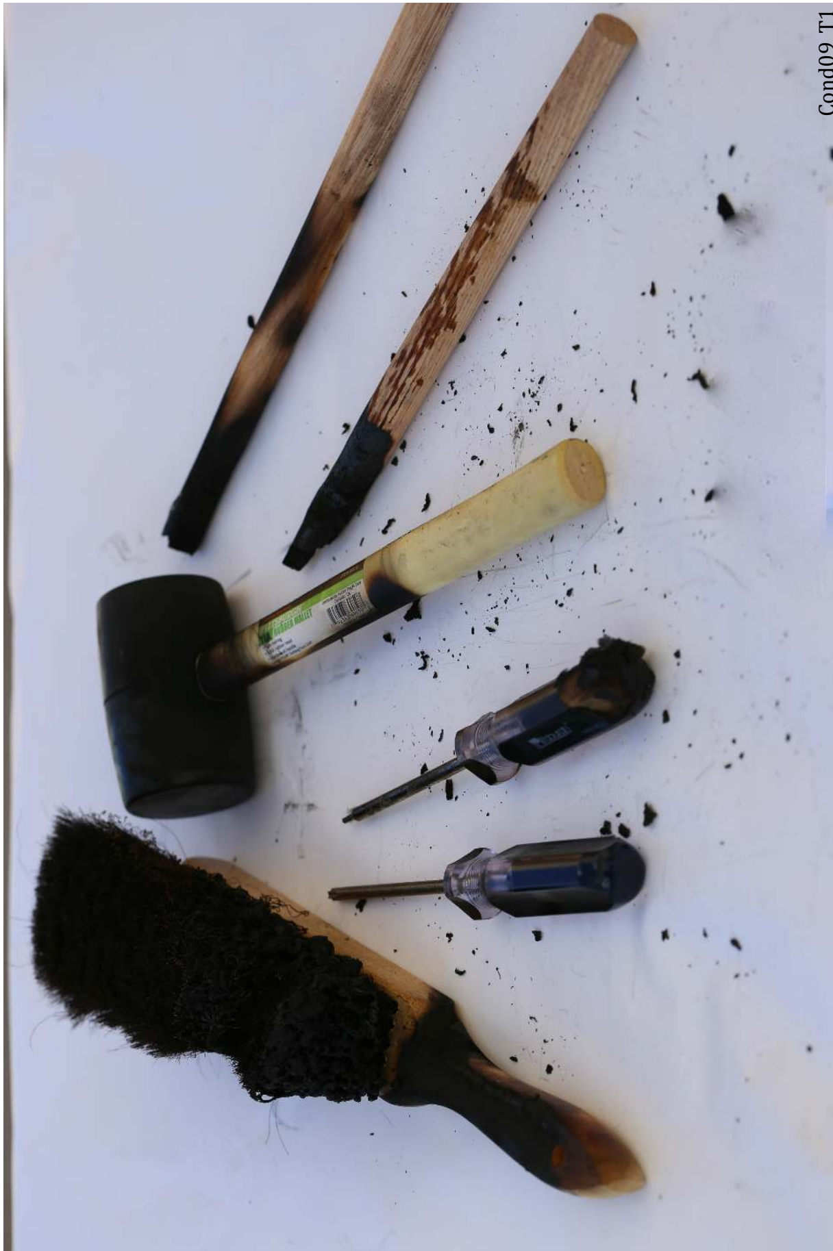
Figure 166: Condition 09 Trial 1. The horsehair brush, screwdrivers, mallet, and wooden dowel were all charred and burned.
