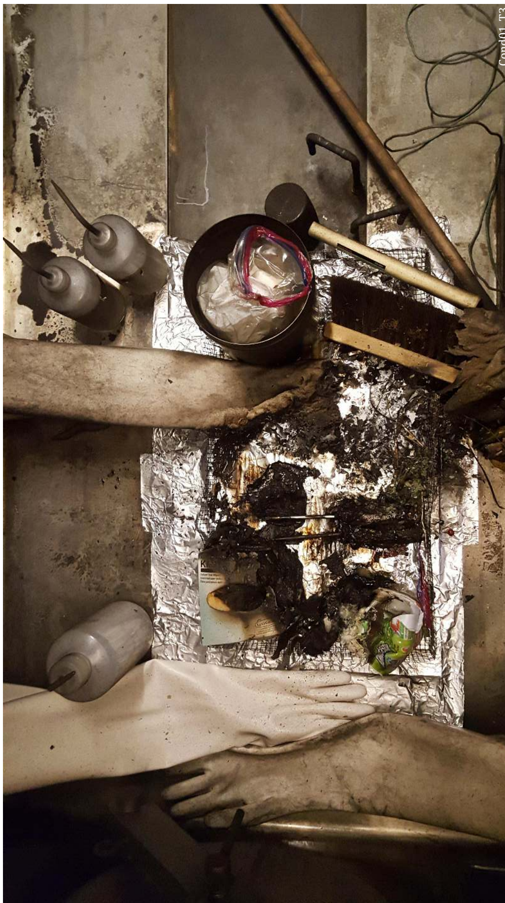
Figure 73: Condition 01 Trial 3. A large fire destroyed several gloves and consumables.
