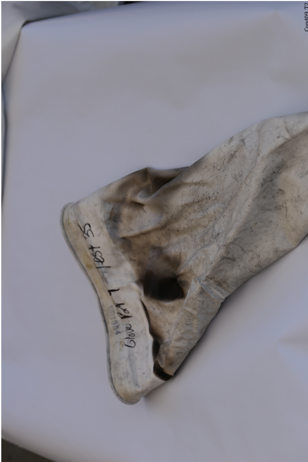
Figure 177: Condition 09 Trial 2. The port 7 glove was damaged near the port ring.
