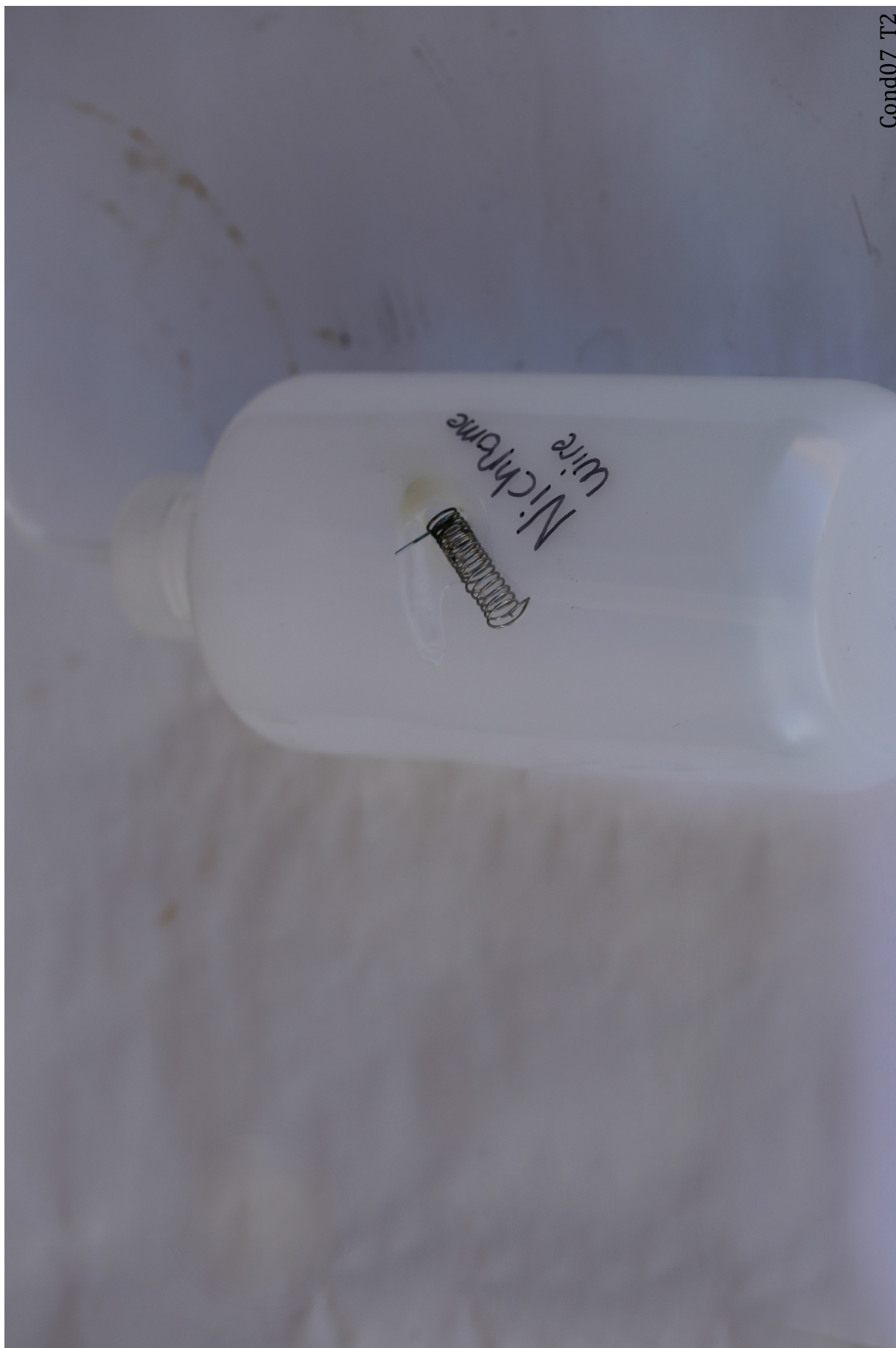
Figure 154: Condition 07 Trial 3. The empty polypropylene bottle melted slightly where in contact with the igniter.
