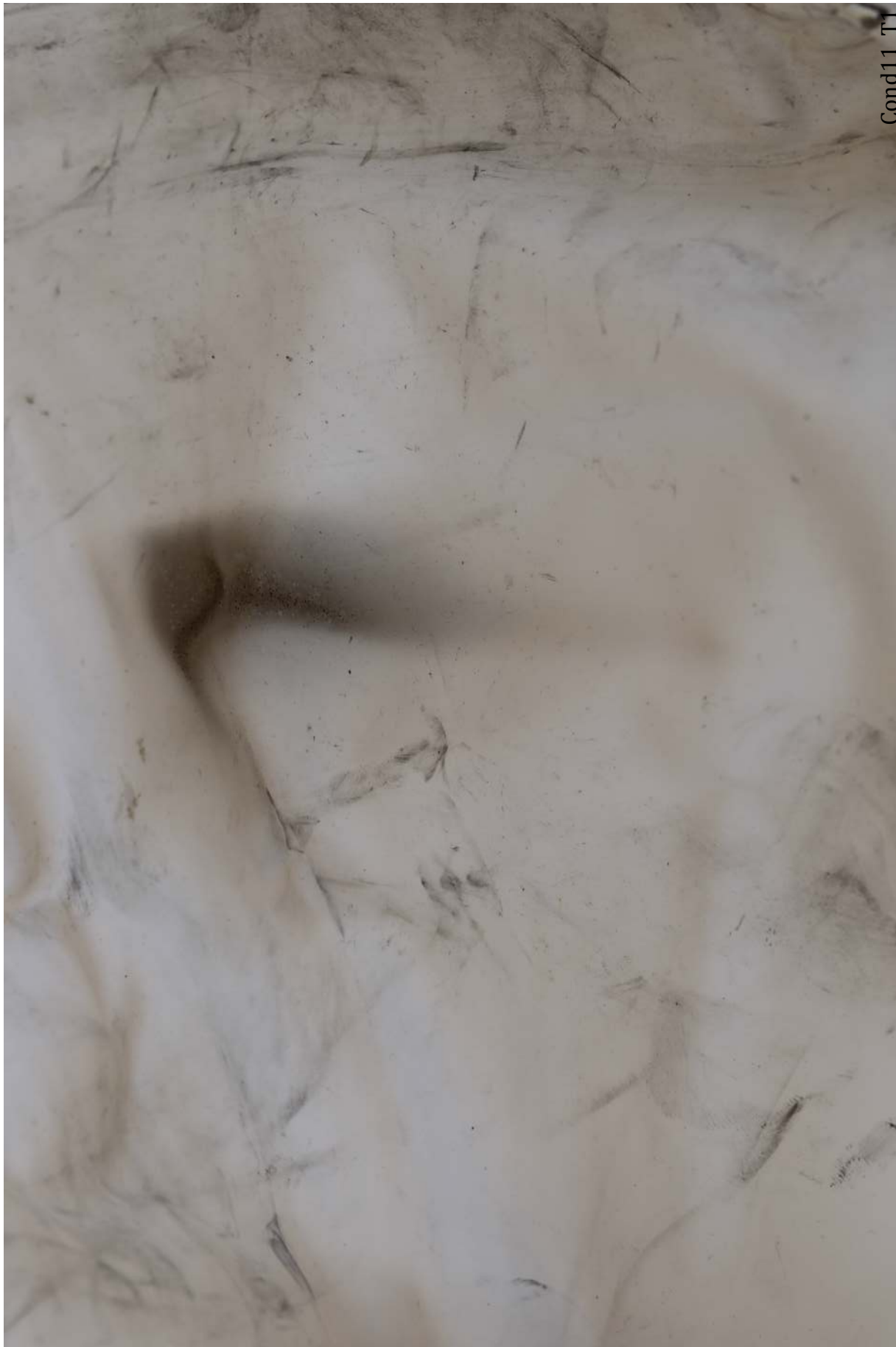
Figure 195: Condition 11 Trial 1. The port 10 glove sustained slight damage.
