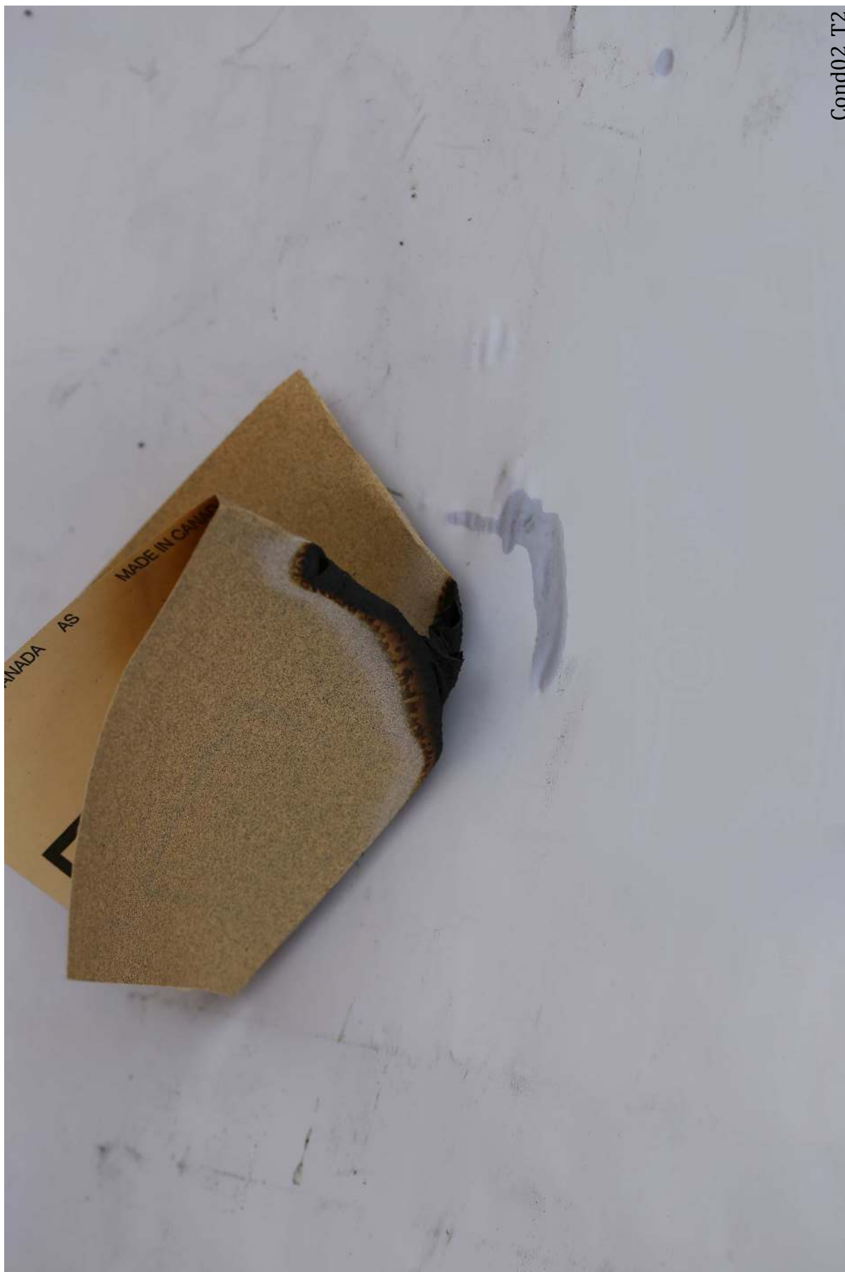
Figure 85: Condition 02 Trial 2. Minor charring is apparent on the edge of the sandpaper.
