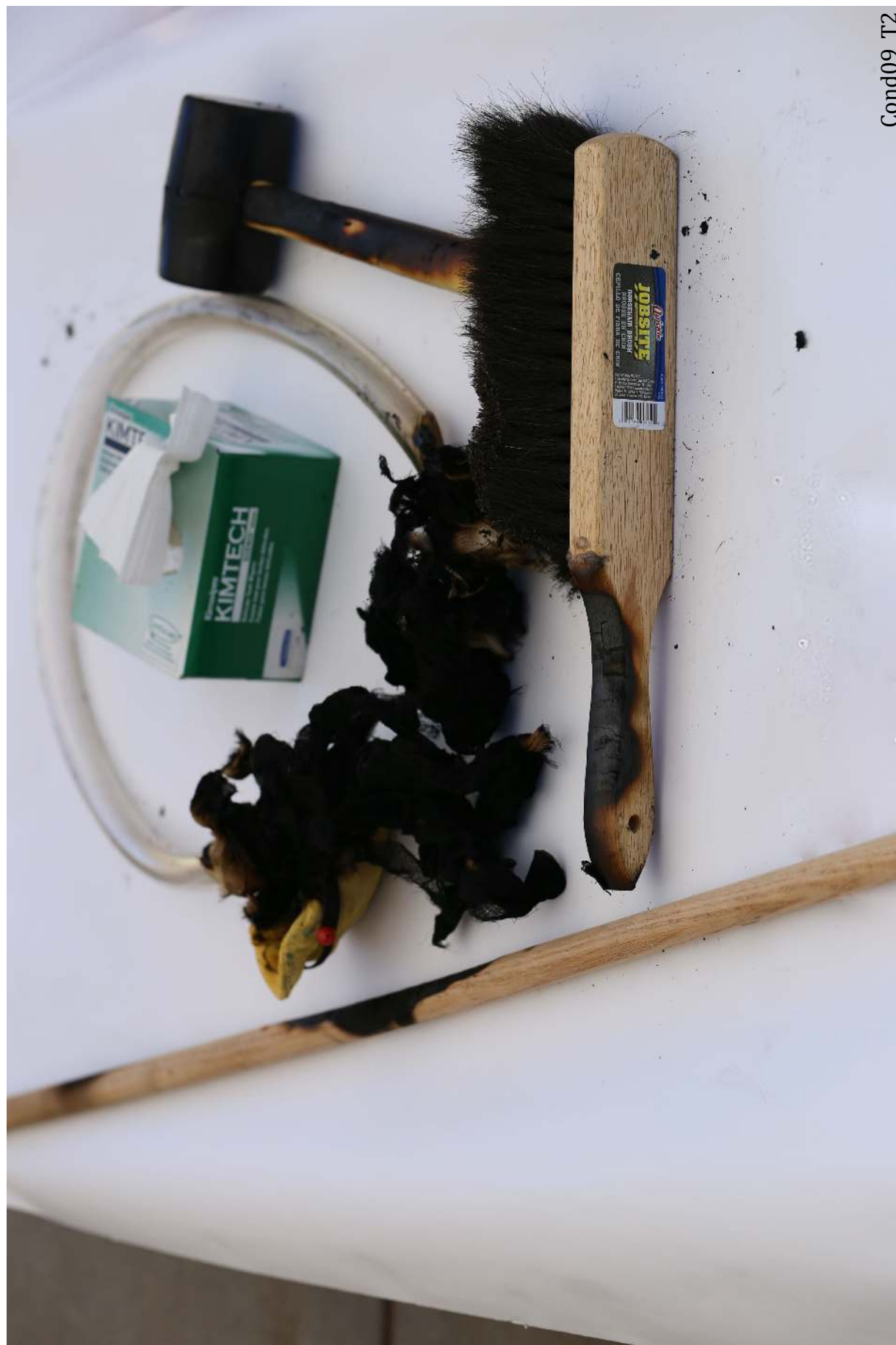
Figure 175: Condition 09 Trial 2. The horsehair brush, mallet handle, Tygon tubing, leather gloves, and task wipes were consumed in the fire.
