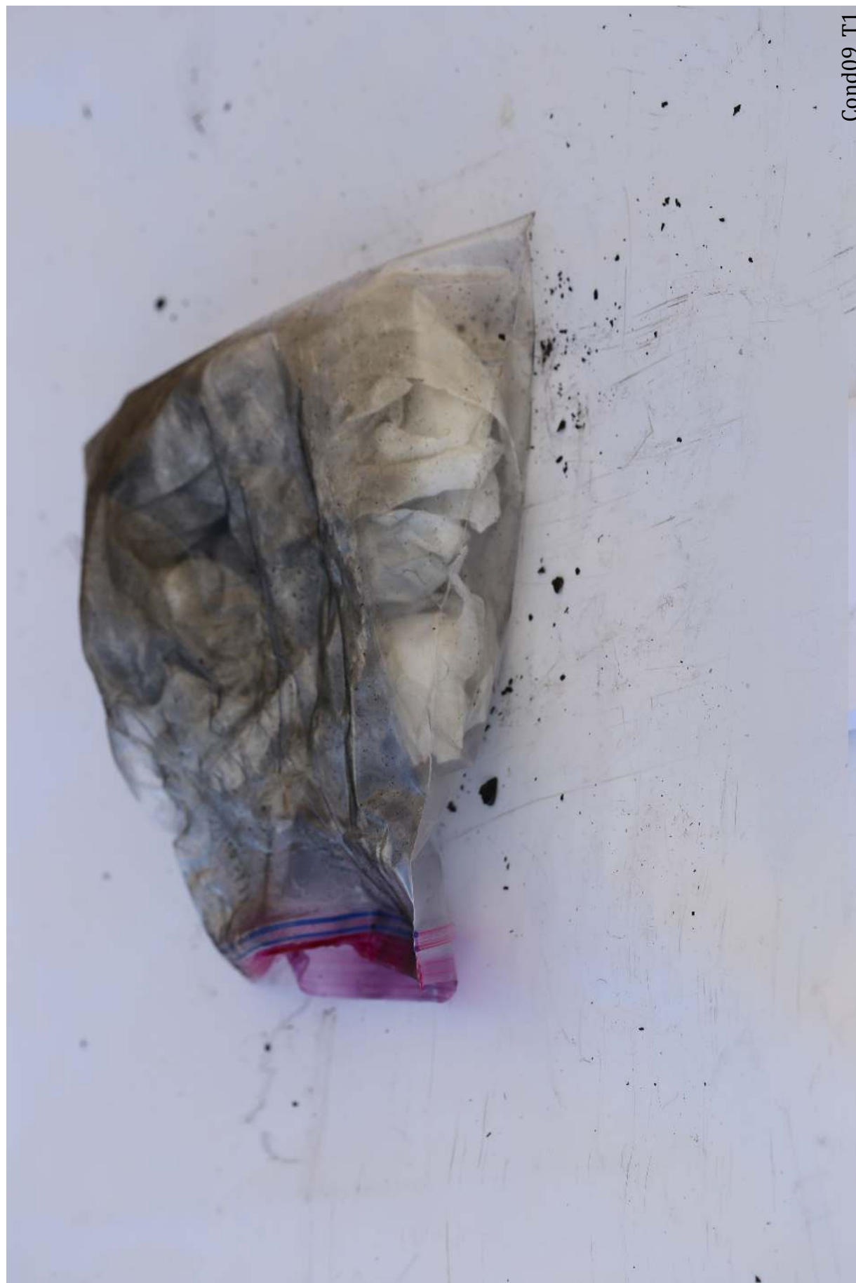
Figure 169: Condition 09 Trial 1. A bag of used cheesecloth was blackened slightly but the cheesecloth did not ignite.
