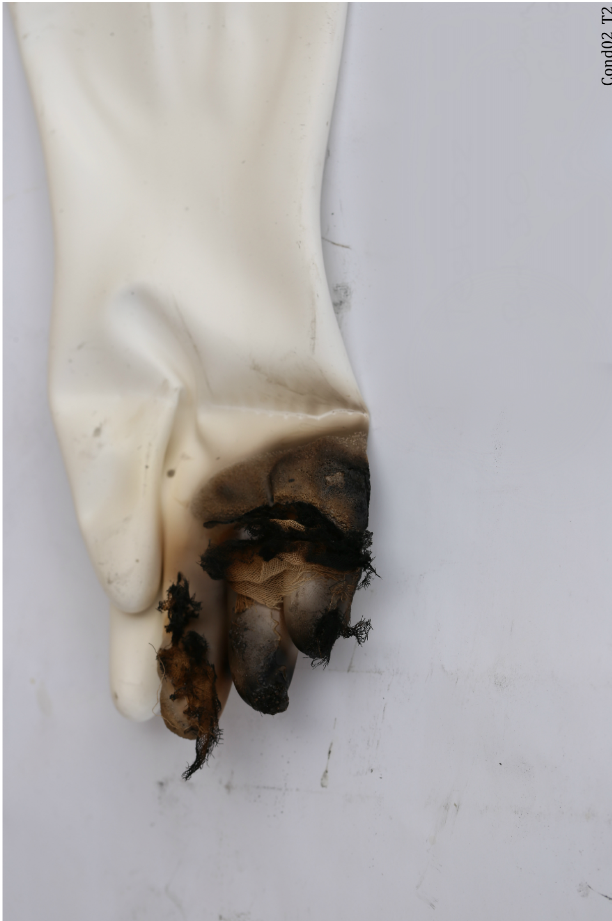
Figure 87: Condition 02 Trial 2. Charring occurred on the fingers of the port 30 glove. Burnt cheesecloth is melted to the fingers.
