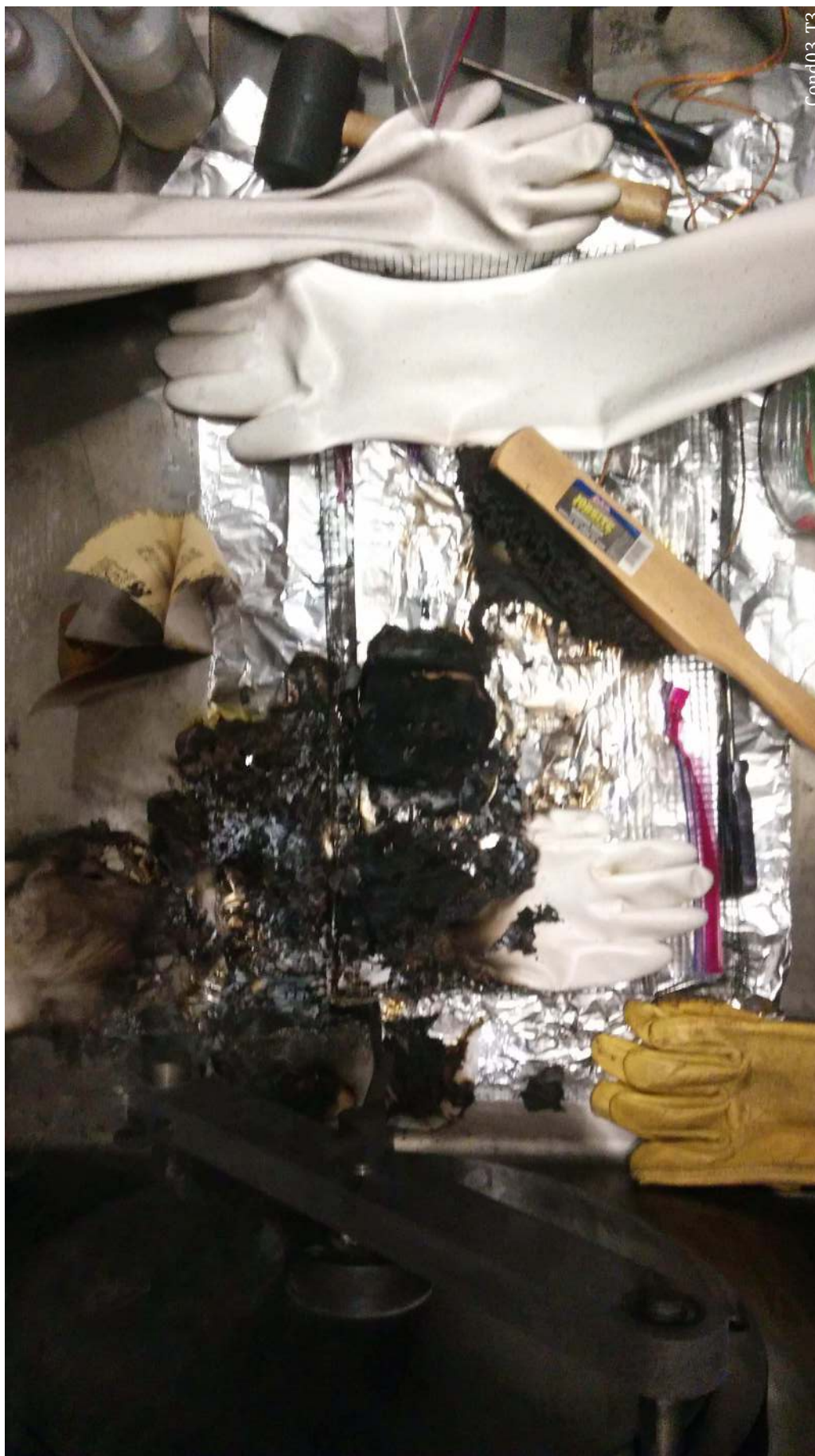
Figure 106: Condition 03 Trial 3. An isolated fire led to significant damage of two gloves.
