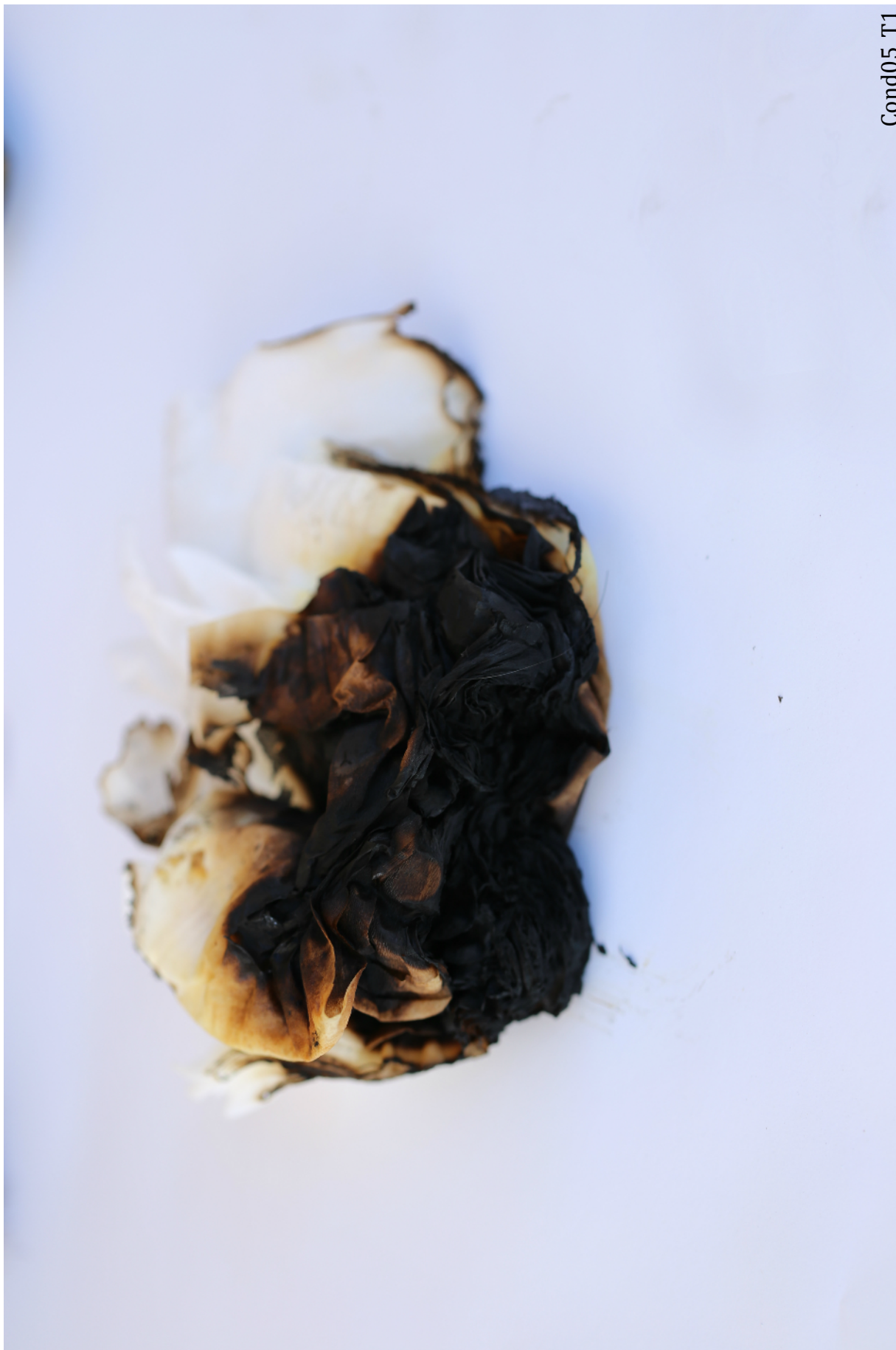
Figure 131: Condition 05 Trial 1. Crumpled task wipes burned.
