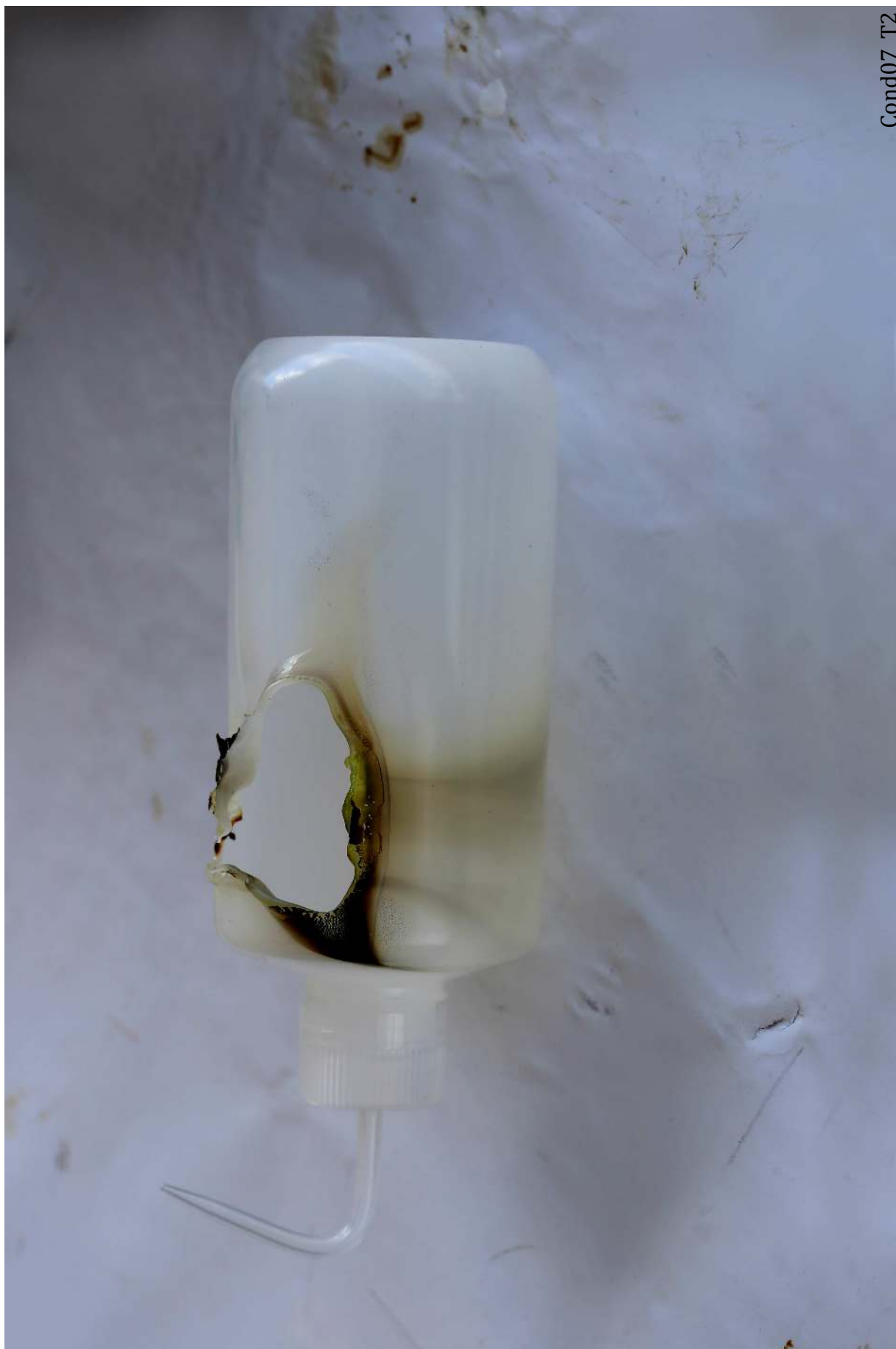
Figure 151: Condition 07 Trial 2. Igniters burned a large hole in the empty polypropylene bottle.
