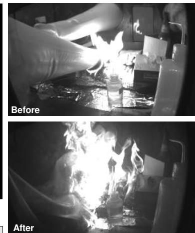
Figure 4. Fire before & after breach. External oxygen flow through the breach simultaneously strengthened the fire, leading to a more rapid consumption of the breached glove.
