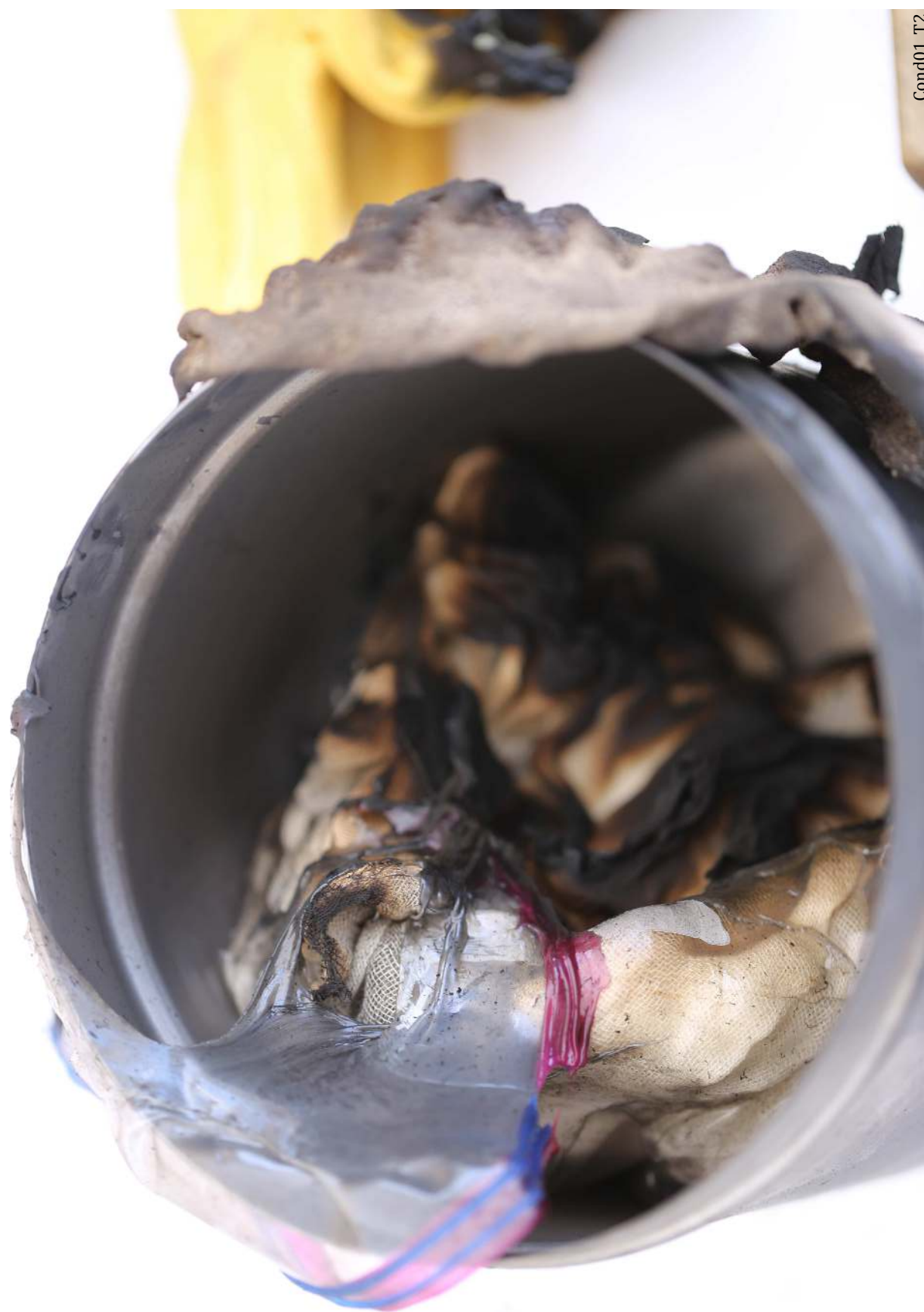
Figure 70: Condition 01 Trial 2. The open container did little to stop the cheesecloth inside from participating.
