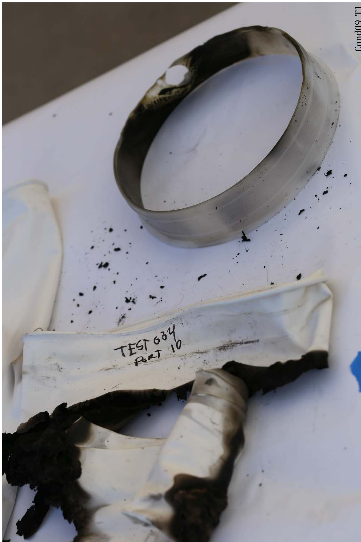
Figure 170: Condition 09 Trial 1. The port 10 glove (Inside port cover) burned severely.
