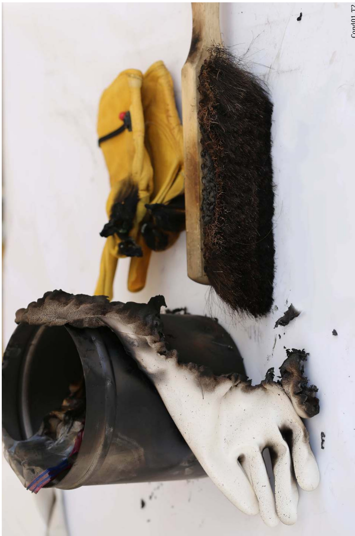
Figure 69: Condition 01 Trial 2. Burning of cheesecloth in the open container, the horsehair brush, and leather gloves led to a large breach in a glove.
