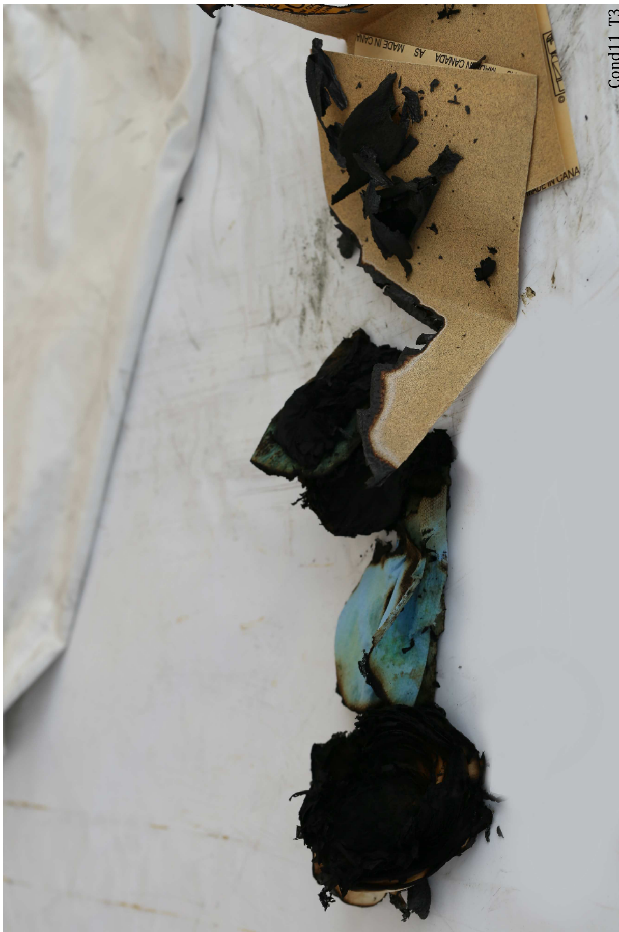
Figure 199: Condition 11 Trial 3. Sandpaper, task wipes, and a shop towel were burned.
