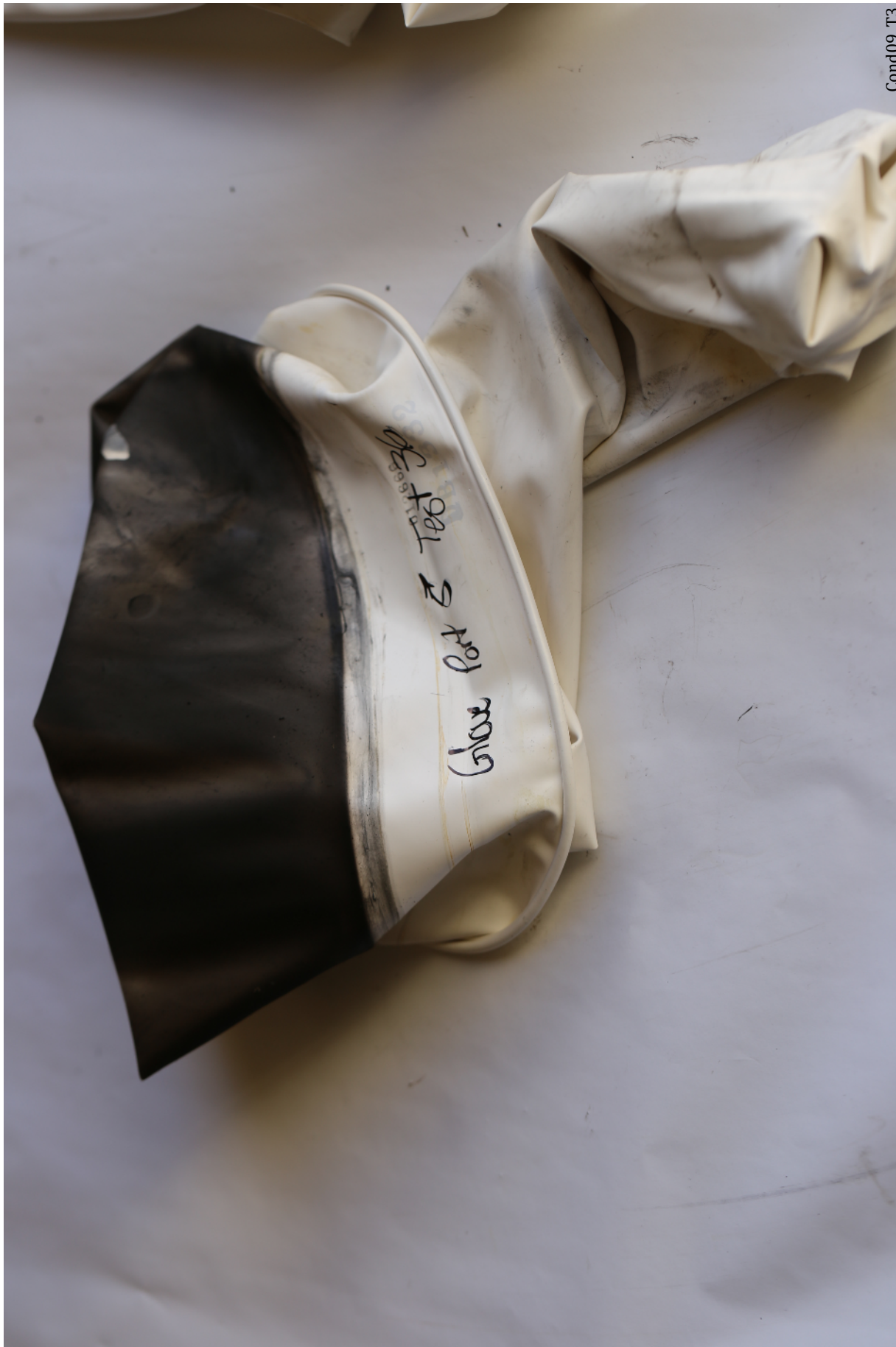
Figure 188: Condition 09 Trial 3. The port 5 glove was blackened and sustained a possible small breach.
