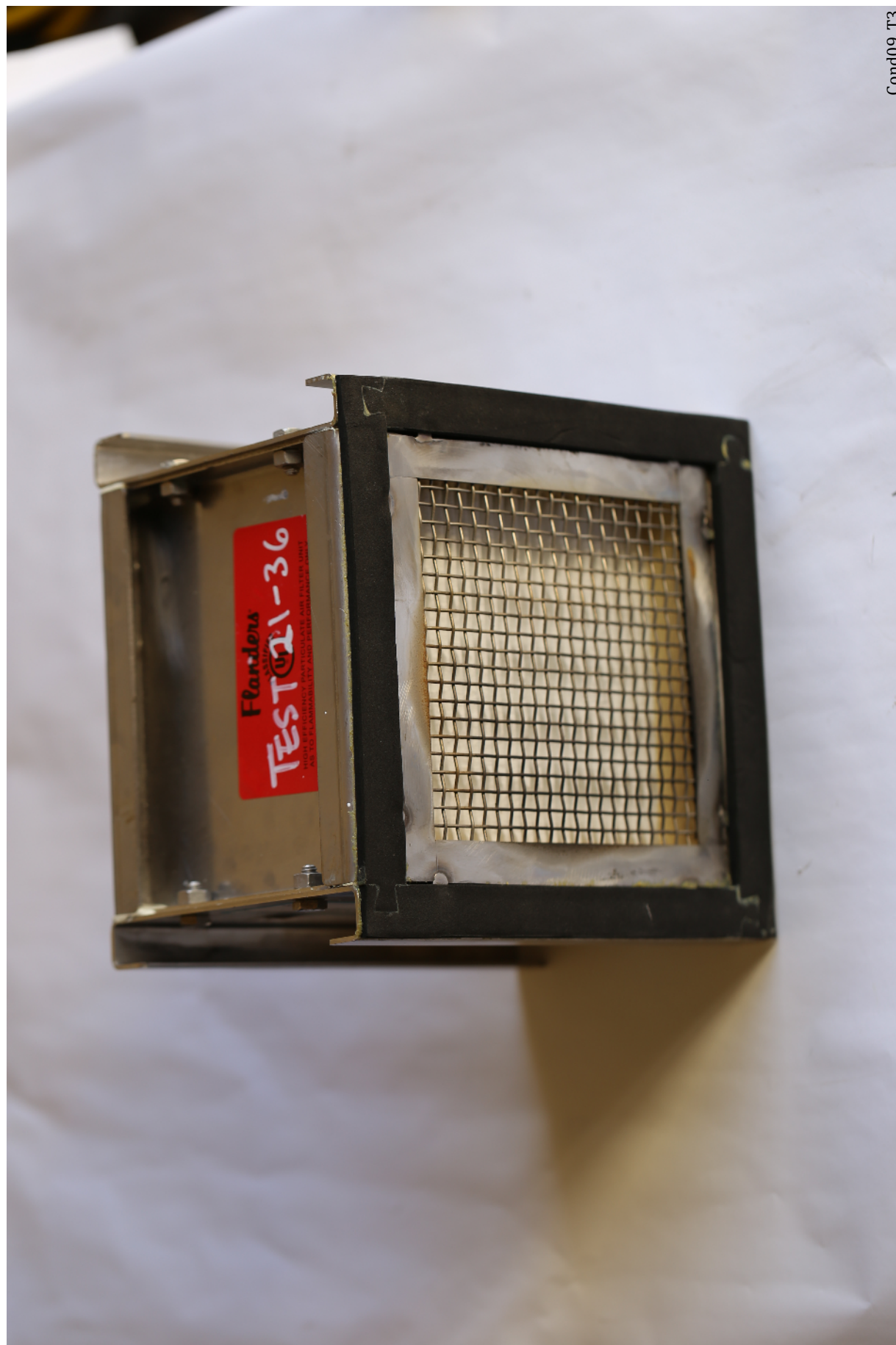
Figure 201: Inlet filters did not pack as quickly as exhaust; the same filter was often used for multiple consecutive trials.
