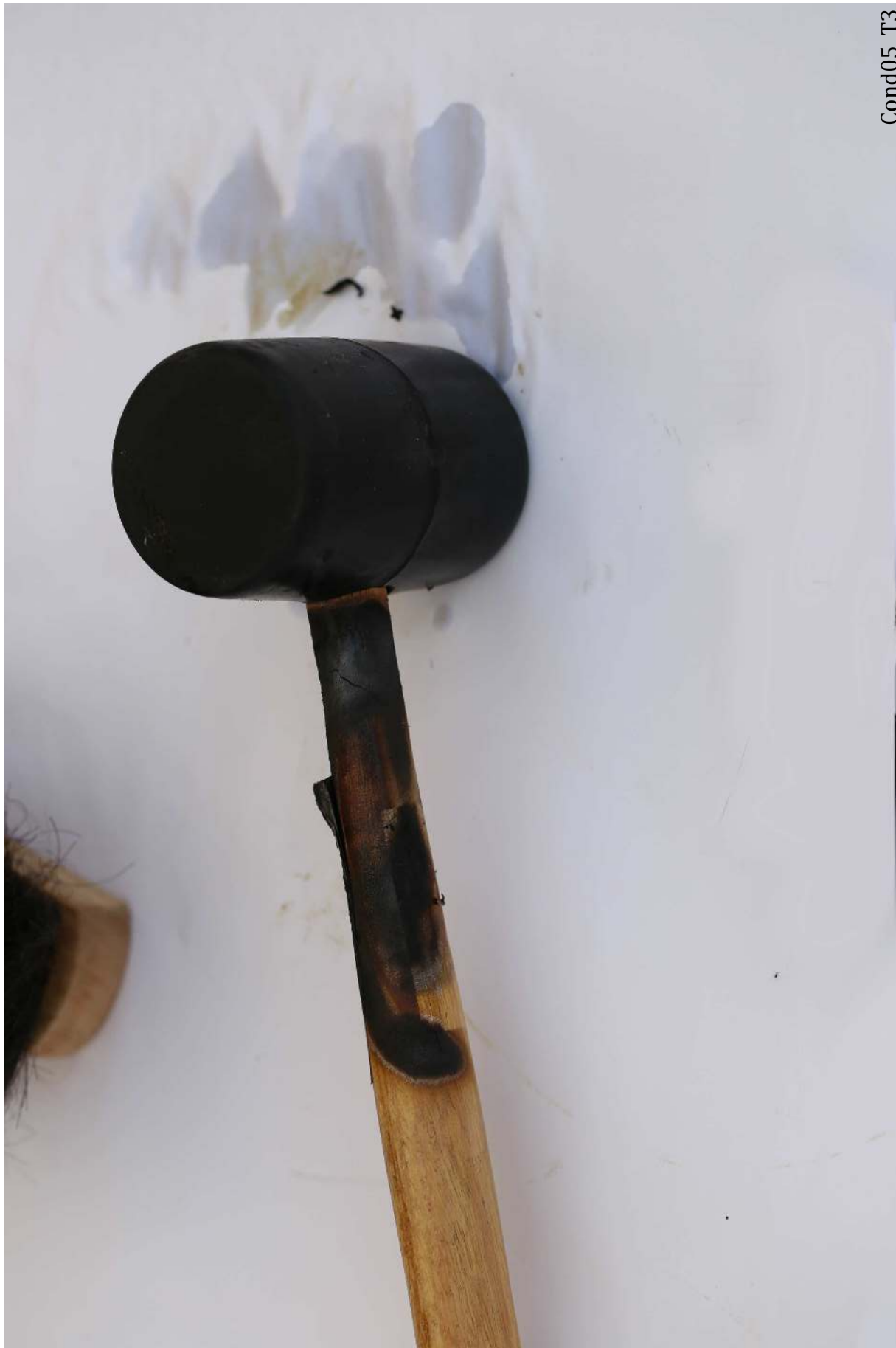
Figure 140: Condition 05 Trial 3. The handle of the mallet was burned.
