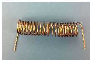
Figure 4: Ignitors were prepared from 22 AWG Nichrome wire.
