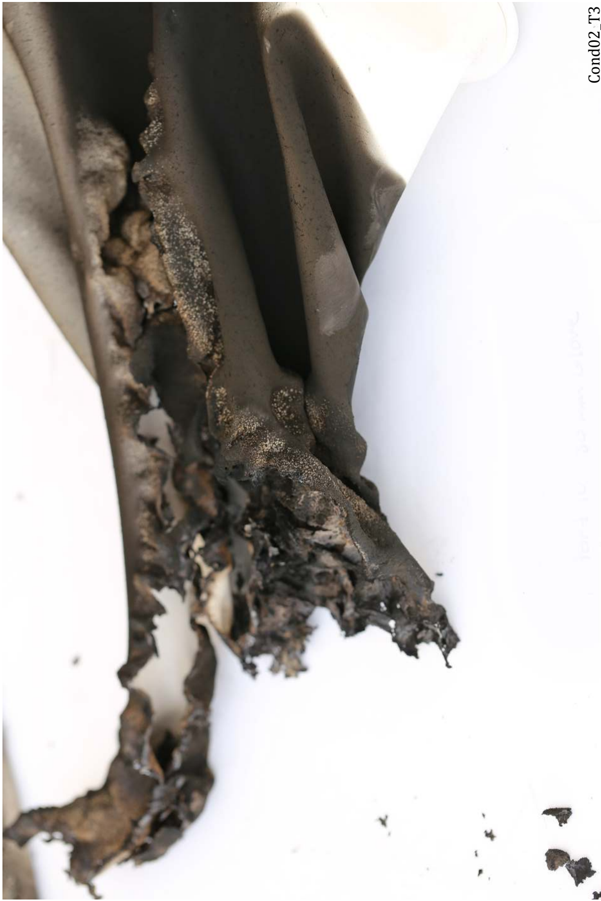
Figure 92: Condition 02 Trial 3. The hand and part of the sleeve on the port 10 glove were severely damaged.
