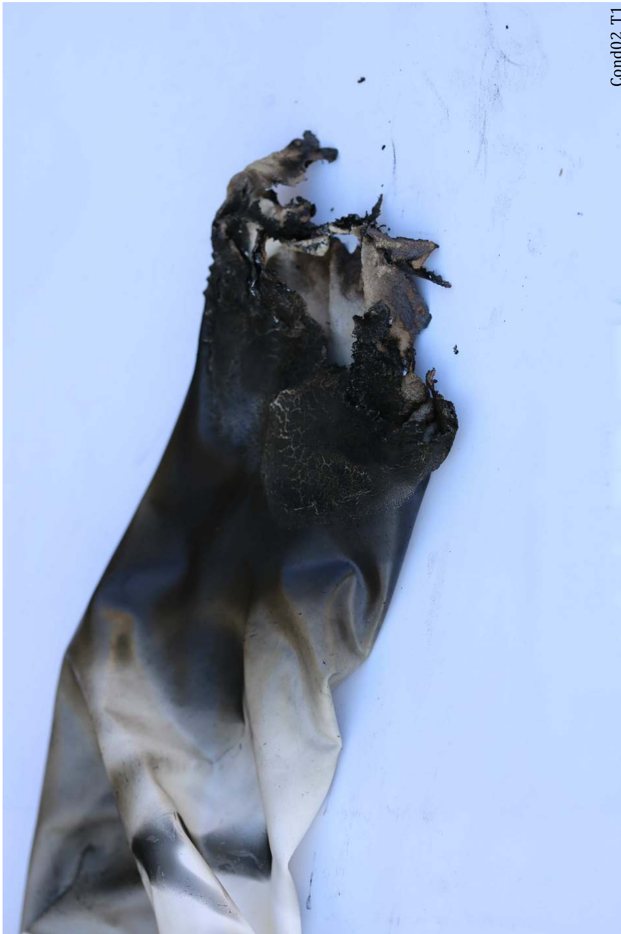
Figure 81: Condition 02 Trial 1. The hand on the port 24 glove completely deteriorated.
