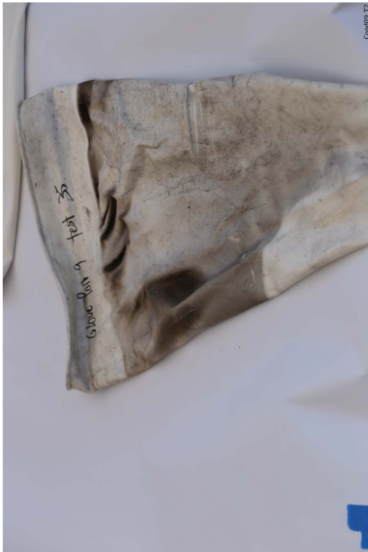
Figure 178: Condition 09 Trial 2. The port 9 glove exhibits bubbling near the ring.
