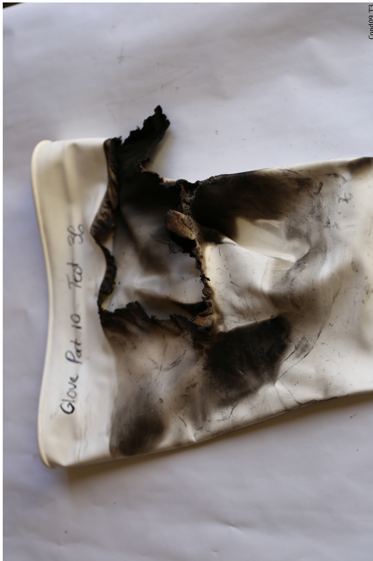
Figure 186: Condition 09 Trial 3. The port 10 glove sustained a substantial breach near the port ring.
