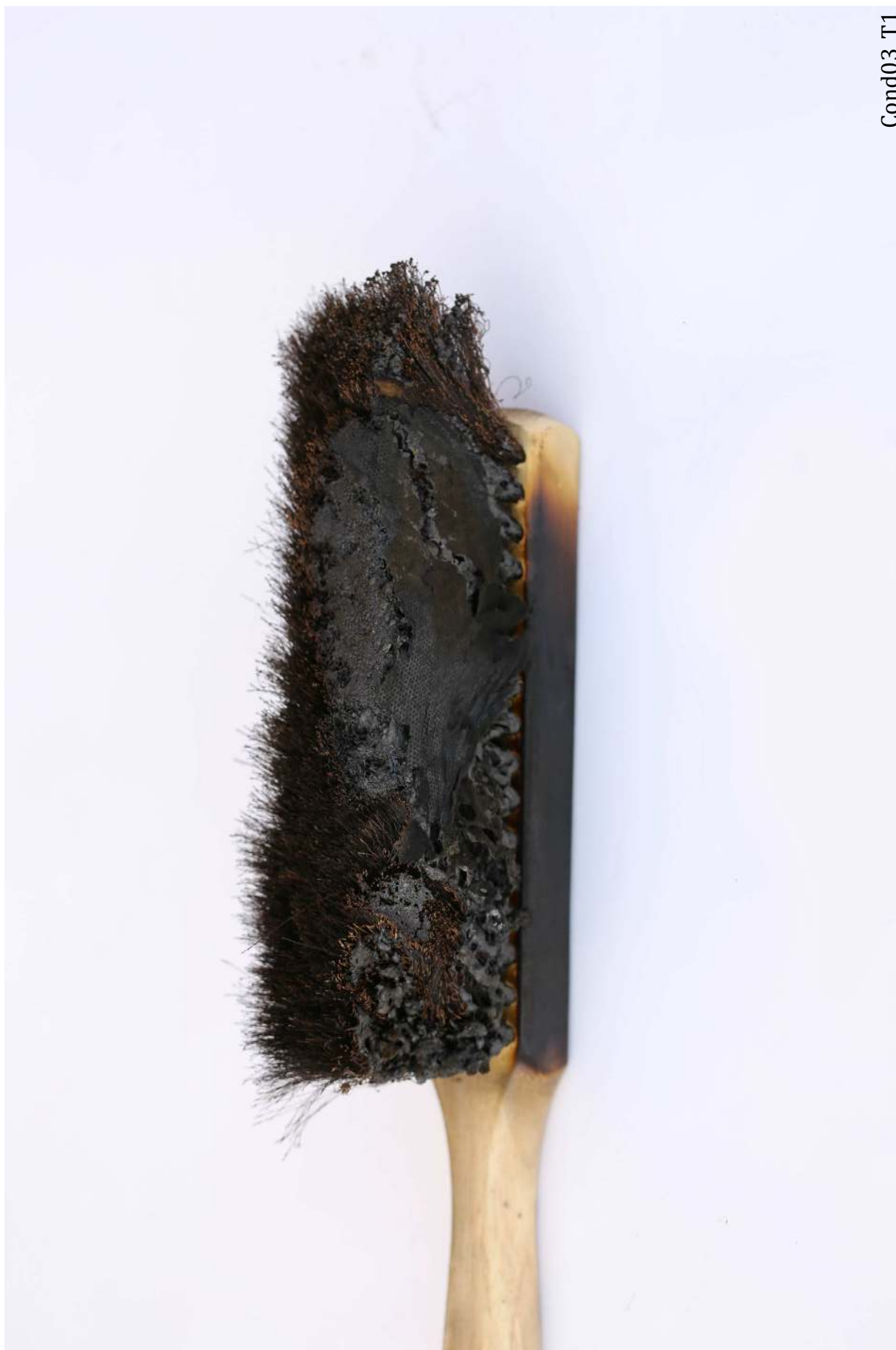
Figure 99: Condition 03 Trial 1. The horsehair brush was singed and the hair melted.
