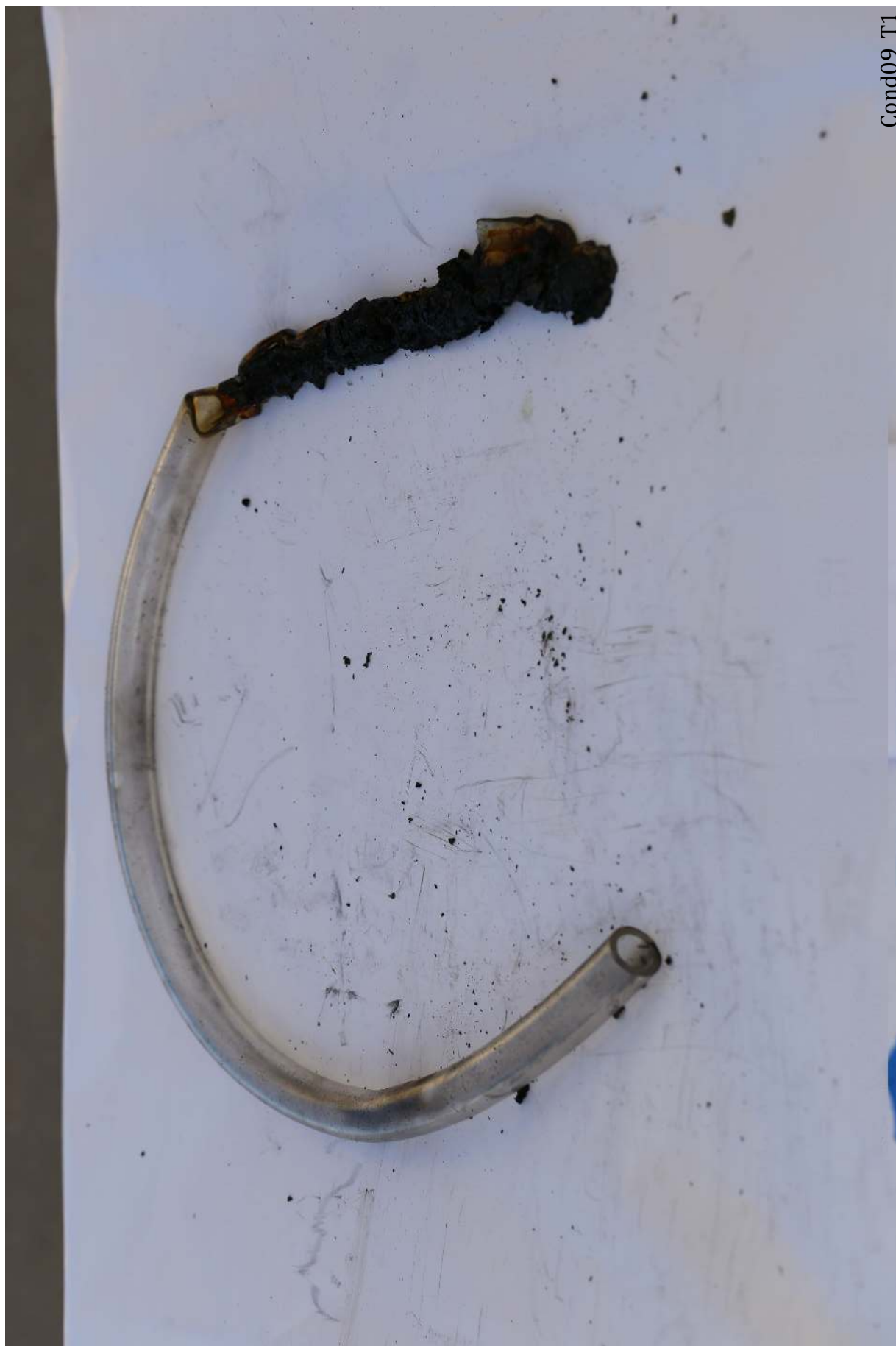
Figure 168: Condition 09 Trial 1. Fire burned and traveled along the Tygon tubing.
