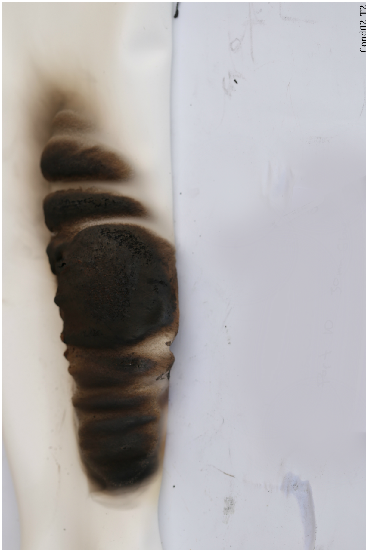
Figure 86: Condition 02 Trial 2. Bubbling and minor cracking occurred on the port 10 glove.
