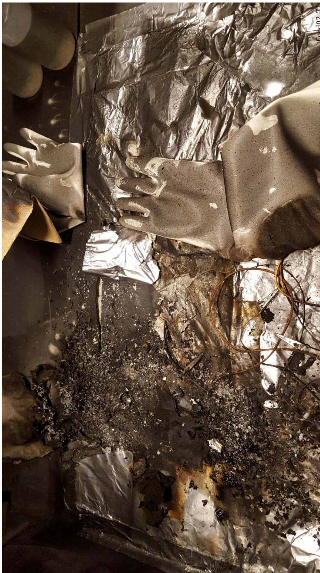
Figure 77: Condition 02 Trial 1. A robust fire was produced that severely damaged several gloves. (Burnt consumables were removed before photo)
