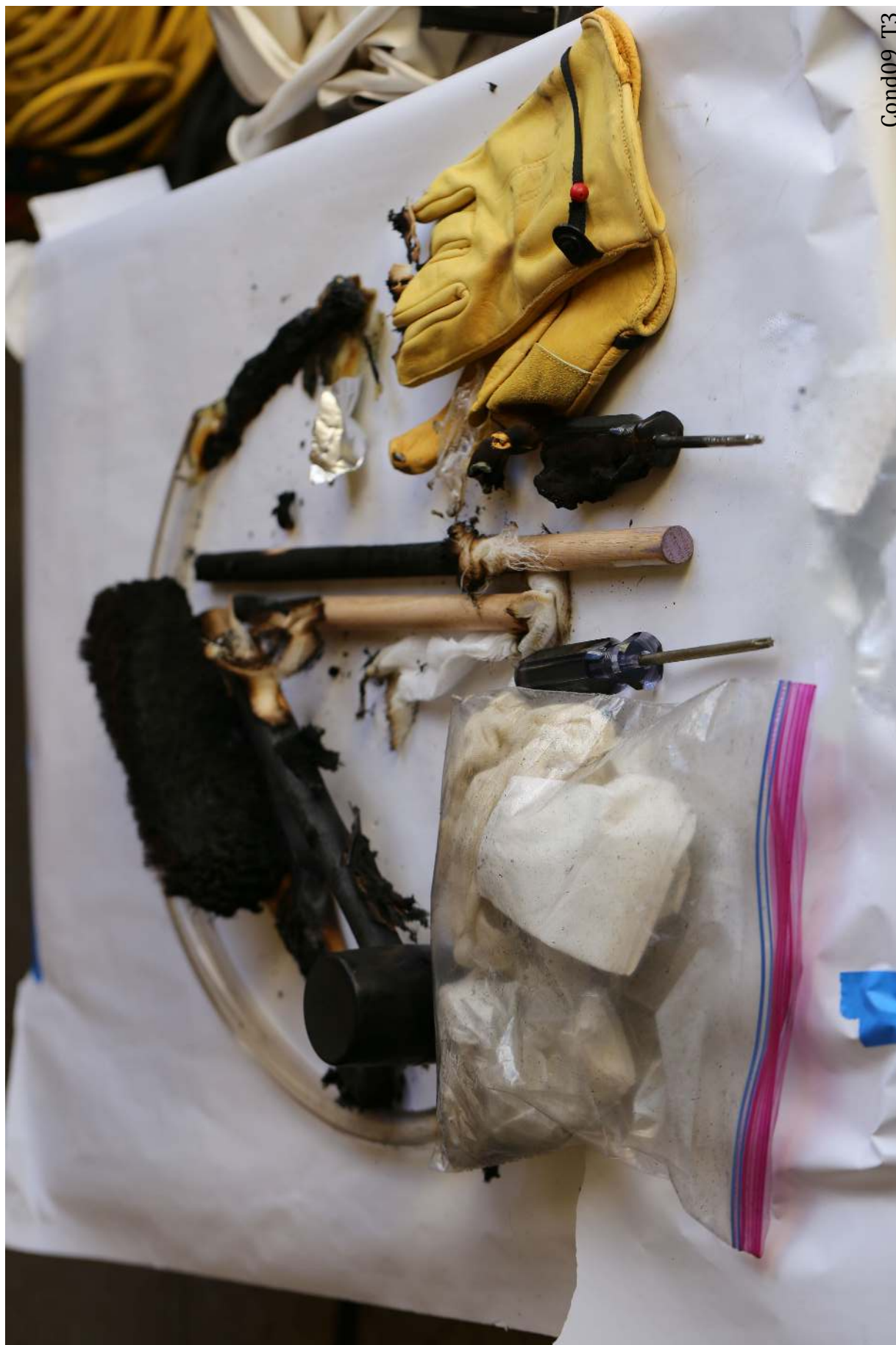
Figure 183: Condition 09 Trial 3. The horsehair brush, mallet, dowel, and leather gloves were burned.
