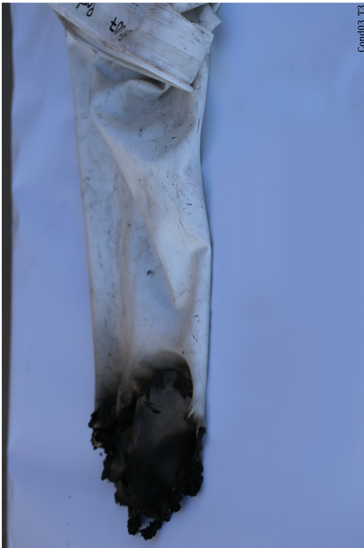
Figure 111: Condition 03 Trial 3. Condition 01 Trial 1. The fingers on the port 9 glove were consumed.
