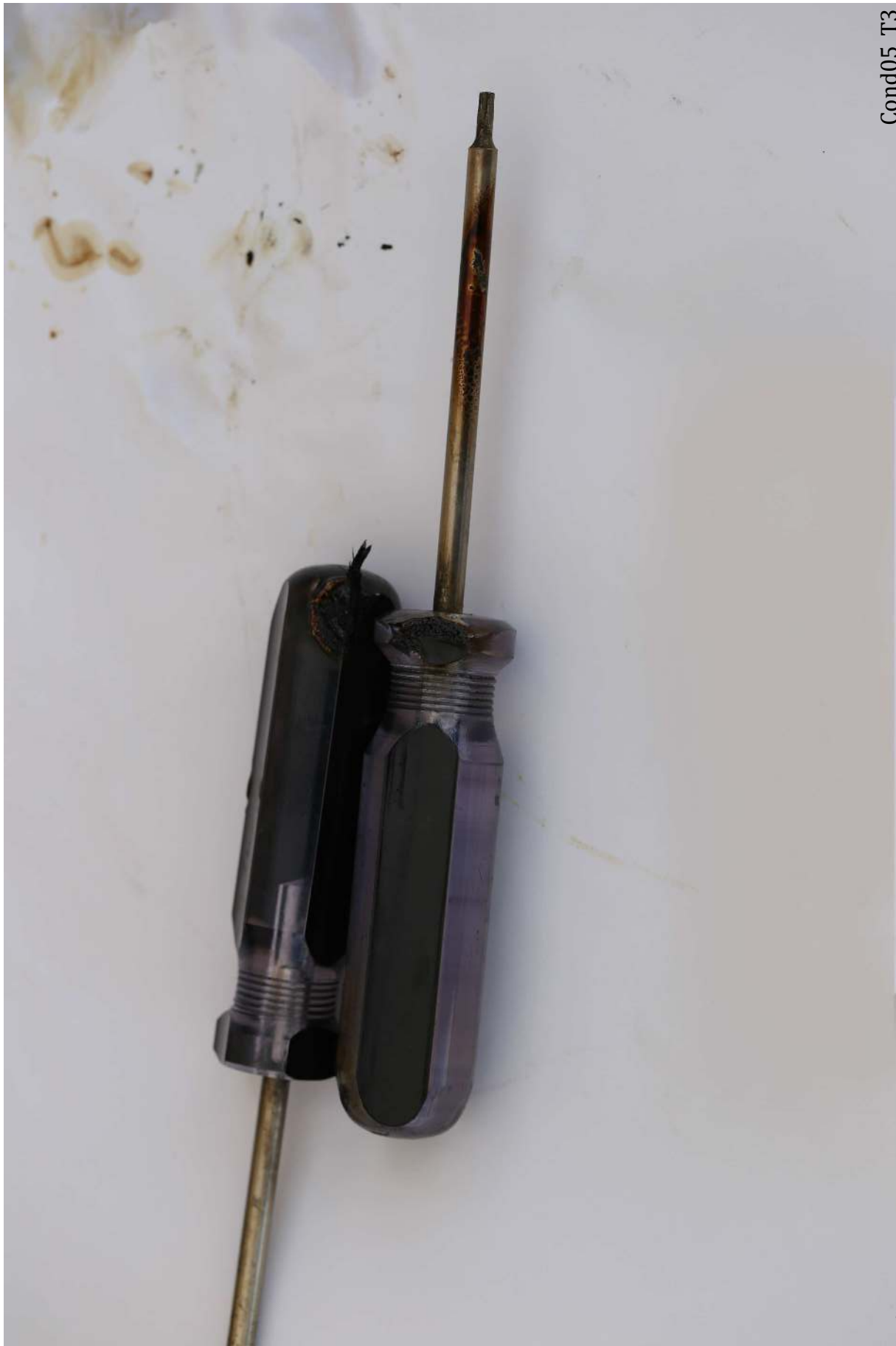
Figure 141: Condition 05 Trial 3. Screwdrivers were charred.
