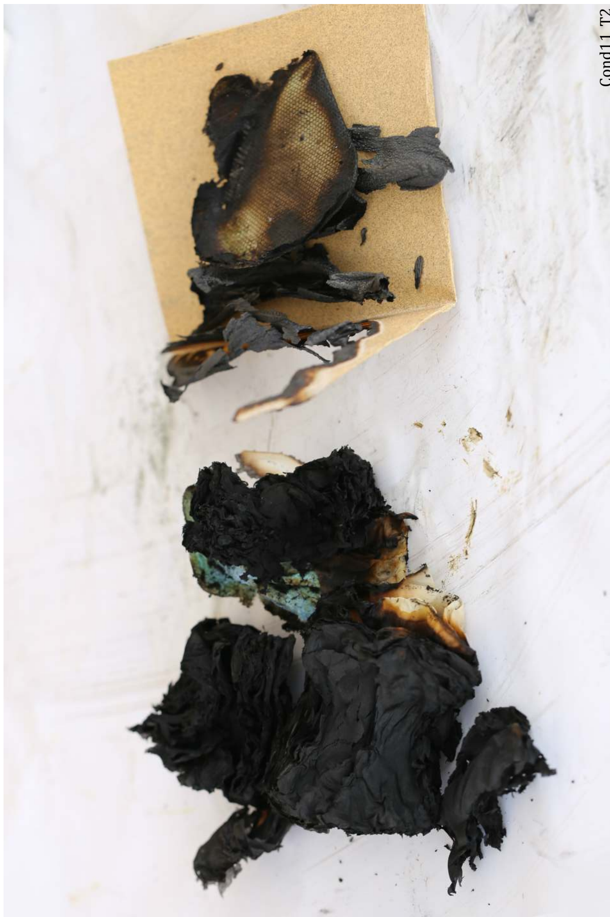
Figure 197: Condition 11 Trial 2. Sandpaper, task wipes, and a shop towel were burned.
