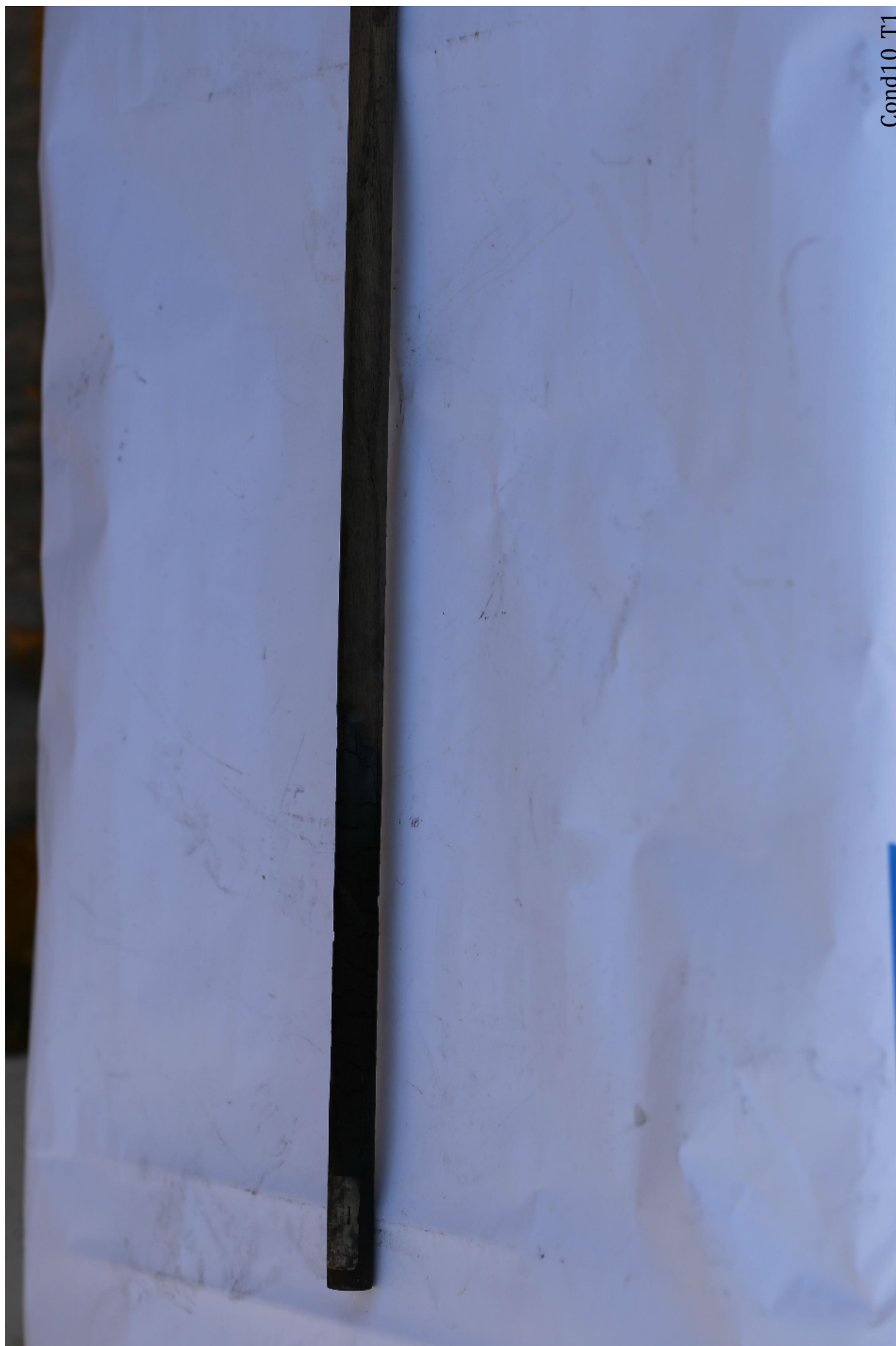
Figure 193: Condition 10 Trial 1. The wooden dowel caught fire and charred thoroughly.
