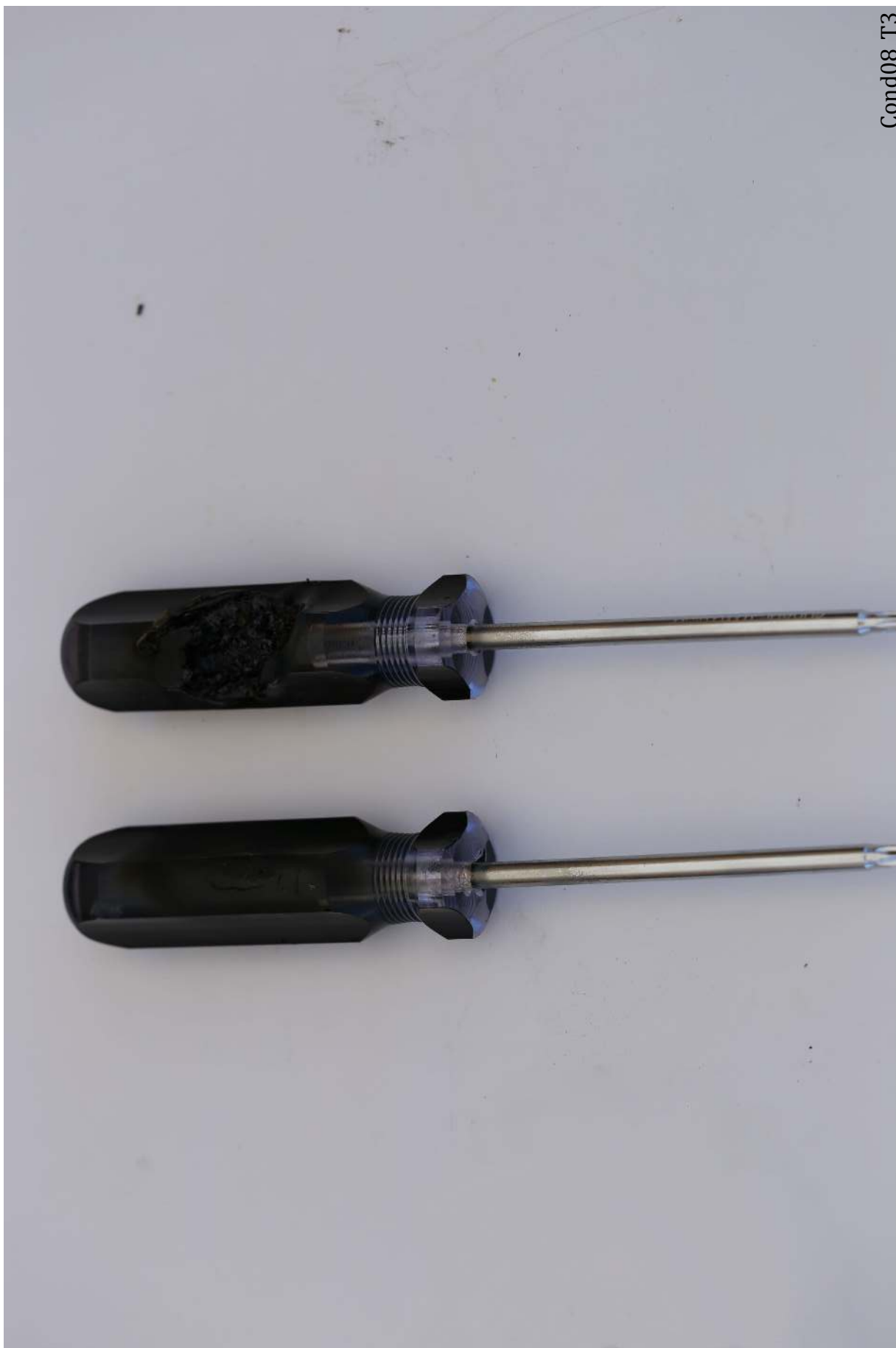
Figure 163: Condition 08 Trial 3. Screwdrivers were charred and melted where they contacted with igniters.
