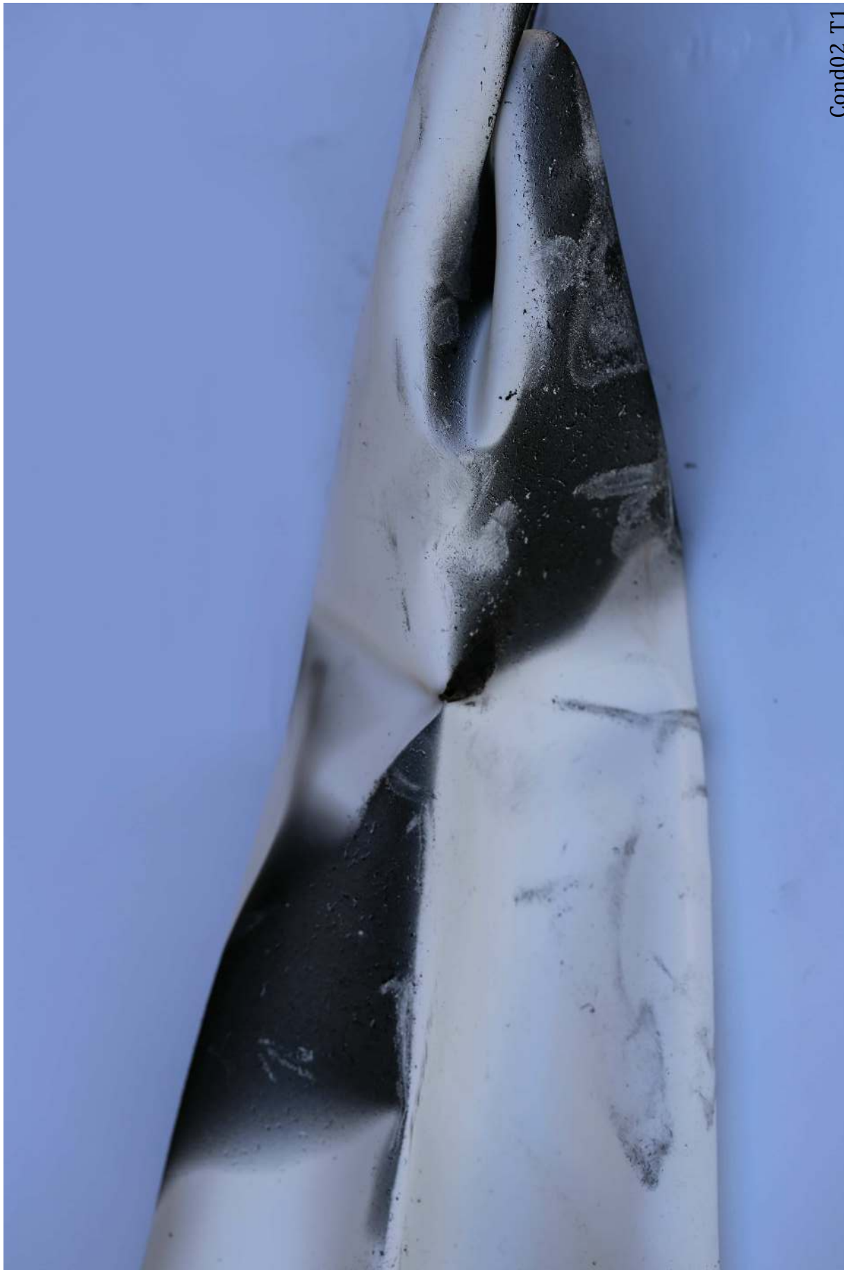
Figure 80: Condition 02 Trial 1. Charring is apparent on the port 23 glove
