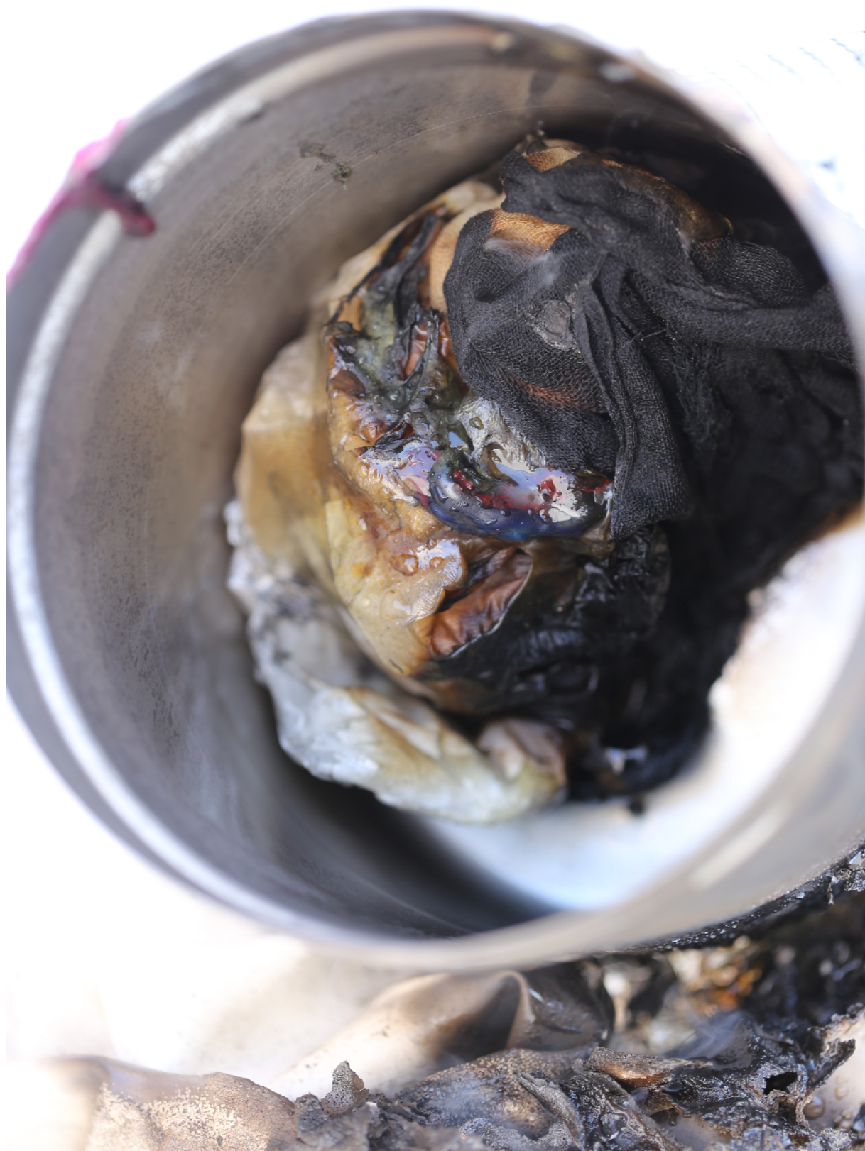
Figure 65: Condition 01 Trial 1. With the lid off, the fire resistant container did little to protect its contents from fire.
