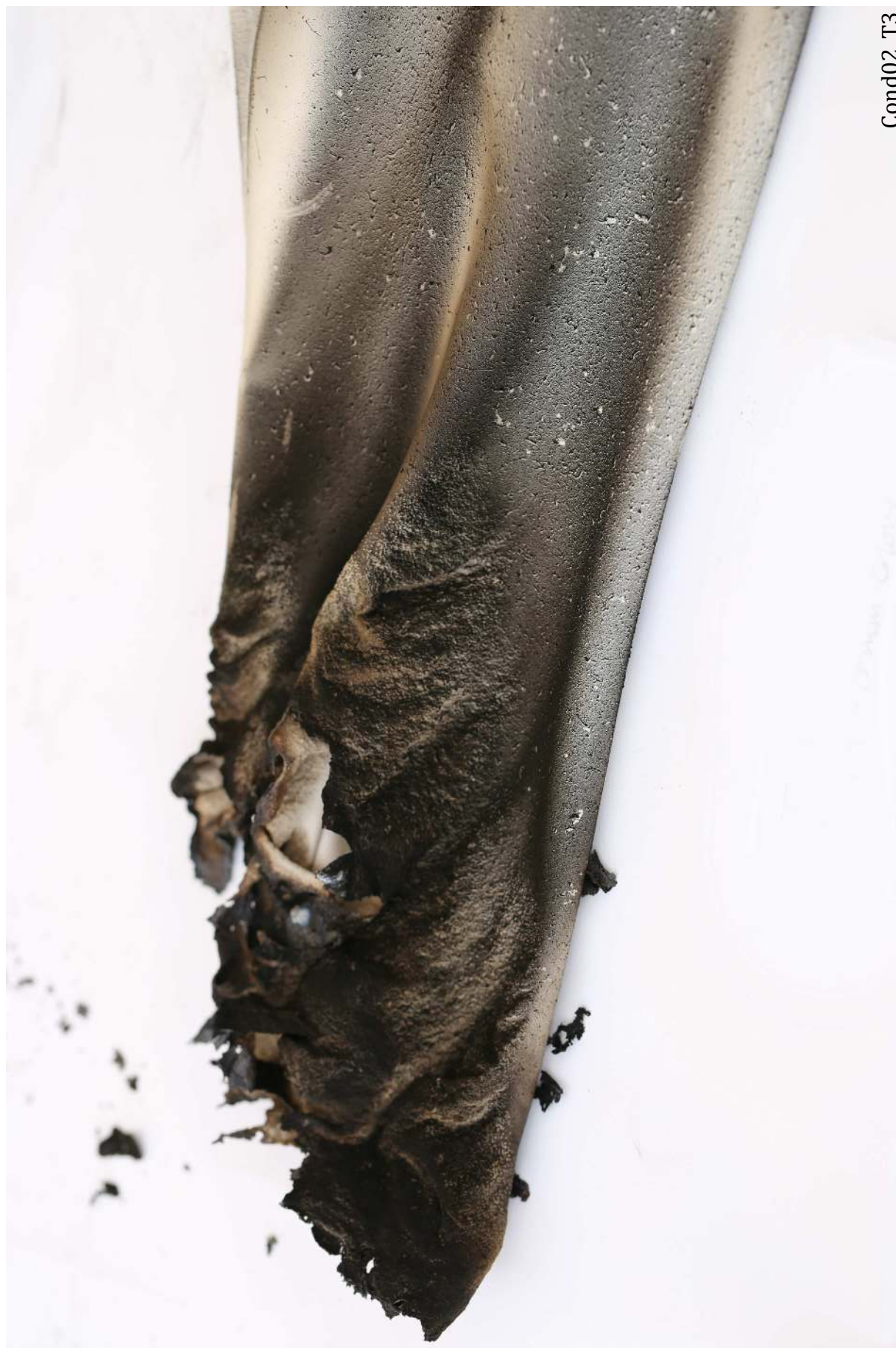
Figure 91: Condition 02 Trial 3. The fingers on the port 9 glove were consumed.
