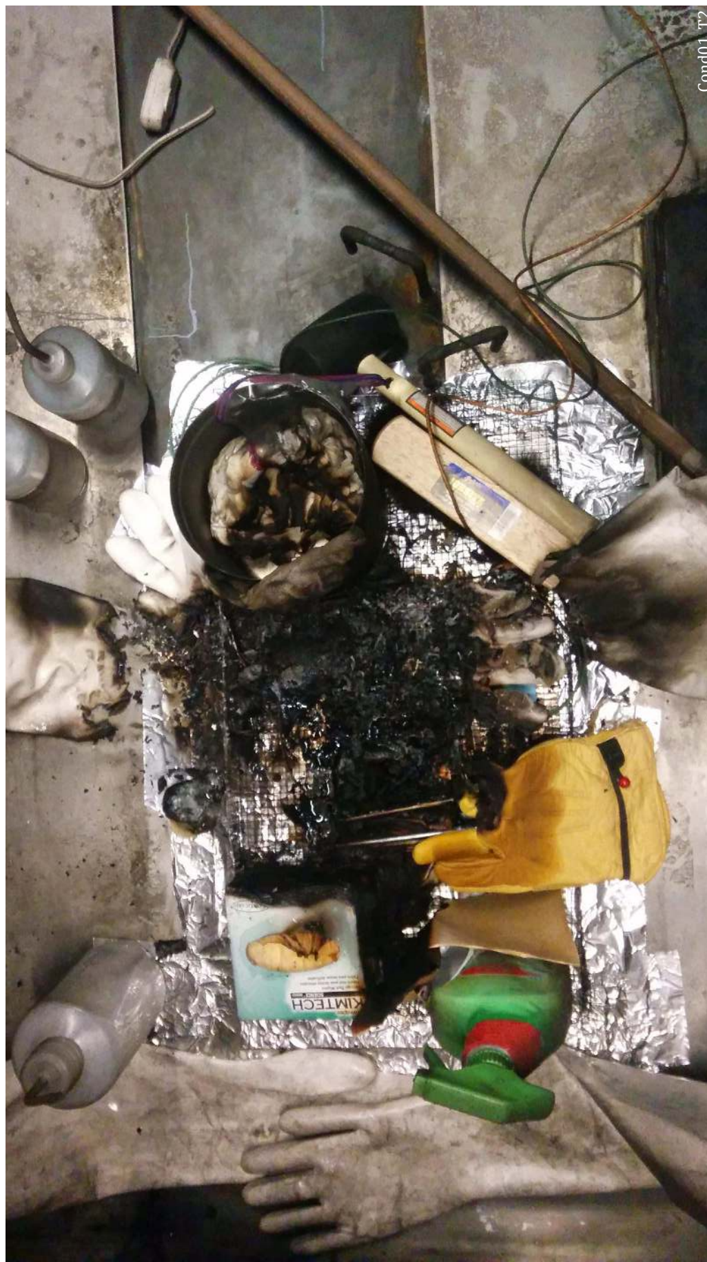
Figure 67: Condition 01 Trial 2. A robust fire burned several gloves and consumables, including cheesecloth in the fire resistant container.
