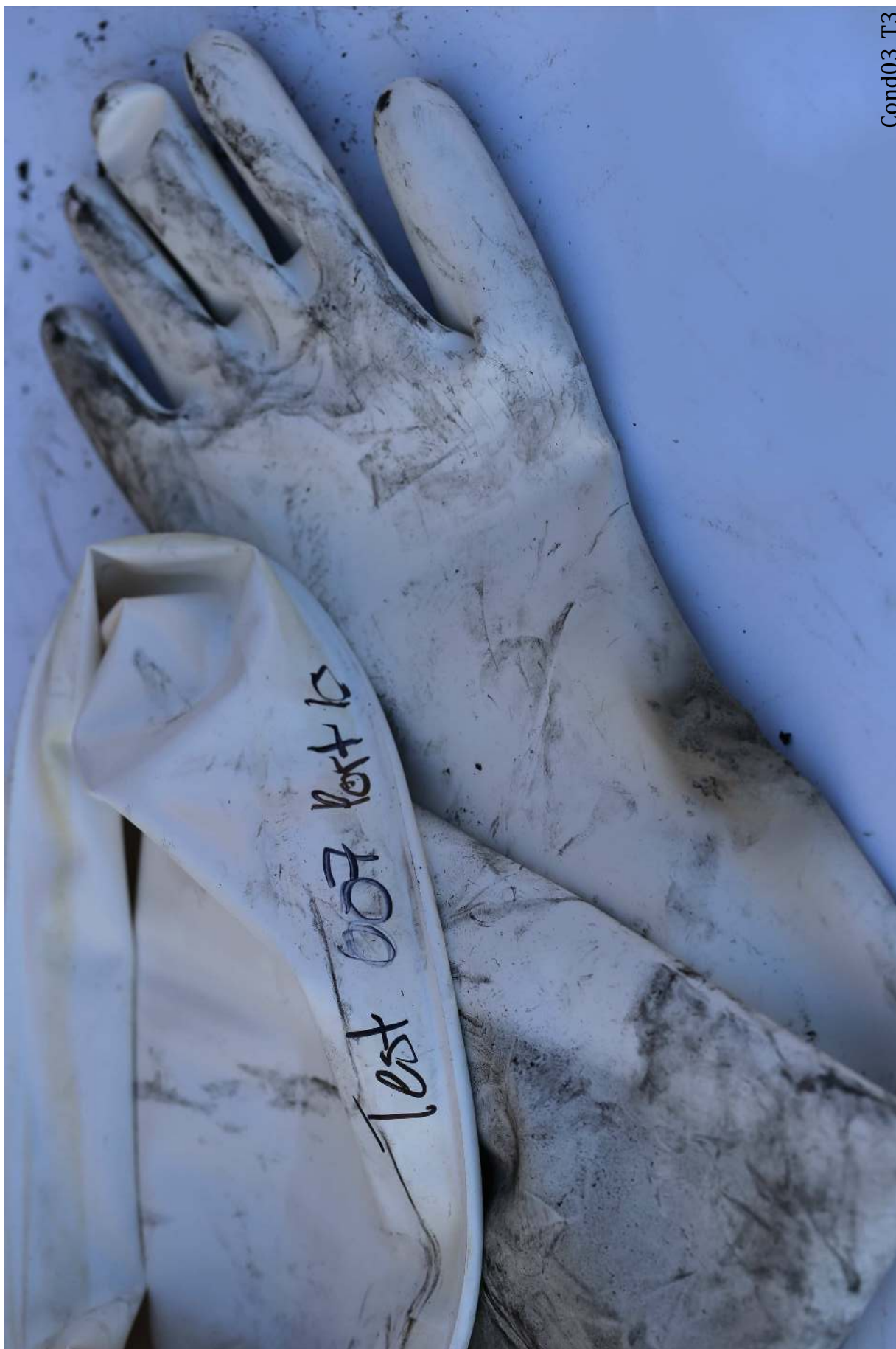
Figure 112: Condition 03 Trial 3. The wrist of the port 10 glove sustained minor damage.
