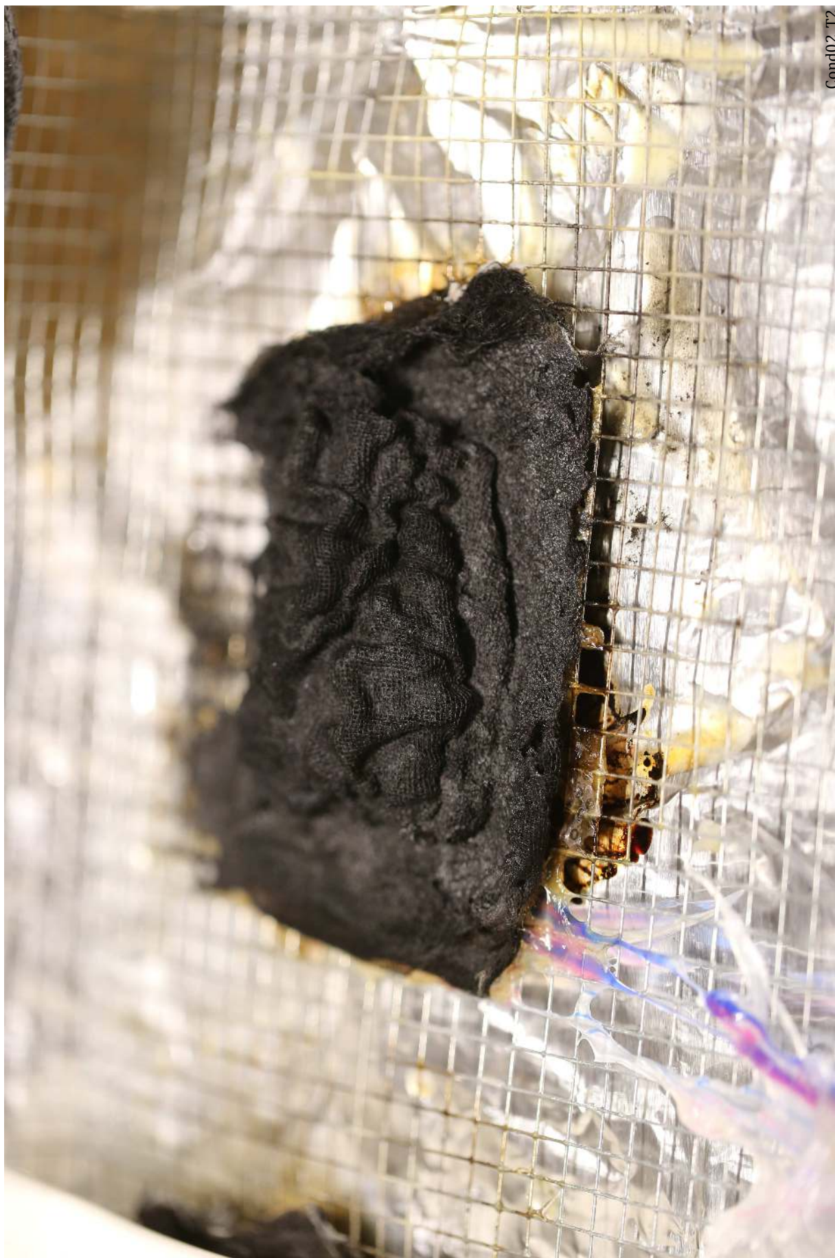
Figure 84: Condition 02 Trial 2. Cheesecloth was completely burned.
