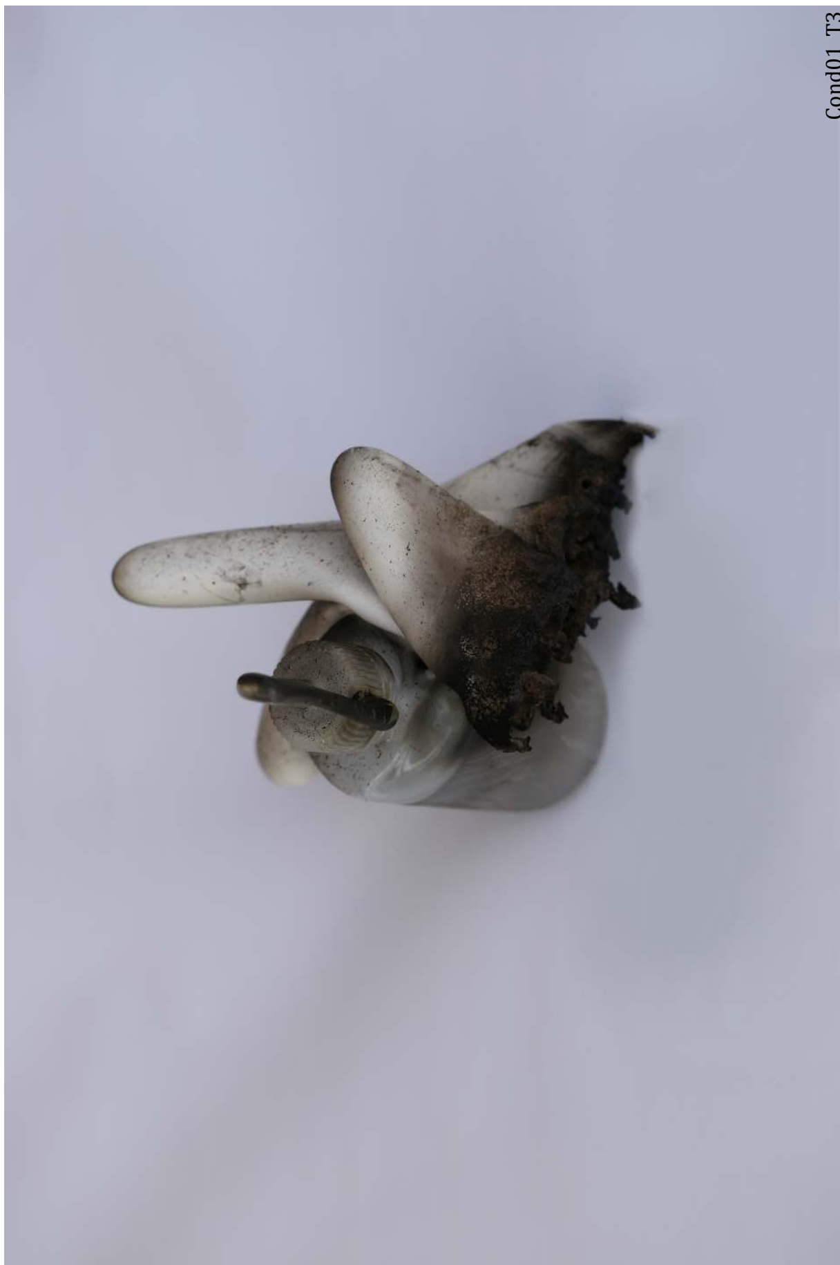
Figure 76: Condition 01 Trial 3. The fingers of the Port 10 Glove were detached and melted onto the alcohol bottle.
