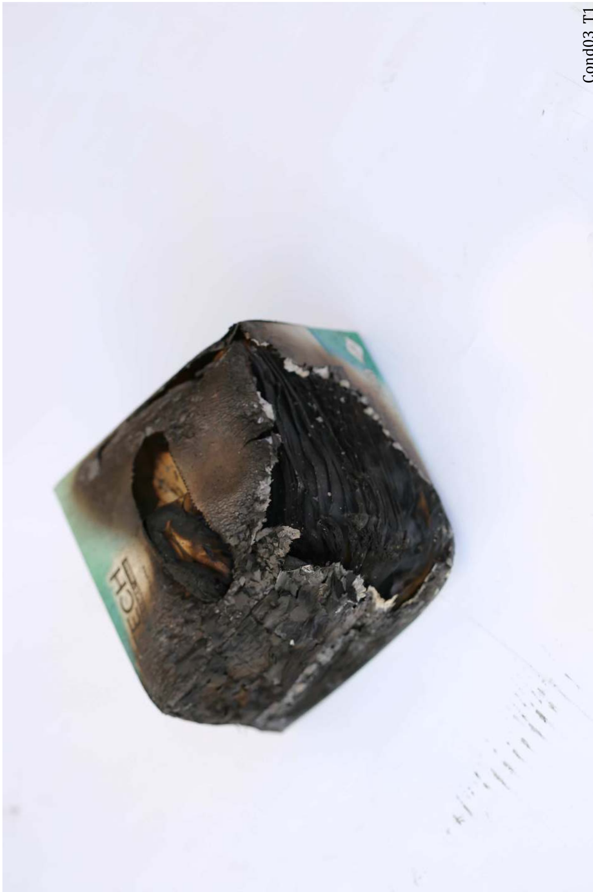
Figure 100: Condition 03 Trial 1. The box of task wipes was thoroughly burnt.
