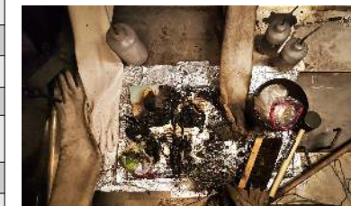
Figure 5. Typical state of GB contents after fire. Damage is localized and extent of combustion varies.
