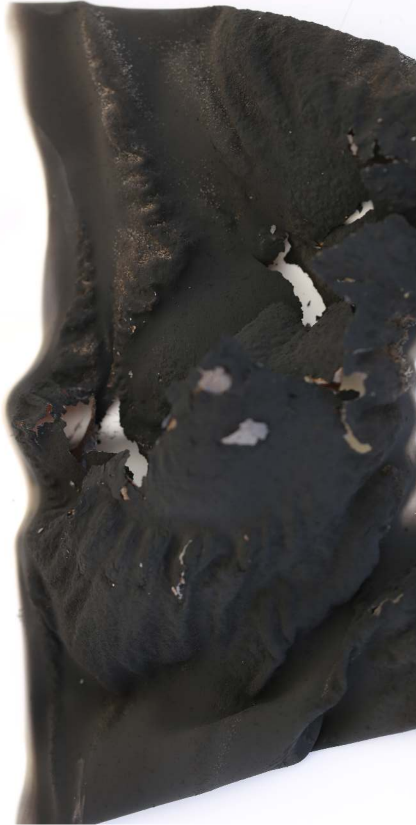
Figure 126: Condition 04 Trial 2. The port 9 glove was charred and cracked near the ring.
