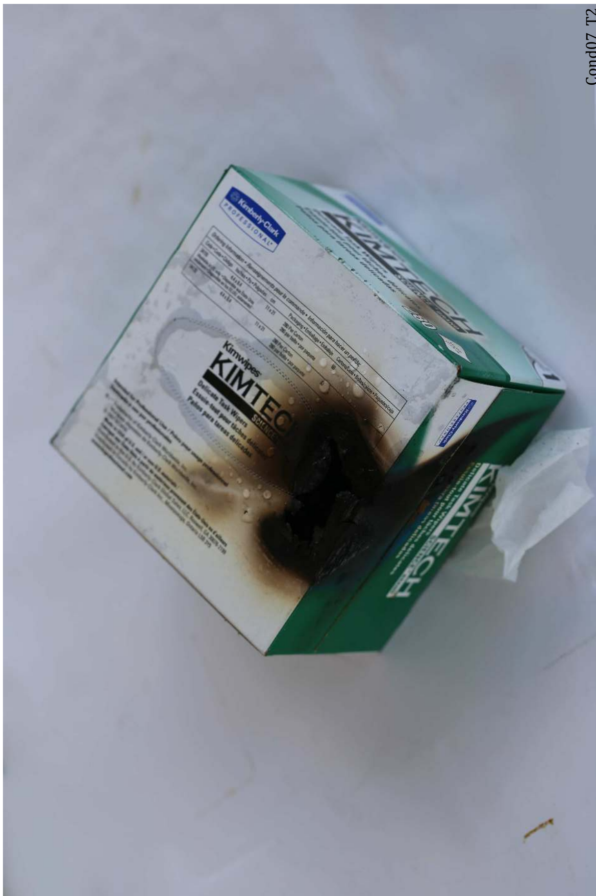
Figure 152: Condition 07 Trial 2. The box of task wipes was singed.
