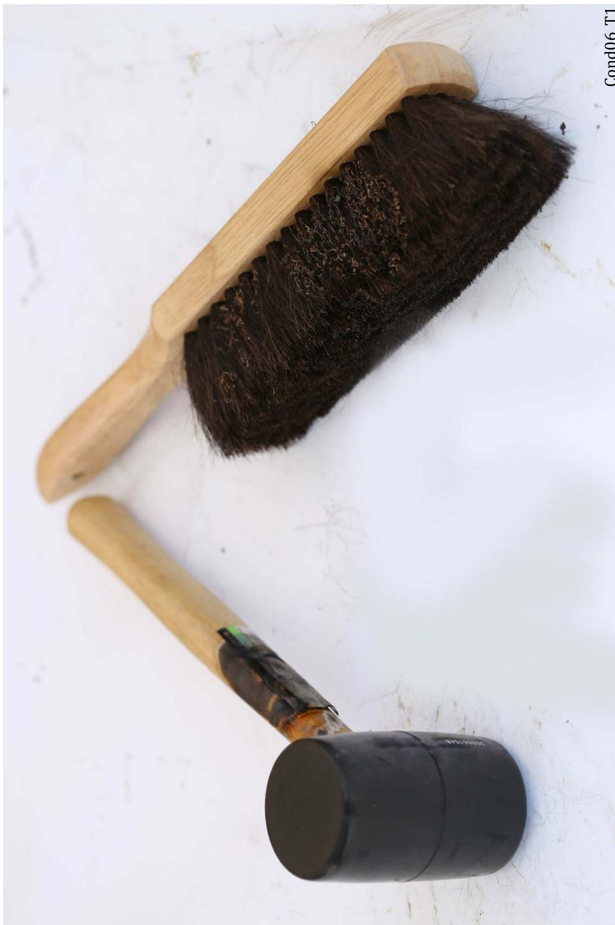
Figure 143: Condition 06 Trial 1. The horsehair brush and mallet were lightly singed.
