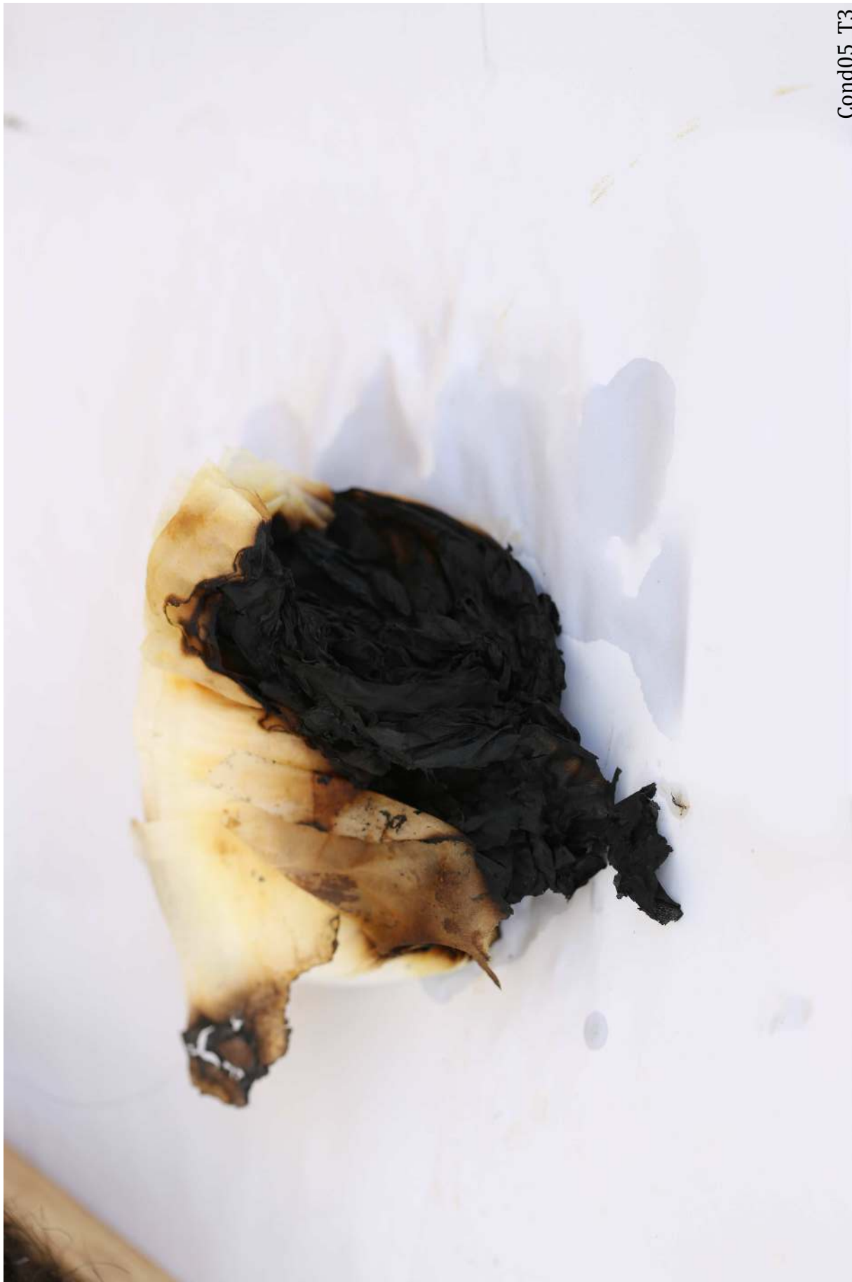
Figure 139: Condition 05 Trial 3. Task wipes were burned.
