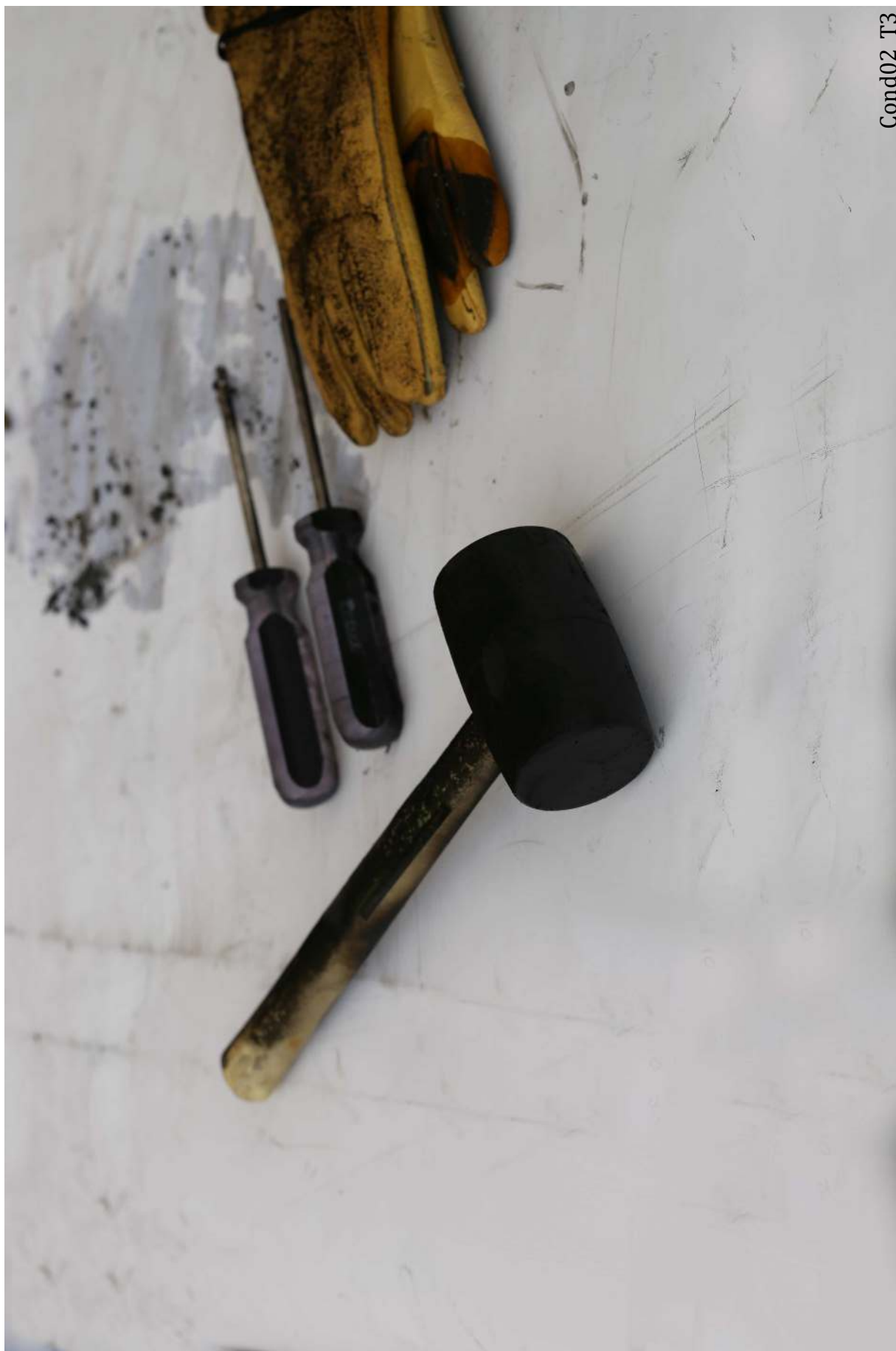
Figure 90: Condition 02 Trial 3. Not all consumables present engaged in the fire. Some charring is visible on the mallet, screwdrivers, and leather gloves.
