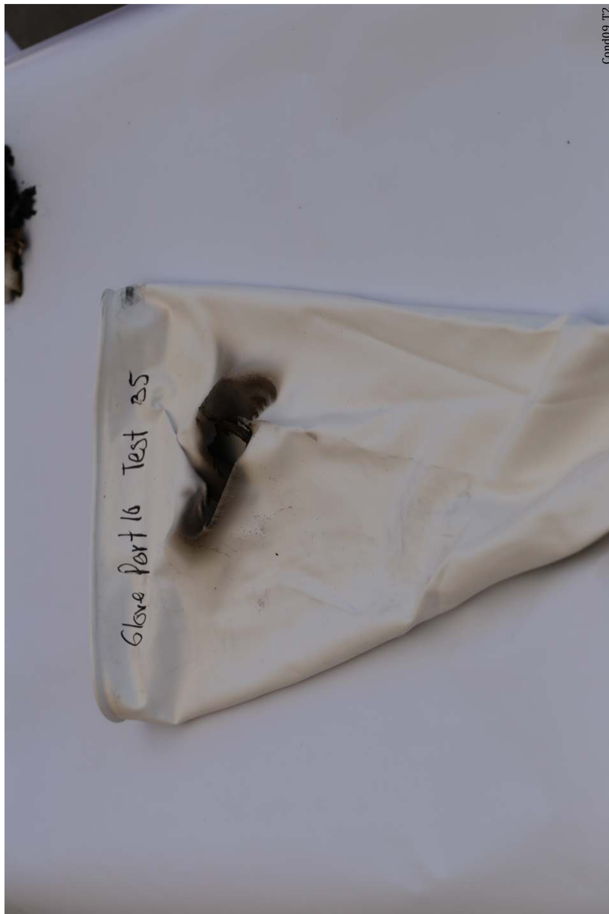
Figure 179: Condition 09 Trial 2. A small hole was burned in the port 10 glove near the ring.
