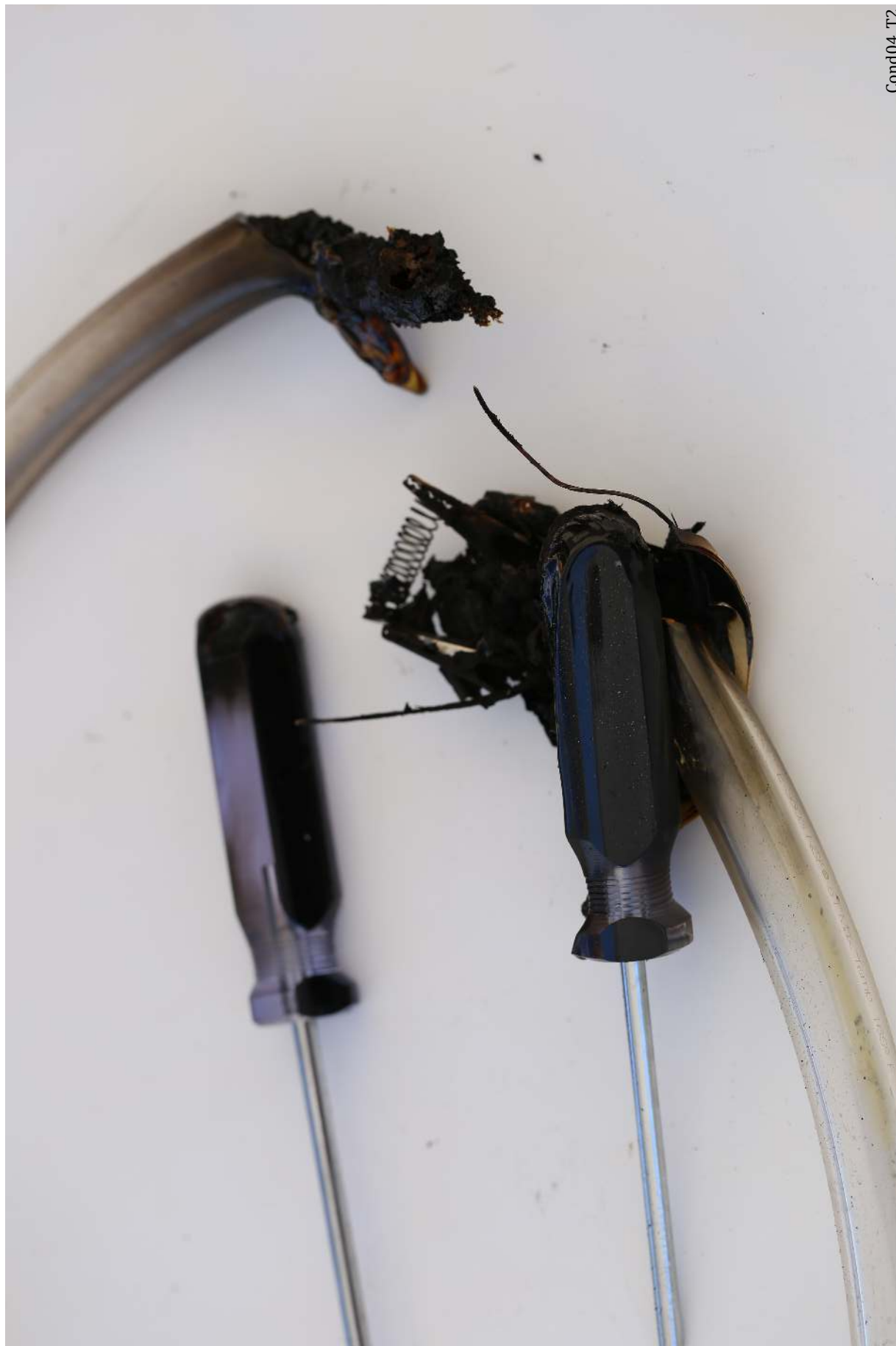
Figure 122: Condition 04 Trial 2. Tygon tubing burned but the flame did not travel along the tubing.
