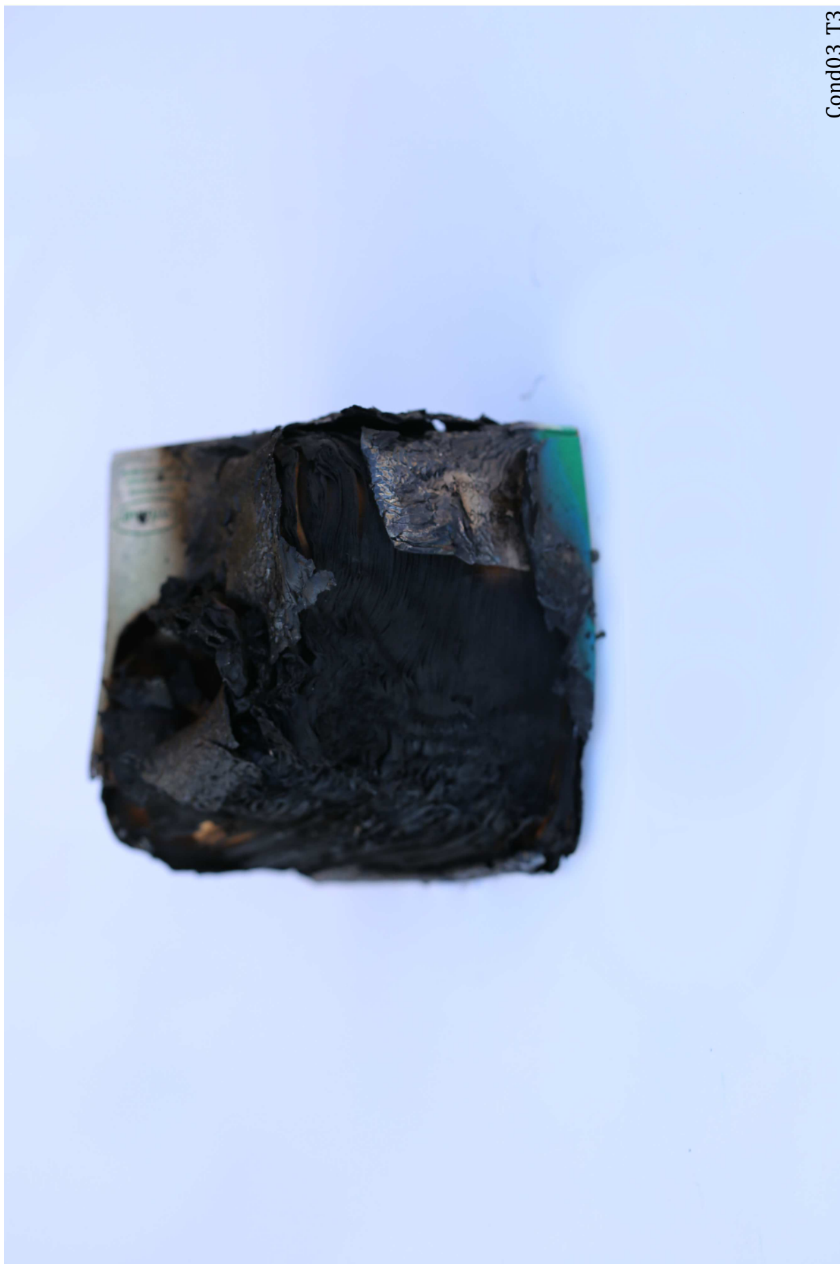
Figure 110: Condition 03 Trial 3. The box of task wipes burned thoroughly.
