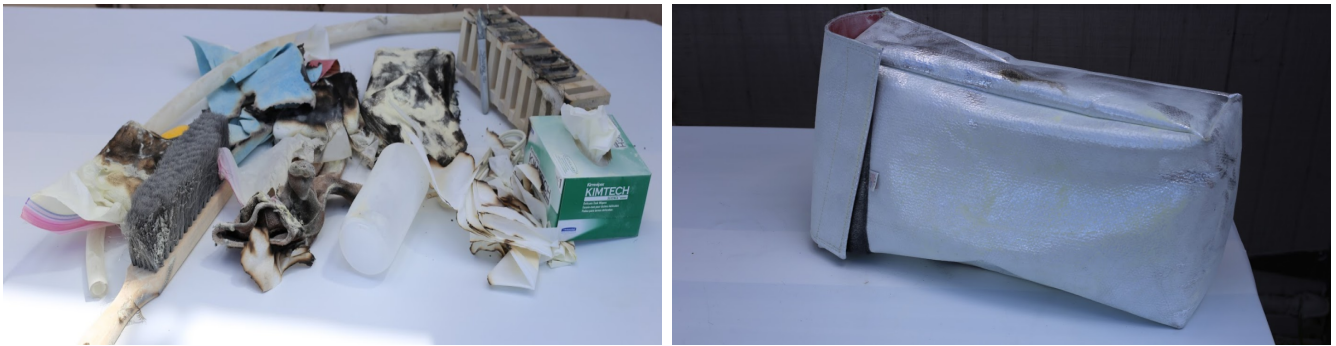
Figure 21: Additional views of GB consumables located on the inlet side after testing ( Test 3 ). Some items were in the open (left) and some alcohol-soaked cheesecloth was stored in a fire resistant bag (right, Hot-Stop 'L' , large item pouch, Baker Aviation, Addison, TX).
