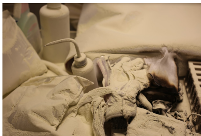
Figure 24: Post-testing images of consumables placed on the inlet side of the GB from Test 4 , the third of three test fires. The shown items were located (red dashed line) atop a rack (black dashed line) inside the GB in the schematic above the photographs.
