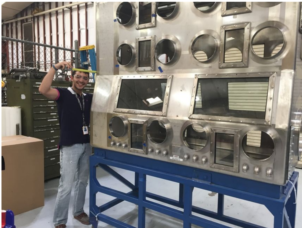
Figure 2. A steel LANL glove box used for experimentation is shown mounted onto a supporting frame. The box contains rectangular windows mounted to the glove box with steel frames, as well as open circular ports at the bottom, middle and top of the box for the
