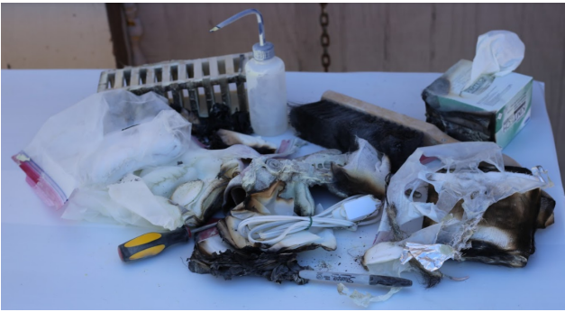
Figure 25: Additional views of GB consumables located on the inlet side after testing ( Test 4 ). Some items were in the open (left) and some alcohol-soaked cheesecloth was stored in a fire resistant bag (right, Hot-Stop 'L' , large item pouch, Baker Aviation, Addison, TX)).
