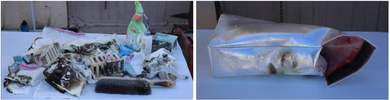
Figure 17: Additional views of GB consumables located on the inlet side after testing ( Test 2 ). Some items were in the open (left) and some alcohol-soaked cheesecloth was stored in a fire resistant bag (right, Hot-Stop 'L' , large item pouch, Baker Aviation, Addison, TX)).
