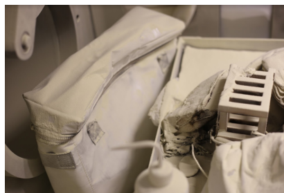
Figure 26: Post-testing images of consumables placed on the exhaust side of the GB from Test 4 , the third of three test fires. The shown items were located (red dashed line) atop a rack (black dashed line) inside the GB in the schematic above the photographs. Also shown is the dry chemical deposition in the Attached Volume (right).
