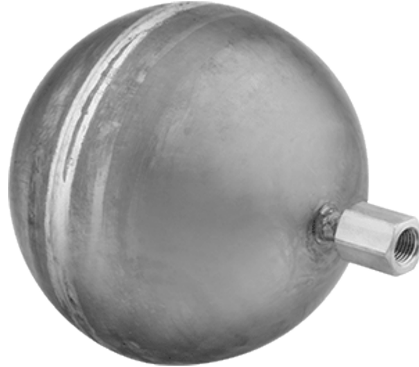
304 Stainless Steel Threaded Float, 2" Diameter, 1/4"-20 UNC Thread Size, 750 Maximum PSI
