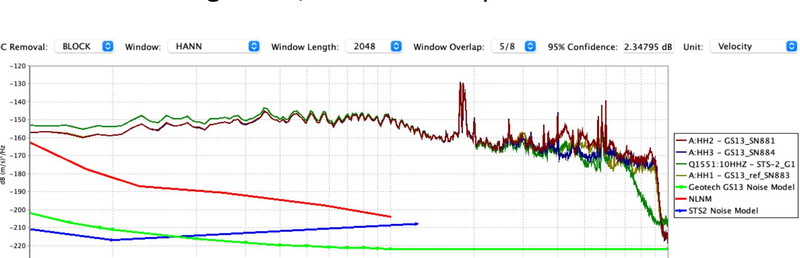
PSD of the August 20, M=3.0 earthquake @ 29.5 C
