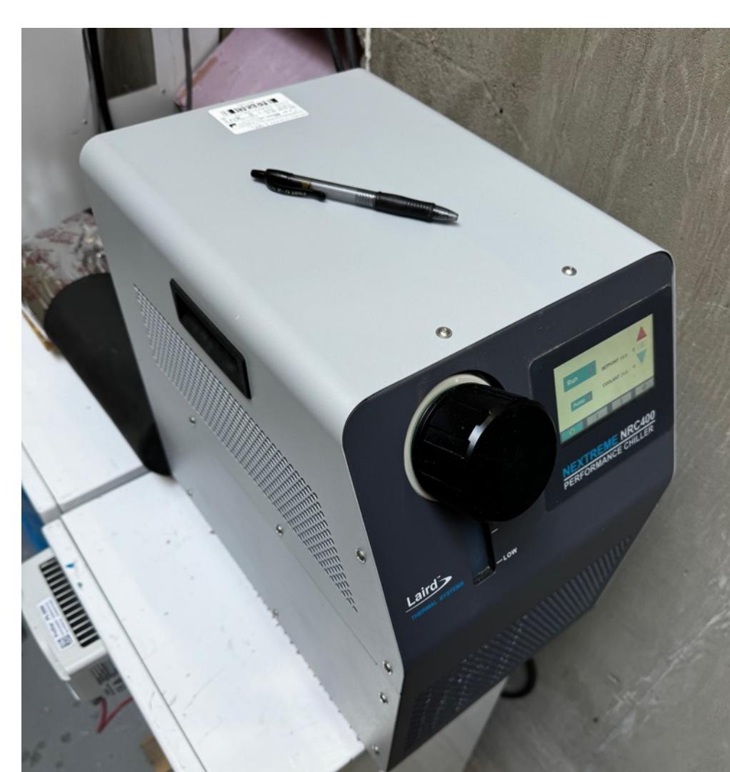
The Laird Thermal NRC-400 (left) is a PID-thermostatically controlled heater/chiller unit. There is no refrigerant compressor as the unit relies upon the Peltier effect for heat transfer. The unit is capable of adding or extracting up to 400 W of heat and, under steady state conditions, can maintain set temperature to within 0.05 C.
