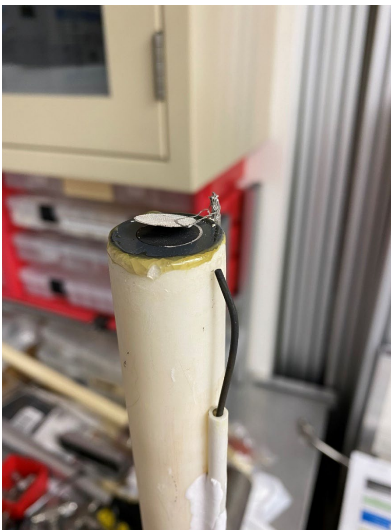
Figure 4. Six-layer GDC cell after testing. The entire cathode was detached.
