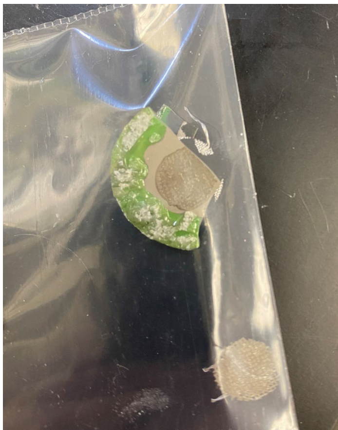
Figure 6. Four-layer cell after disassembly. Note how the glass seal on the anode side defines where the anode has been reduced from NiO (green color) to nickel metal (gray color).
