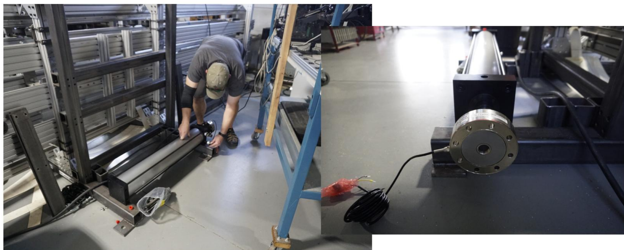
Figure 25 - Preparation of PTO frame and test actuator
