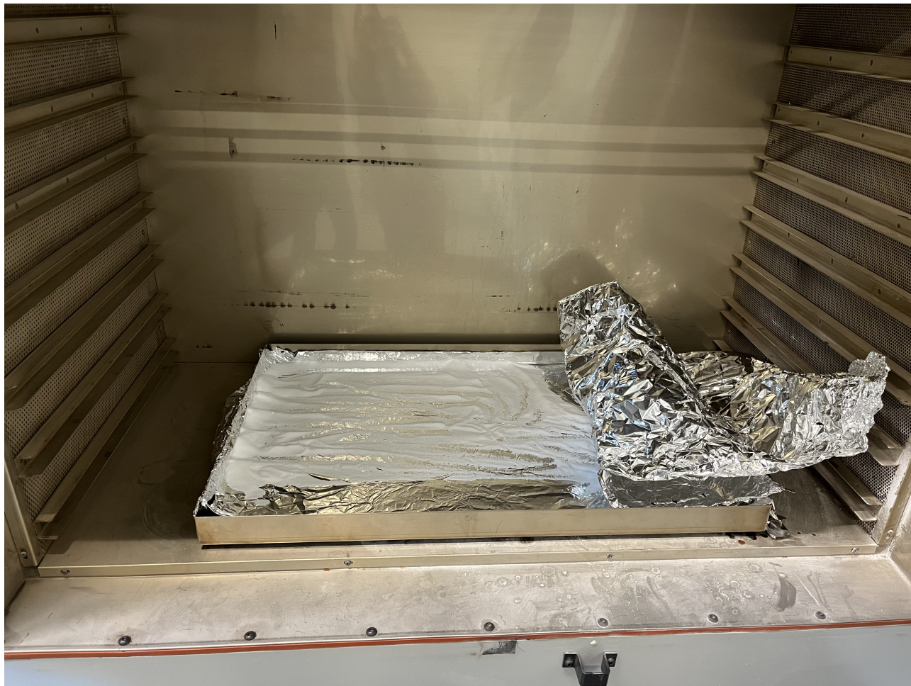
Figure 13: A picture of the oven process to back the salt before filling.
