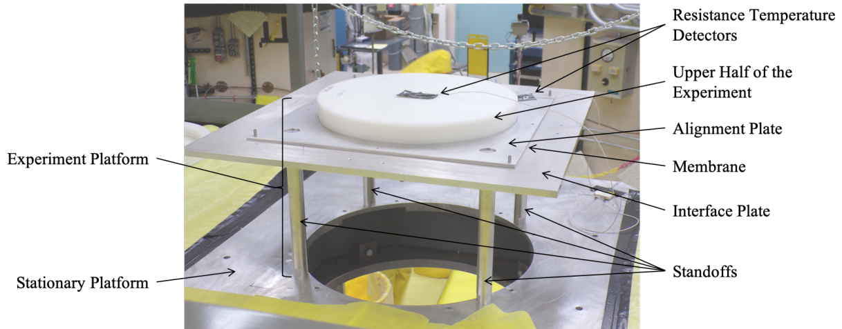
Figure 5: Upper stationary platform of the Comet, with the experiment platform. During the benchmark measurements, the resistance temperature detectors and alignment plate were removed.
