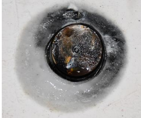
Figure 19. Failed gauge due to side wall heating.
