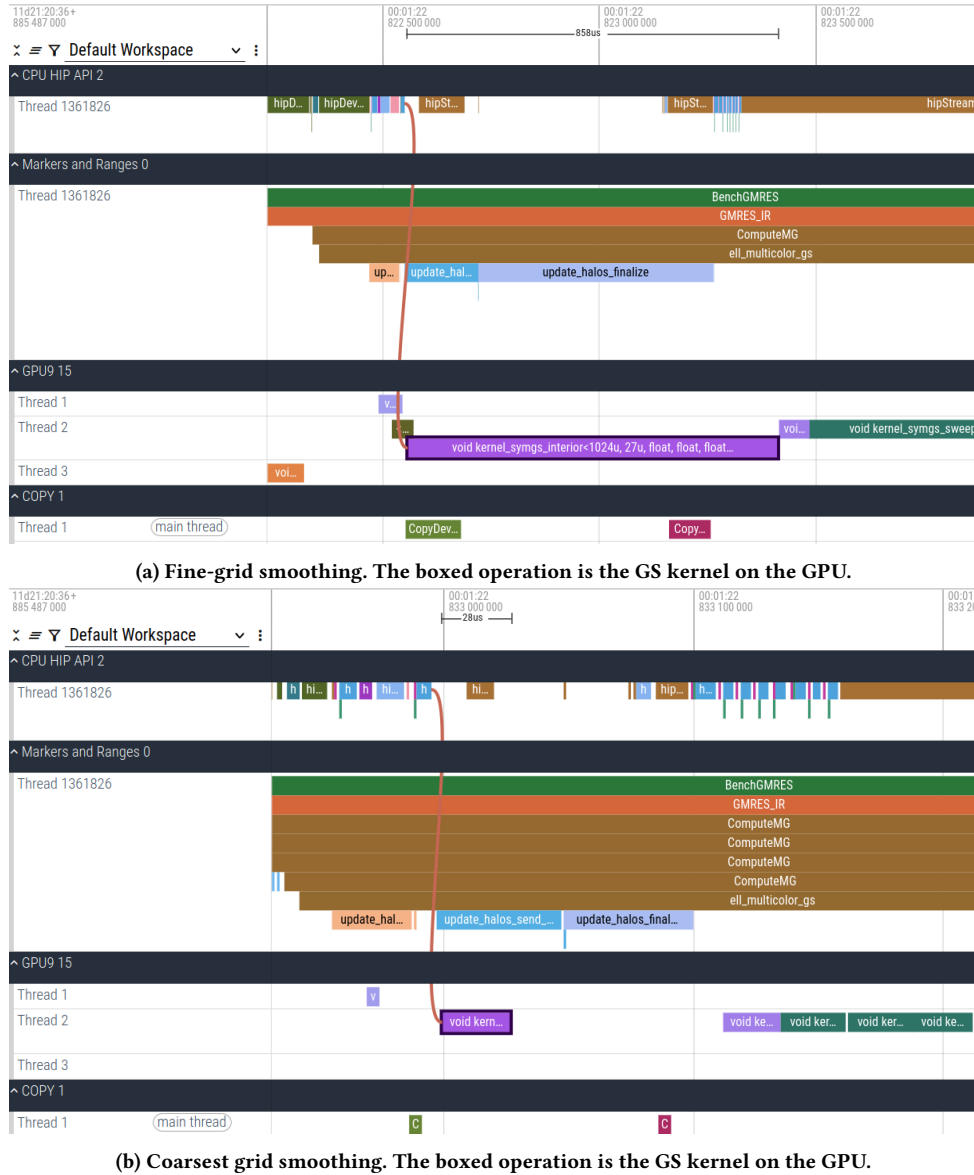
Figure 9: Traces of our GMRES-IR implementation in an 8-node benchmark run on Frontier. In each trace, there are 4 sections from top to bottom: ‘CPU HIP API’, ‘Markers and Ranges’, ‘GPU’ and ‘COPY’. Purple bars in the ‘GPU’ section represent the interior Gauss-Seidel kernel. The consecutive orange, blue and gray-blue bars in the ‘Markers and Ranges’ section represent halo buffer and communications operations. In the ‘COPY’ section, the green bar represents the device-to-host copy of the send buffer, while the red bar after it is the host-to-device copy of the received data.
