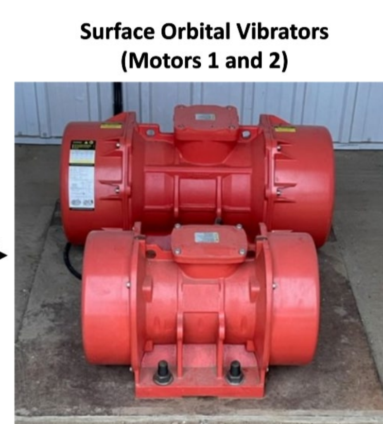
Diagram showing a cross section of the SOV setup and the location of the 3C reference geophone. Right: SOVs. Motors 1 and 2 are induction motors that spin eccentric weights to generate vertical compressive and horizontal shear forces.
