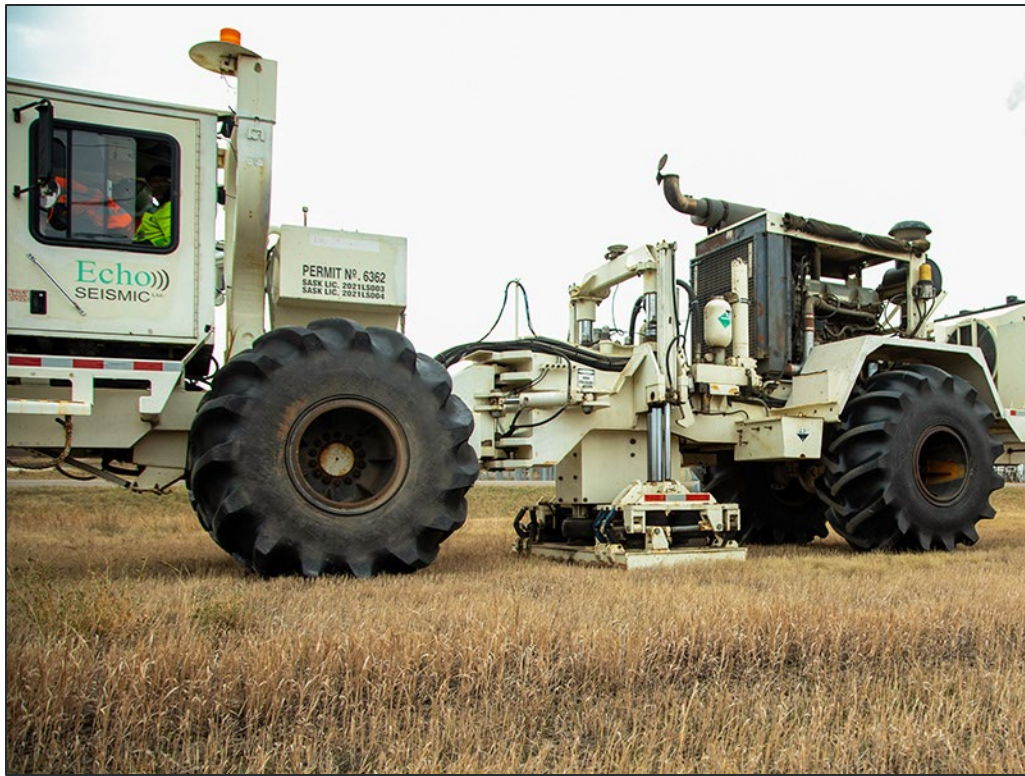
Vibroseis truck used to acquire DGC's commercial 2D survey.
