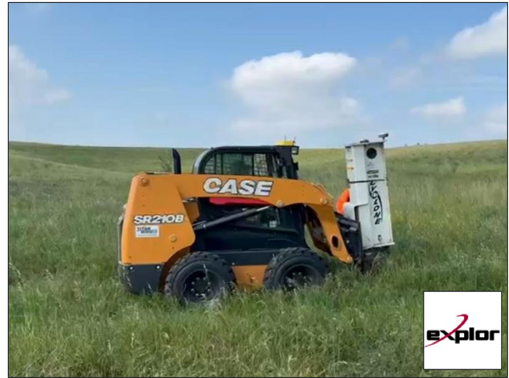
Accelerated weight drop (AWD) used in this project.
