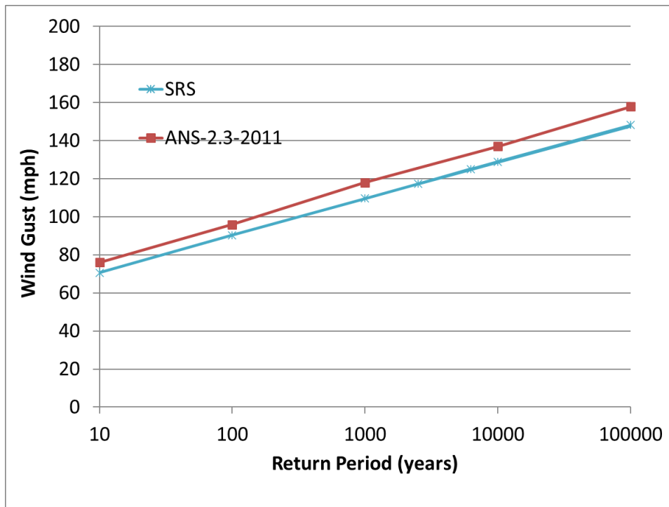
Figure 4.6 Projected wind gust values for various return periods at SRS (from Eq. 21), along with the values from the ANS-2.3-2011 reports.
