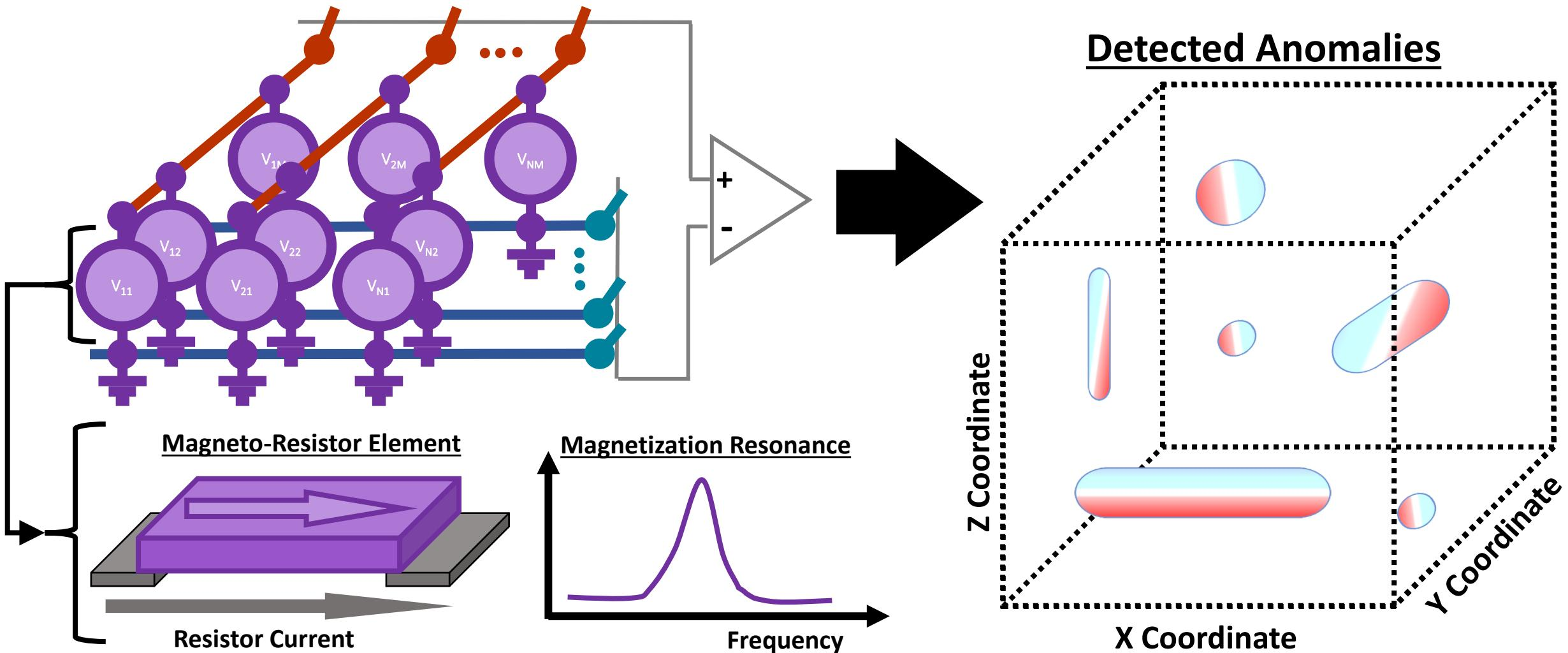
*We propose a novel sensor leveraging nonlinear magnetization dynamics for 3D imaging of small ( $\sim 1 \mu\text{m}$ ) defects through magnetic field gradients.*
