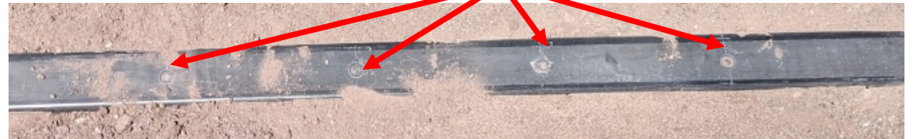
Pressure transducers spaced apart by 1 ft
