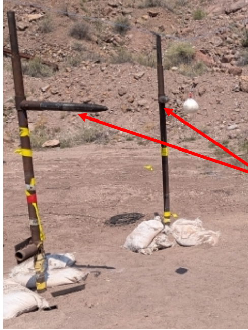
Free-air pressure transducers in line with the charge
