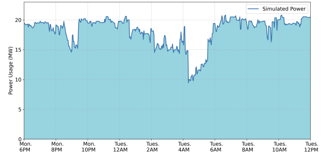
Figure 7: The results of simulating a synthetic job trace running on Frontier with the FastSim scheduler. The simulated job schedule is passed to ExaDigiT, which can then compute the resource usage over time.
