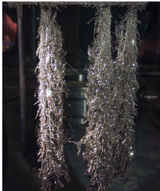
Figure 3.1-4 Image from Argonne National Laboratory experimental results of Uranium plated onto an electrode
