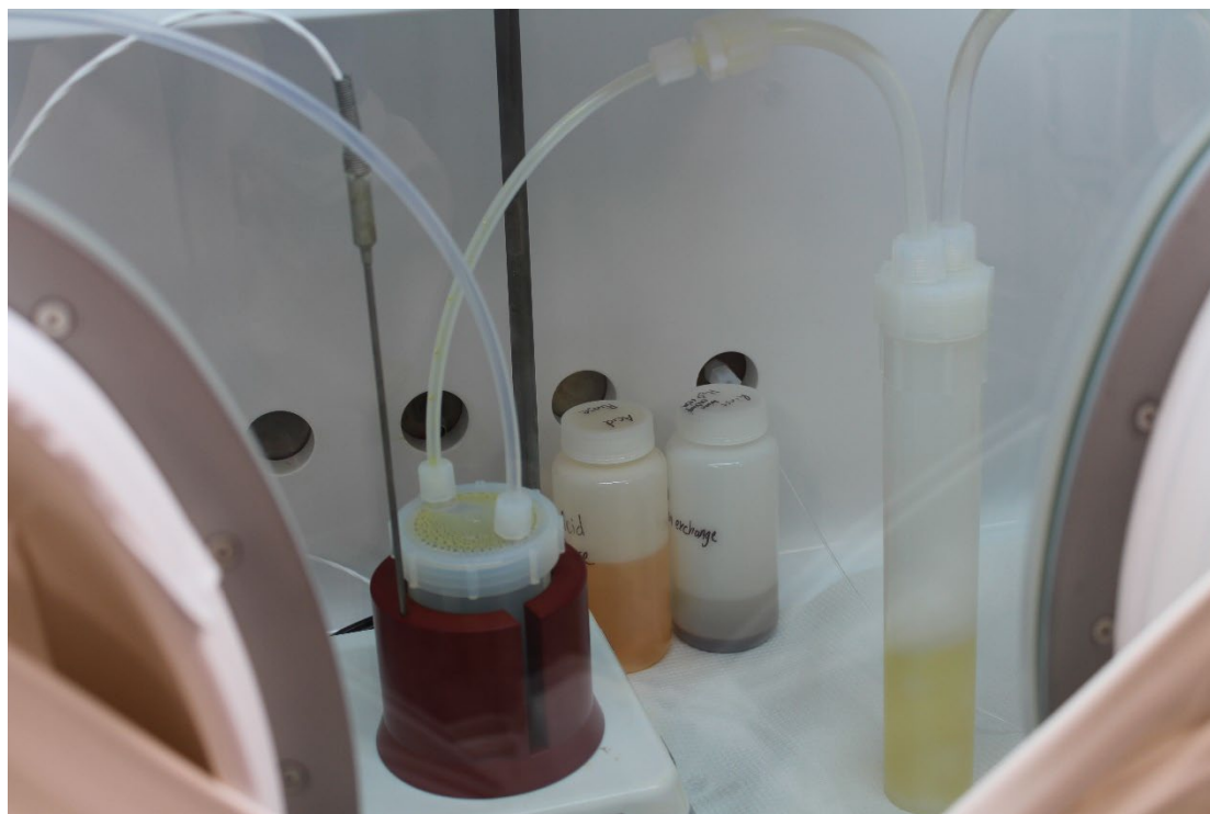
Figure 14. Evaporation of HCl/HI solution through Teflon impingers for conversion of eluted Pu to nitrate form in nitric acid.
