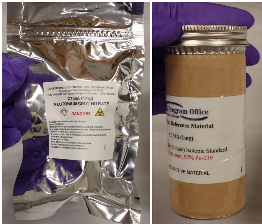
Figure 24. Unit 1 of C138A packaged in Mylar zip-lock pouch (left) and in cardboard mailer tube (right).
