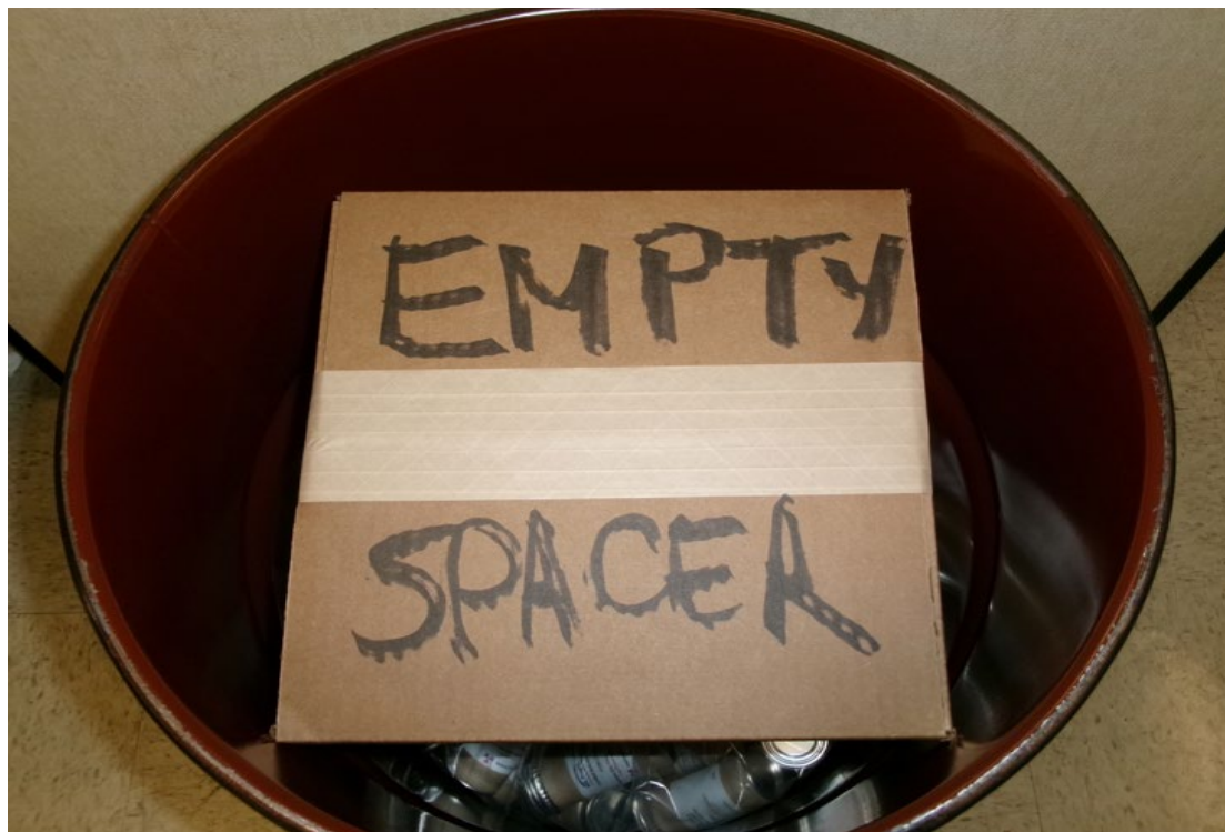
Figure 28. Example drum with empty spacer box on top of packaged units to reduce movement during shipping.
