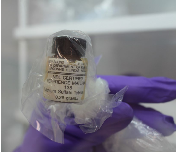
Figure 6. C138 unit in primary packaging from LANL.
