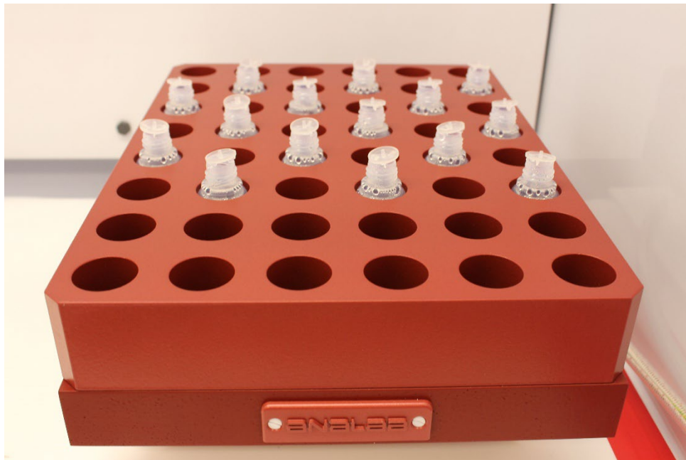
Figure 17. 15 CRM137A units gently evaporating on an Analab® hot plate with heating block, set to 85° C.
