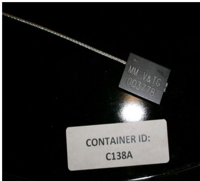
Figure 32. C138A container label and MM V&TG cable seal.
