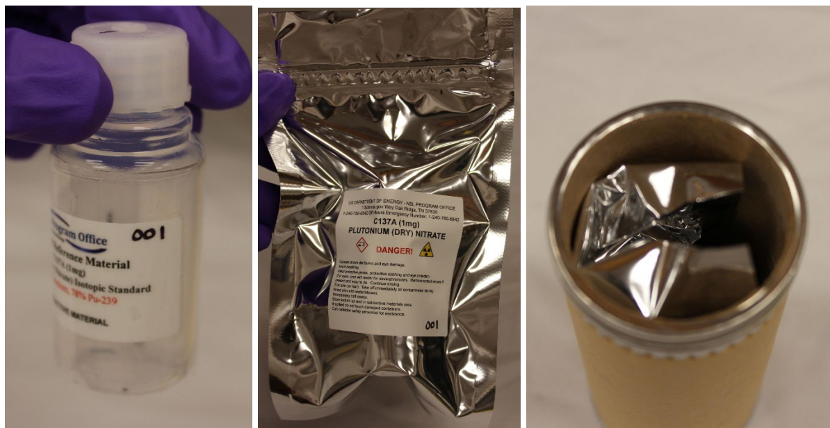
Figure 19. Unit 1 of C137A with label applied to bottle (left), inside labeled zip-lock mylar pouch (middle), and pouch placed inside cardboard mailer tube (right).
