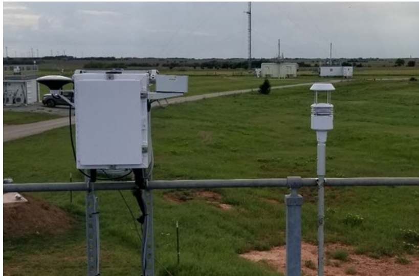
Figure 1. Infrared cloud imager with its integrated weather sensor deployed on SGP's guest instrument platform.
