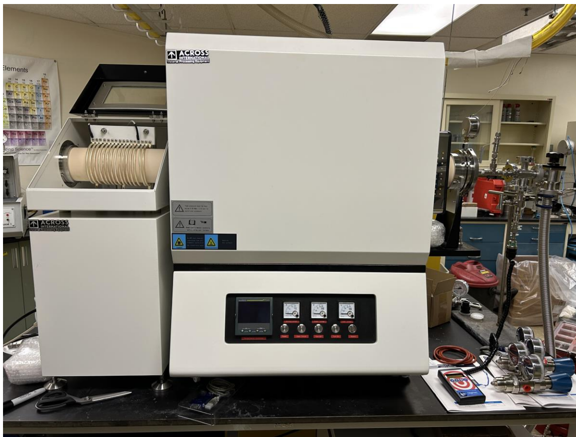
Figure 6. Commercial plasma enhanced MOCVD system procured during this funding period, with the induction coil shown on the left. Temperature control is shown on the furnace body, and not-pictured is the gas-mixing module, vacuum system, and AC power controller for the plasma generation system.
